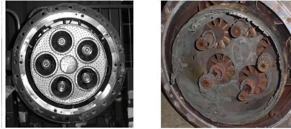
Figure 2.2: A new Burner assembly (left) and a burner assembly damaged by combustion instability (right) [65]
