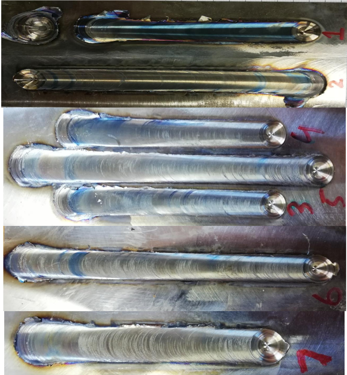
Figure 4 UNS S32750 SDSS FSPed plates.
