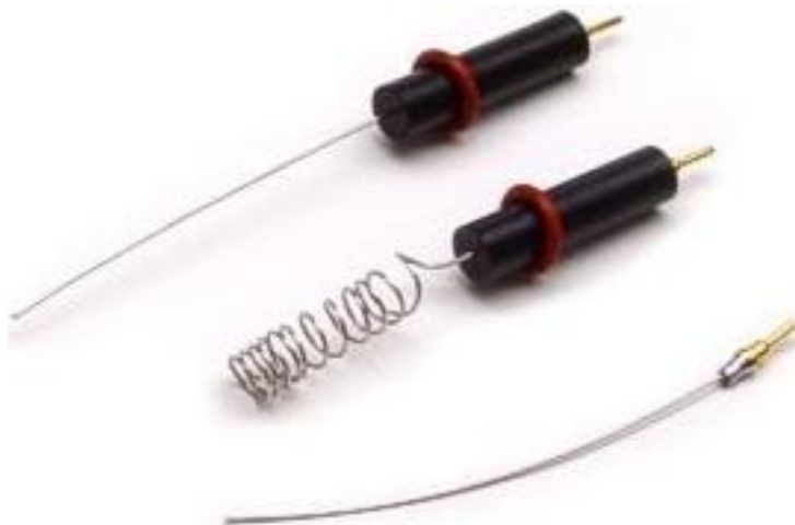
Figure 7 Picture of the counter electrode (platinum wire) [174]
