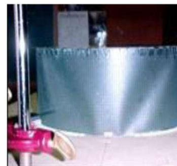
c) Buckling of a tank due foundation settlement
