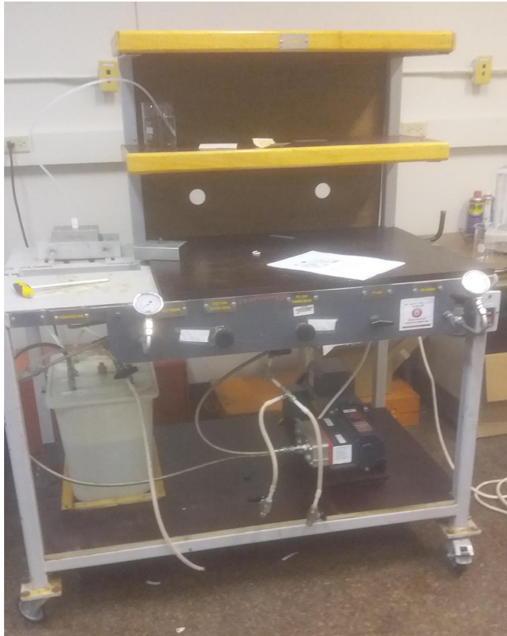
Figure 13. The laboratory filtration setup for cross-flow membrane filtration
