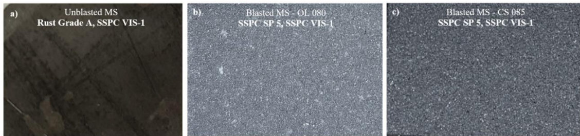
Figure 4.1 a) Appearance of non-textured mild steel substrate b) Appearance of substrate textured using Olivine (OL 080) abrasive with SSPC SP 5 finish c) Appearance of substrate textured using Calcium Silicate (CS 085 abrasive) with SSPC SP 5 finish
