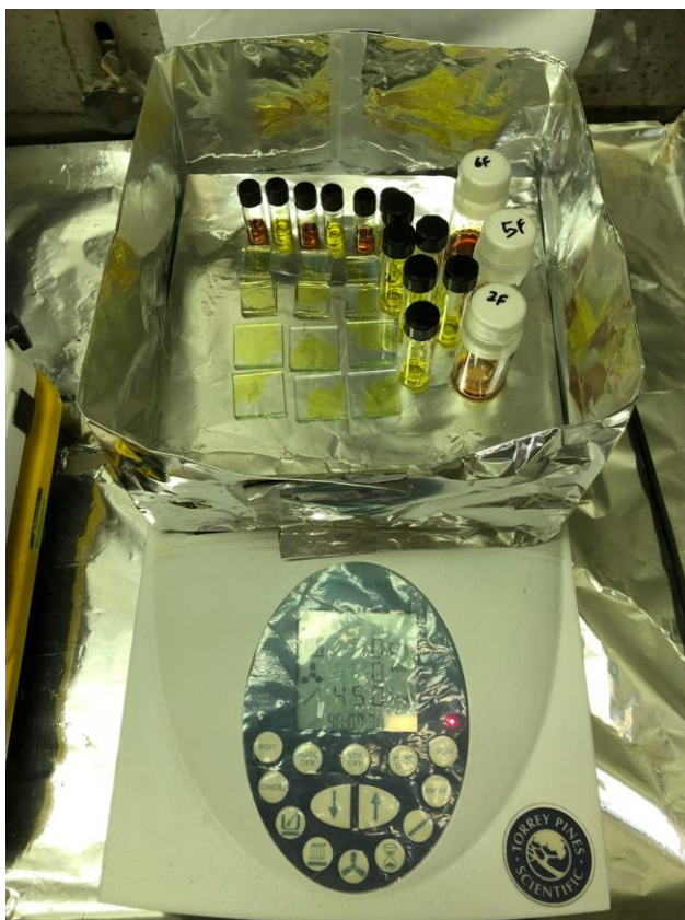
Figure 8 Growth of bulk and thin perovskite single crystals using programmable hotplate.
