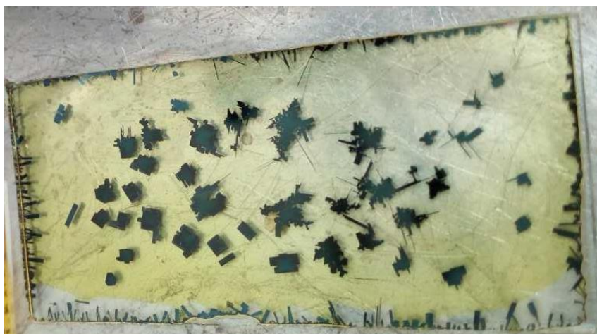
Figure 93 The 2D/3D BAI: MAPbI 3 perovskite thin single crystal between two ITO coated glasses.
