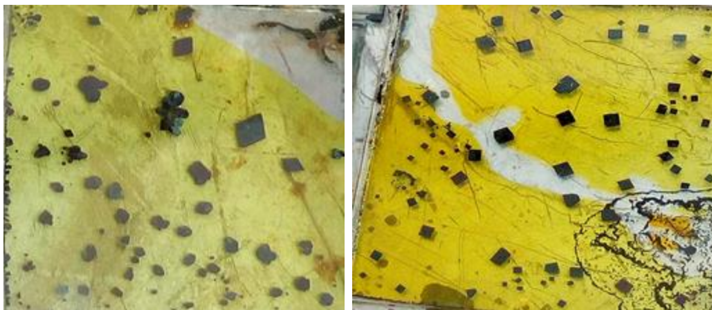
Figure 92 The 3D MAPbI 3 perovskite thin single crystal between two ITO coated glasses.
