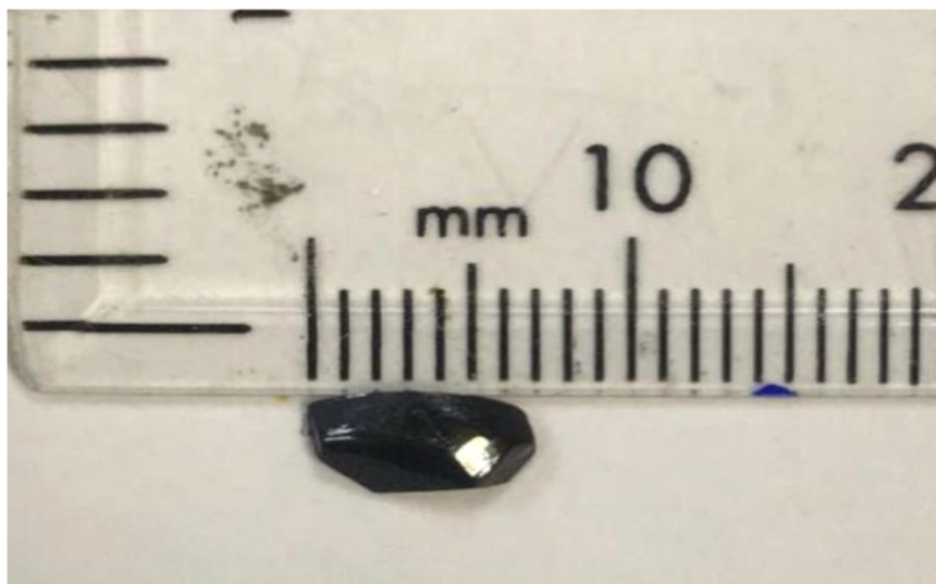
Figure 89 The 3D MAPbI 3 perovskite bulk single crystal.
