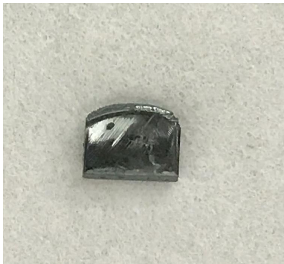
Figure 91 The 2D/3D PAI: MAPbI 3 perovskite bulk single crystal.
