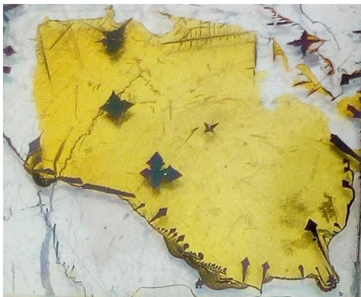
Figure 94 The 2D/3D PAI: MAPbI 3 perovskite thin single crystal between two ITO coated glasses.
