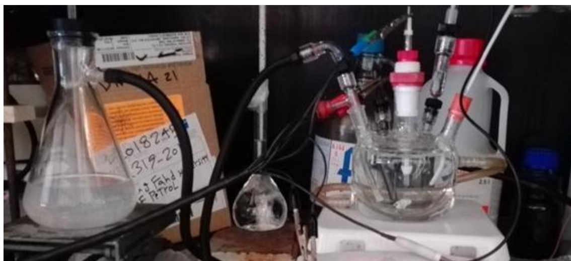
Figure 7.16 Experimental set-up for H_2S corrosion measurement
