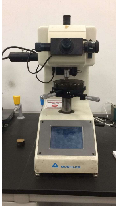
Figure 4.7 - Micro Hardness Tester supplied by Buehler instruments.
