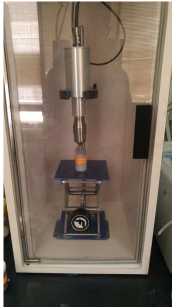
Figure 4.2 - Ultrasonic probe sonicator (Model VC750, Sonics)
