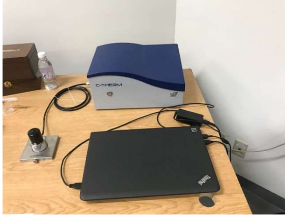
Figure 4.8 - C-Therm TCI Thermal Conductivity Analyzer.
