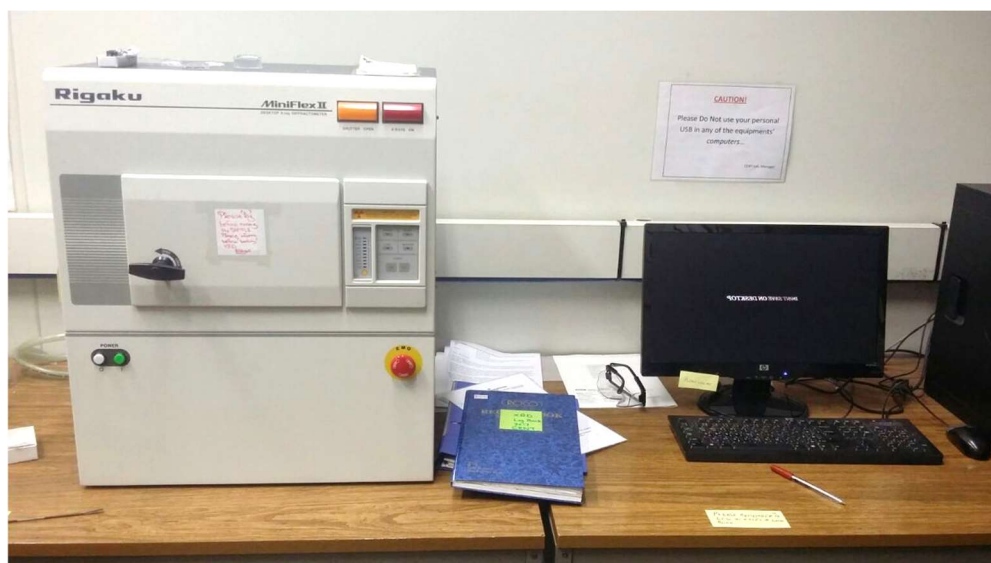
Figure 4.5 - Rigaku desktop x-ray diffractometer model “Miniflex II”.
