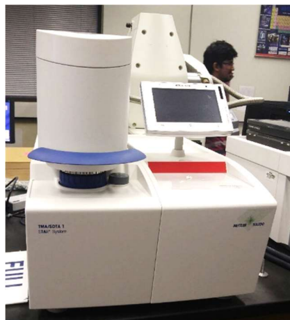
Figure 4.9 - Mettler Toledo Thermal mechanical analyzer (TMA/SDTA 1 LF/1100).
