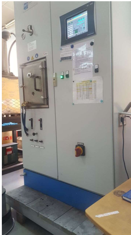
Figure 4.3 - Spark Plasma Sintering system from FCT, Germany.
