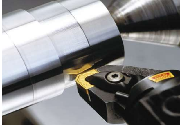
Figure 1.1 - A cutting tool insert under operation [3]
