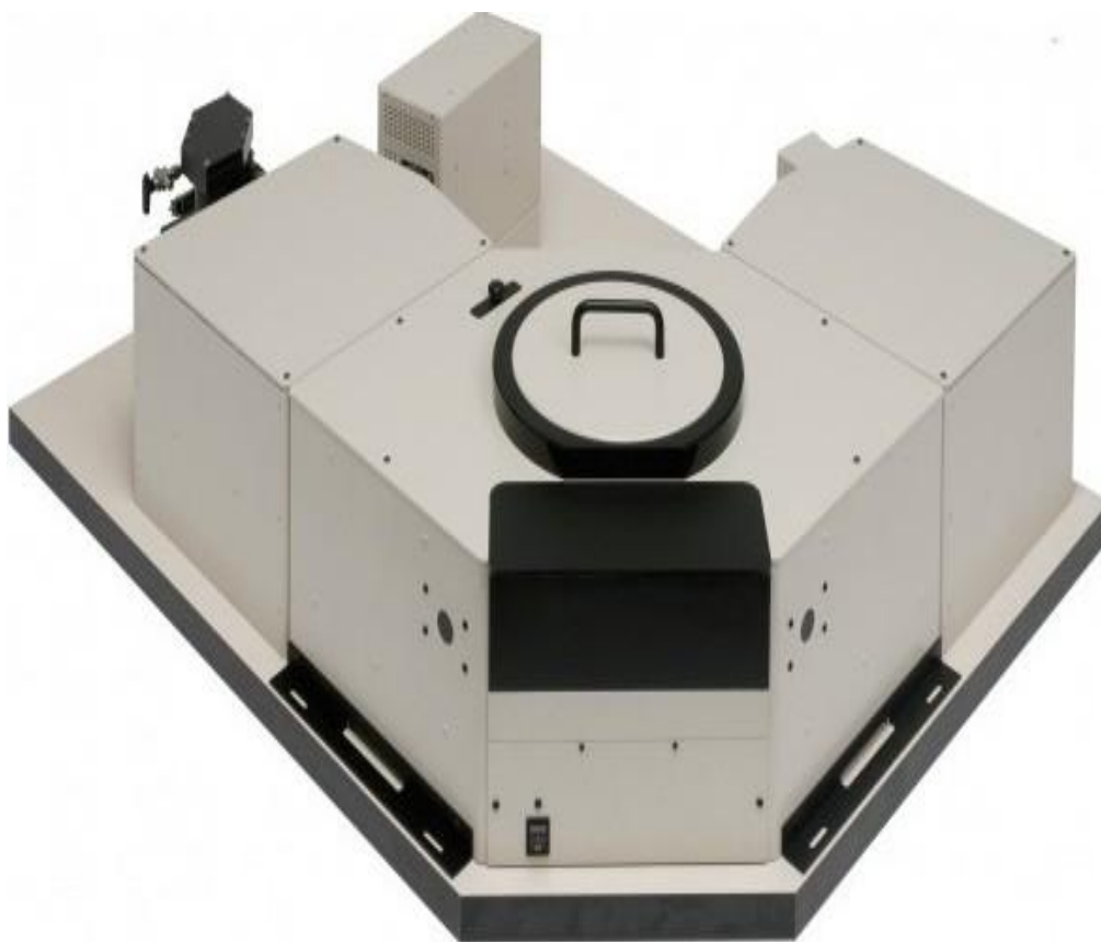
Figure 3.1: Picture of FLS 920 fluorescence spectrometer setup.
