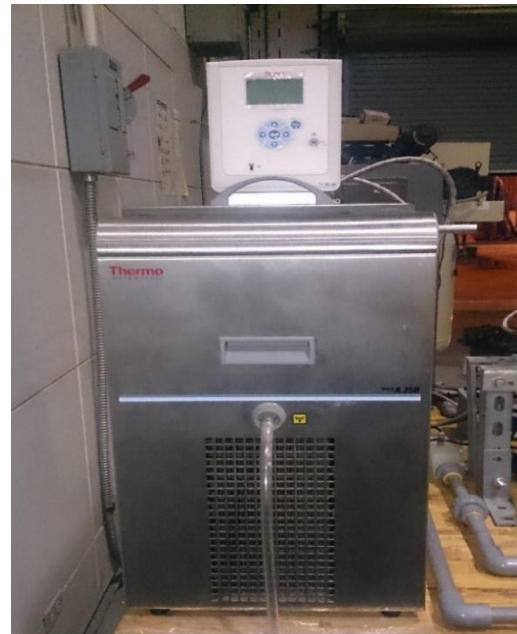
Figure 2.3: The electric chiller
