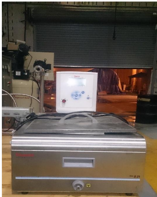
Figure 2.2: The electric heater
