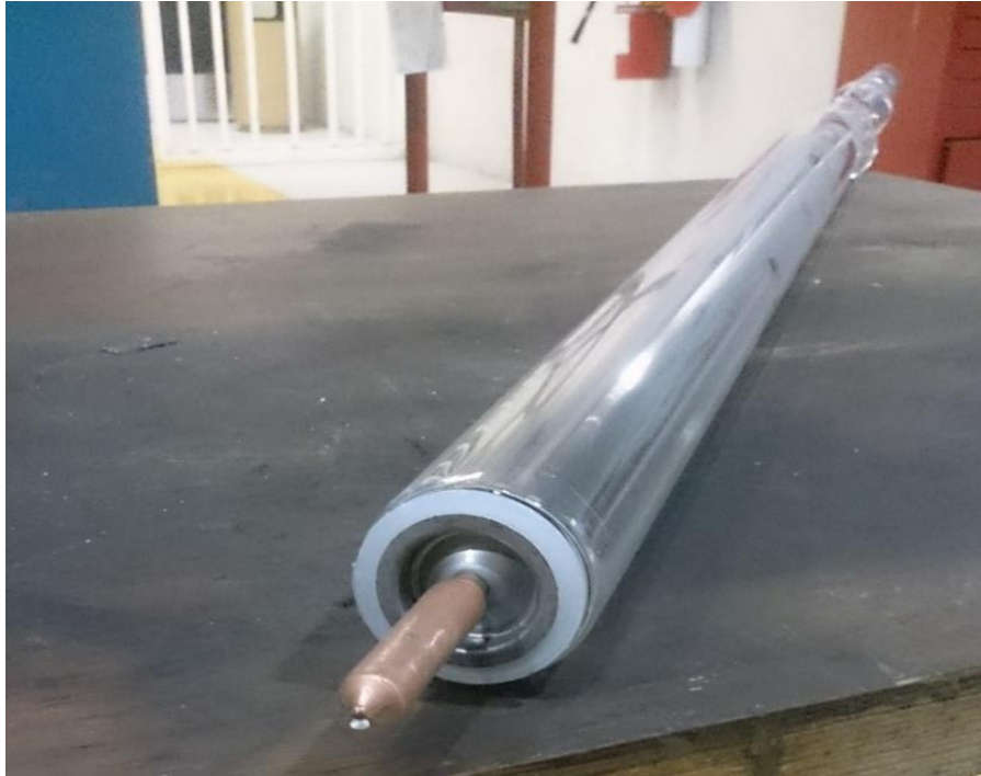
Figure 4.4: The Evacuated Tube Solar Collector
