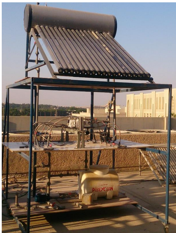
Figure 2.5: The evacuated tube solar collector
