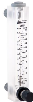
Figure 2.14: Feed flow meter
