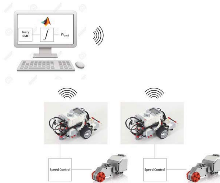
Figure 5.11: Using an integrator to change a fuzzy SMC command to a velocity command calculation and the inner loop diagram
