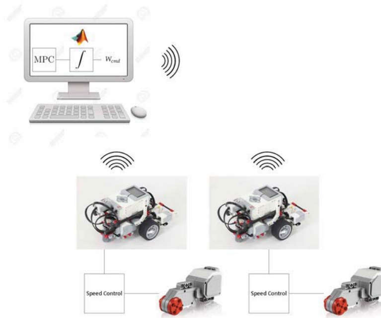
Figure 6.6: MPC velocity error is filtered using an integrator to get a velocity command that is sent to the robot inner loop diagram
