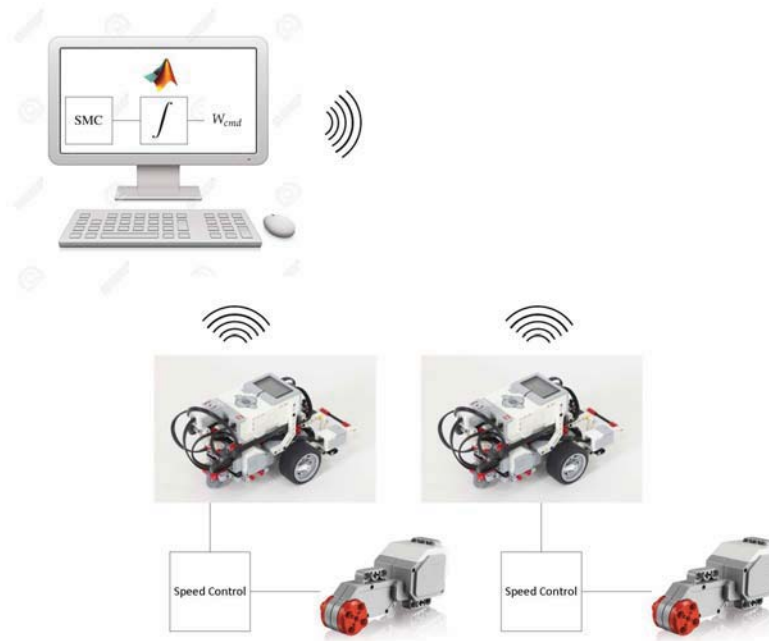
Figure 4.8: Using an integrator to change an SMC command to a velocity command calculation and the inner loop diagram
