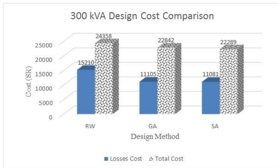
Figure 6. 1 Cost Comparison for 300 kVA Transformer
