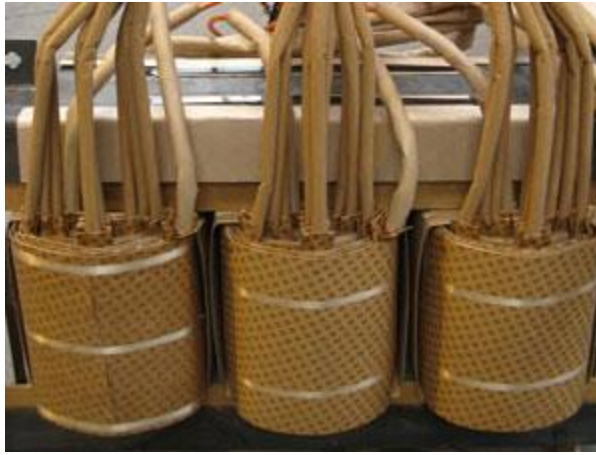
Figure 3. 6 DDP Winding Insulation
