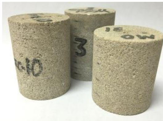
Figure 3-1 Indiana limestone core samples
