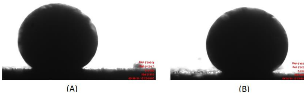
Figure 4-27 (A) Oil droplet in a bulk phase of seawater plus 1 wt% (PVP) plus 0.05 wt% nanoparticles at P=1500 psi and T= 60 C, (B) Oil droplet in a bulk phase of seawater plus 1 wt% (PVP) plus 0.05 wt% nanoparticles at P=3000 psi and T= 60 C
