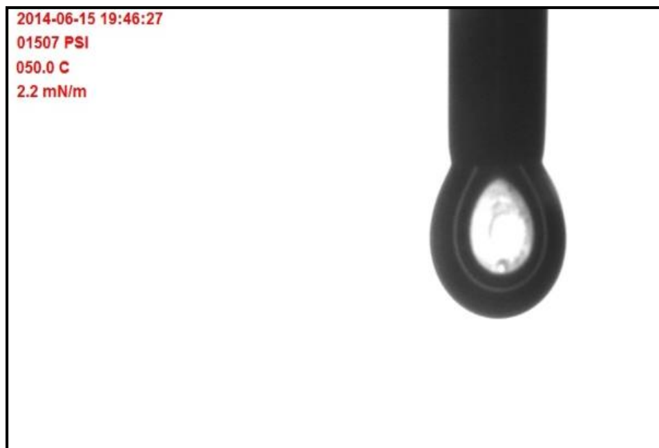
Figure B.3: Shape of 0.10 vol% fluorosurfactant FS-51 in CO 2 at 1500 psi and 50°C
