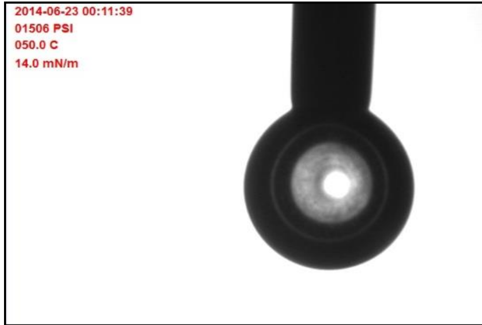
Figure B.1: Shape of distilled water drop in CO 2 (0% surfactant) at 1500 psi and 50°C
