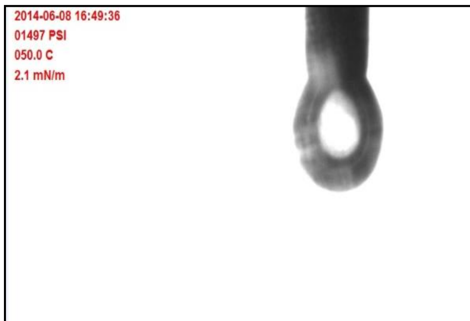
Figure B.4: Shape of 0.15 vol% fluorosurfactant FS-51 in CO 2 at 1500 psi and 50°C
