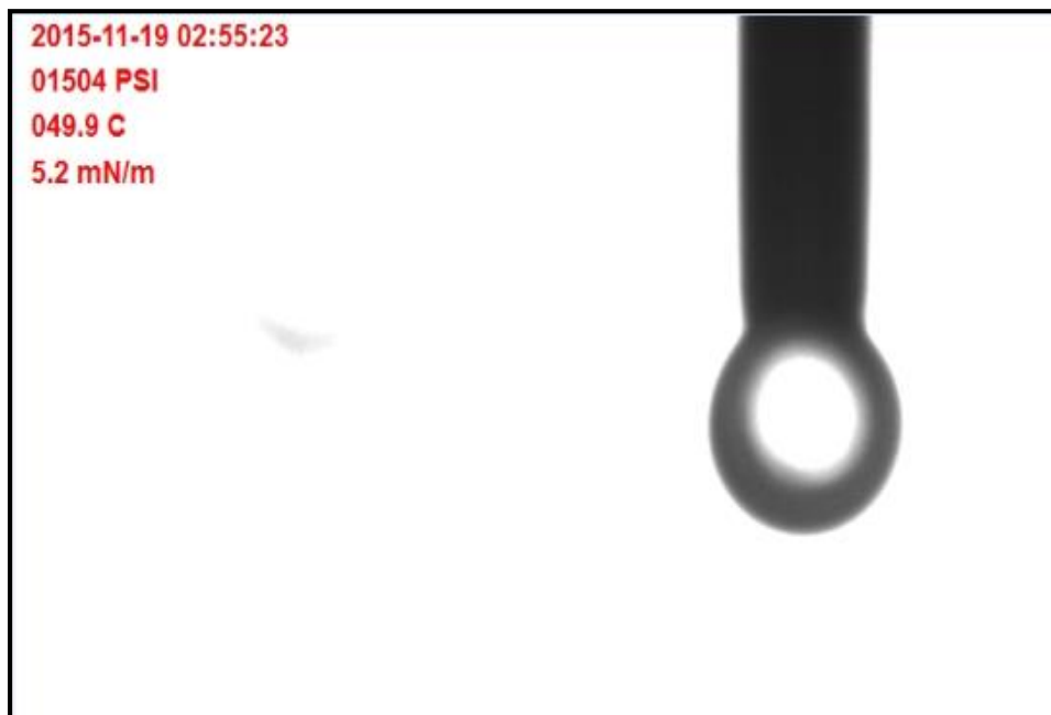
Figure B.10: Shape of 0.50 vol% AOS in CO 2 at 1500 psi and 50°C
