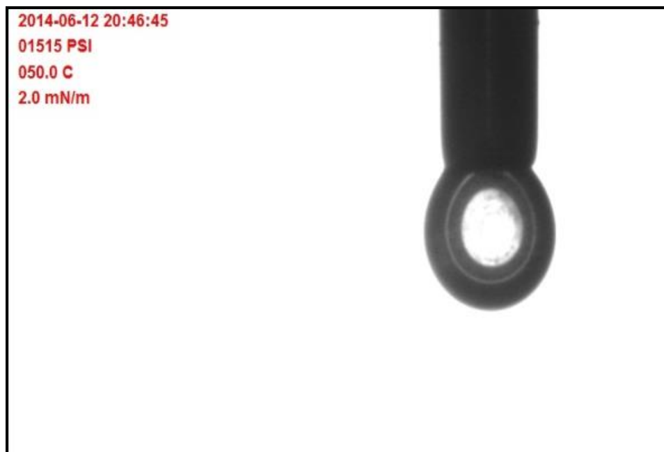
Figure B.5: Shape of 0.20 vol% fluorosurfactant FS-51 in CO 2 at 1500 psi and 50°C
