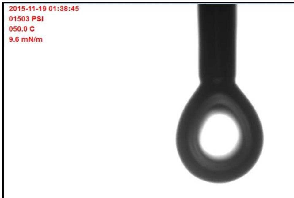
Figure B.8: Shape of 0.15 vol% AOS in CO 2 at 1500 psi and 50°C
