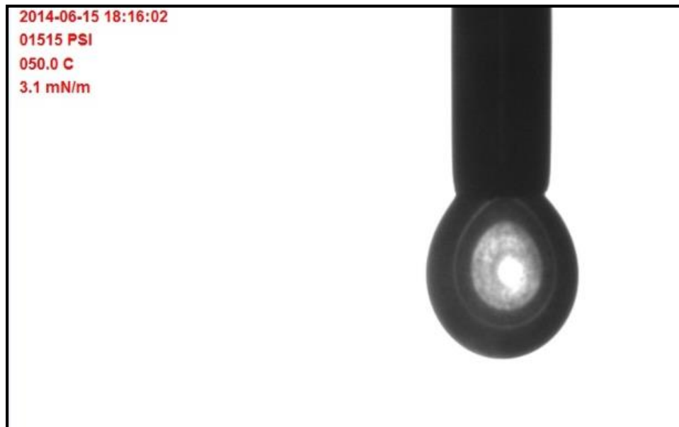
Figure B.2: Shape of 0.05 vol% fluorosurfactant FS-51 in CO 2 at 1500 psi and 50°C
