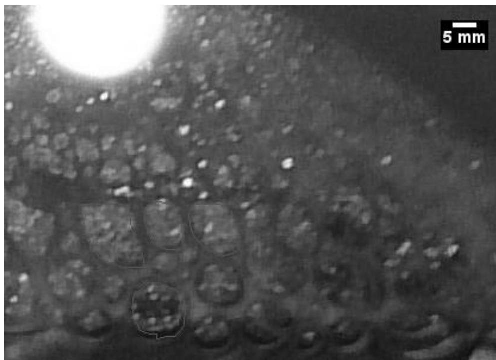
Figure B.50: 8-bit analyzed foam image using AOS surfactant for foam quality 0.90 and 10% N 2
