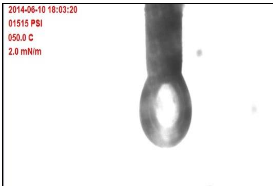
Figure B.6: Shape of 0.30 vol% fluorosurfactant FS-51 in CO 2 at 1500 psi and 50°C
