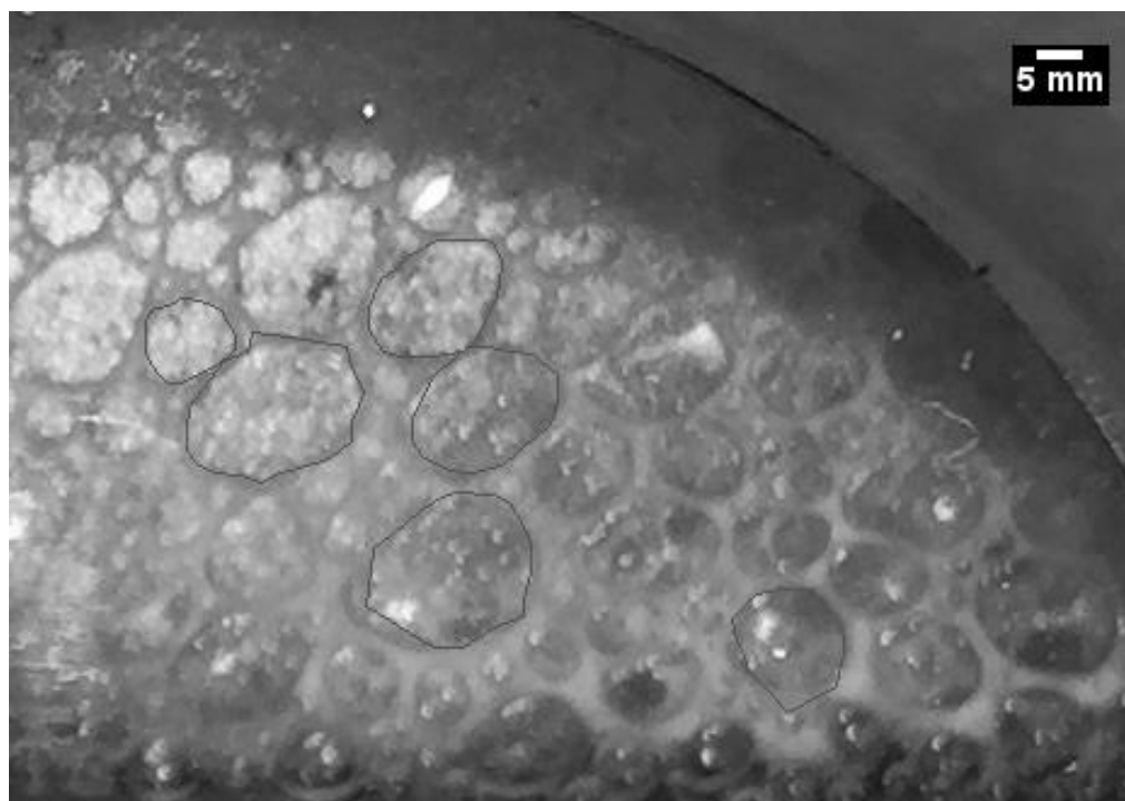
Figure B.51: 8-bit analyzed foam image using AOS surfactant for foam quality 0.90 and 15% N 2
