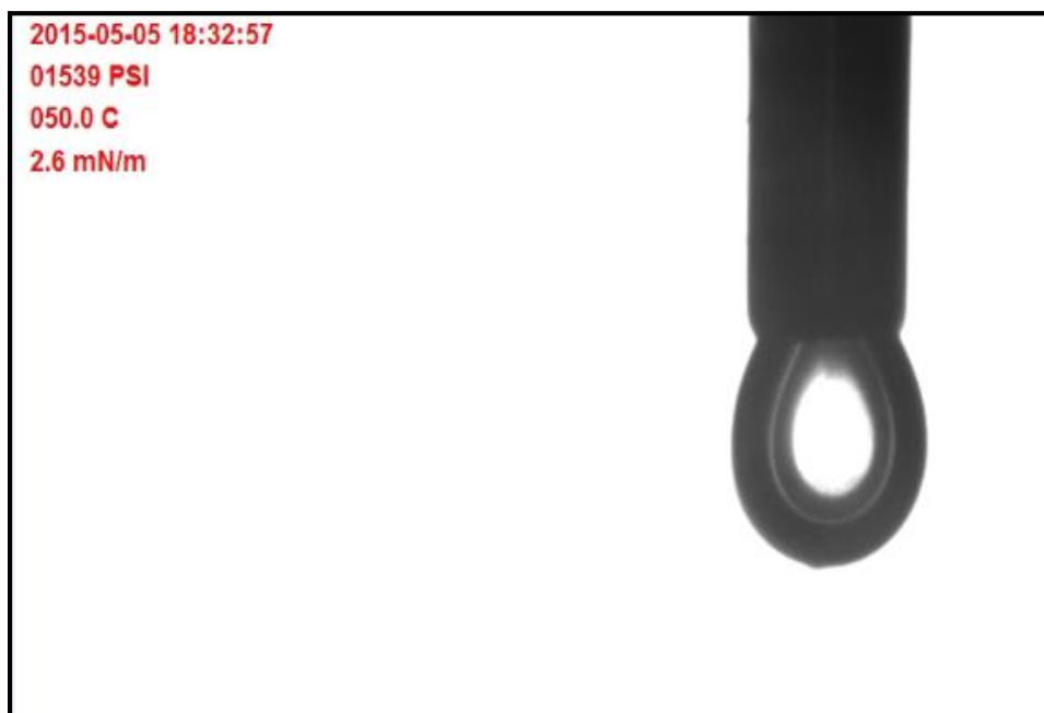
Figure B.16: Shape of 0.05 vol% witcolate in CO 2 at 1500 psi and 50°C
