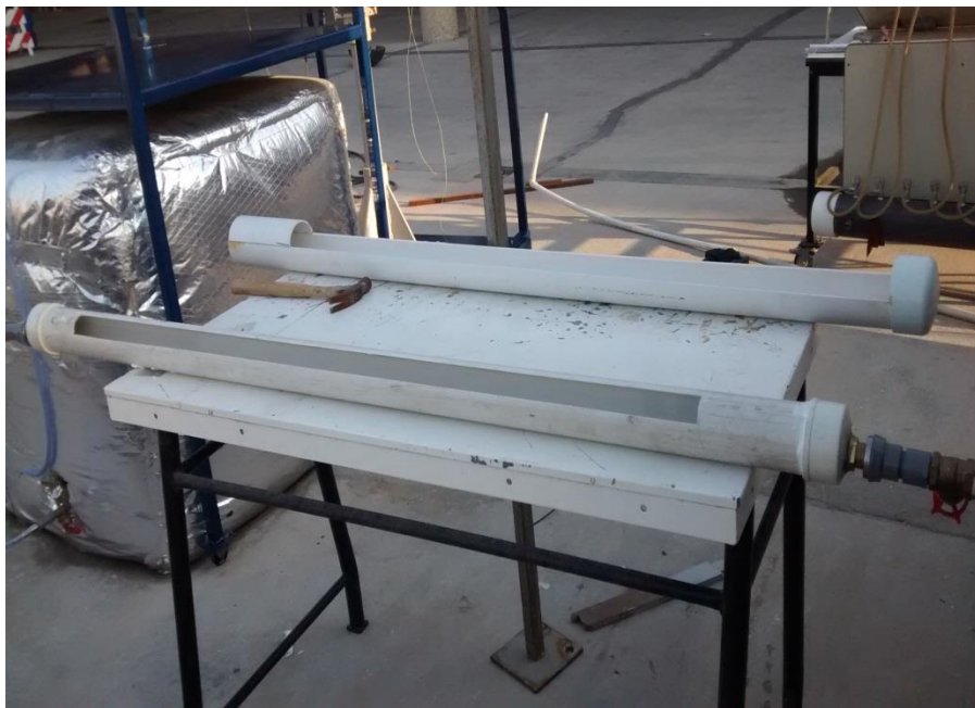
Figure 5-11 : Upper and bottom tube setup to collect water
