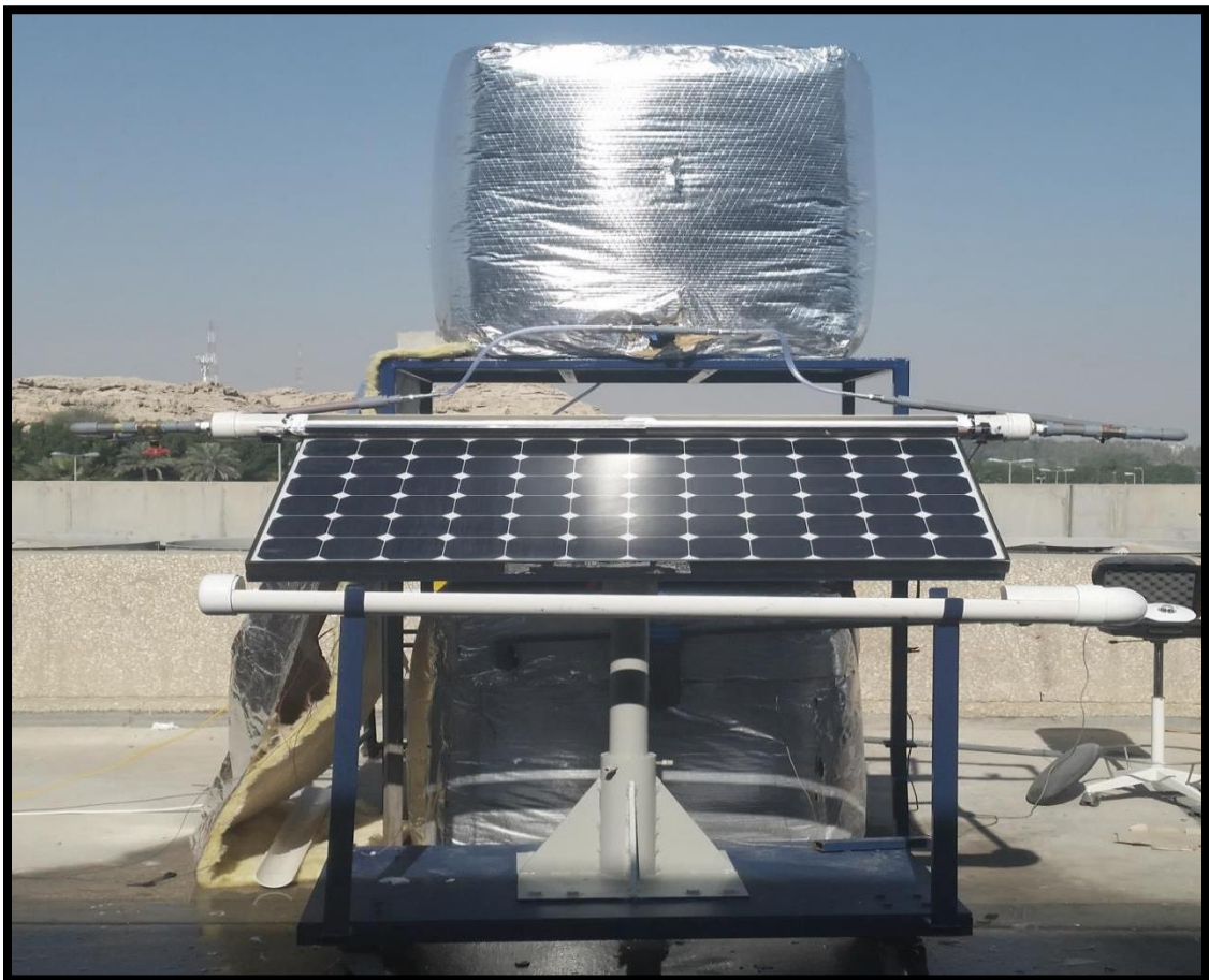
Figure 5-15 : Front view of manually PV cooling system
