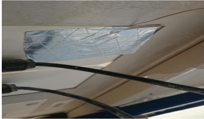
Figure 5-8: Thermocouple attached to the back of one of the solar cells
