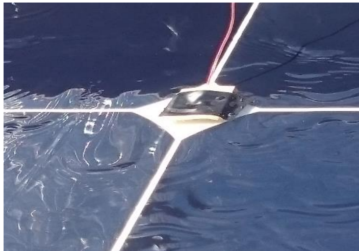
Figure 5-7: Thermocouple attached to the glass of the PV panel
