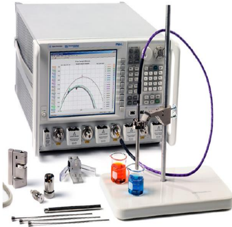
Figure 6: Keysight 85070E Dielectric Probe Kit, Dielectric experimental apparatus for powder samples
