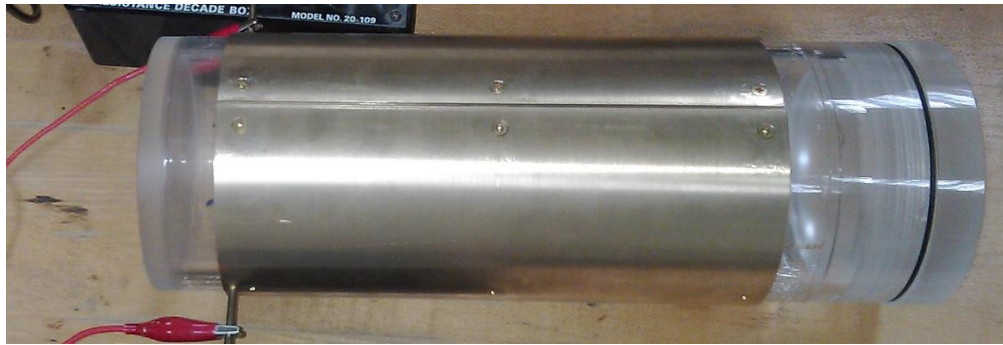
Fig.6.2: Plexiglass tube with copper plates outside the tube
