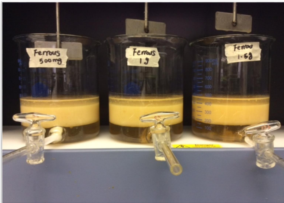
Figure 32: Separation after Jar test when ferrous sulphate added
