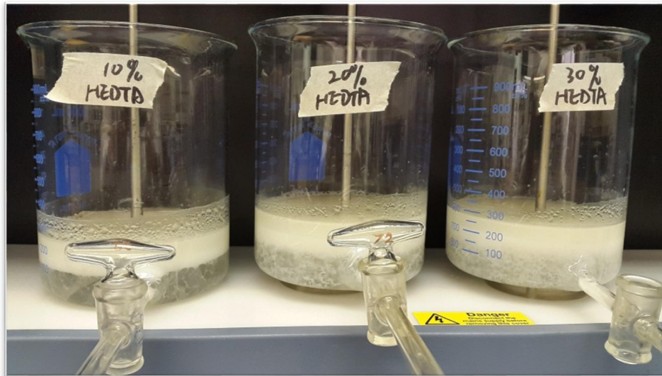
Figure 42: Separated water after Jar test at diluted concentration of HEDTA
