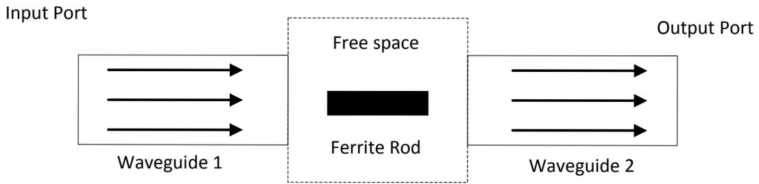
**Figure 12. HFSS simulation model for setup 2 - ferrite rod in free space between waveguides.**
