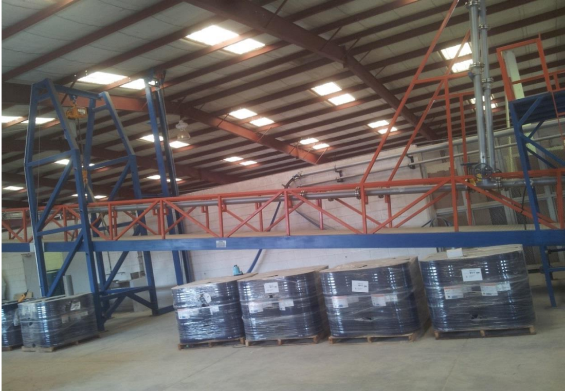
Figure 3.5:- Photograph of the Multiphase flow loop at 15 degree angle
