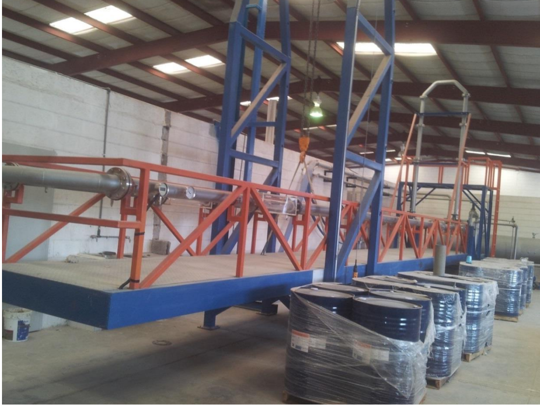
Figure 3.2:-Photograph of Multiphase flow loop in horizontal position
