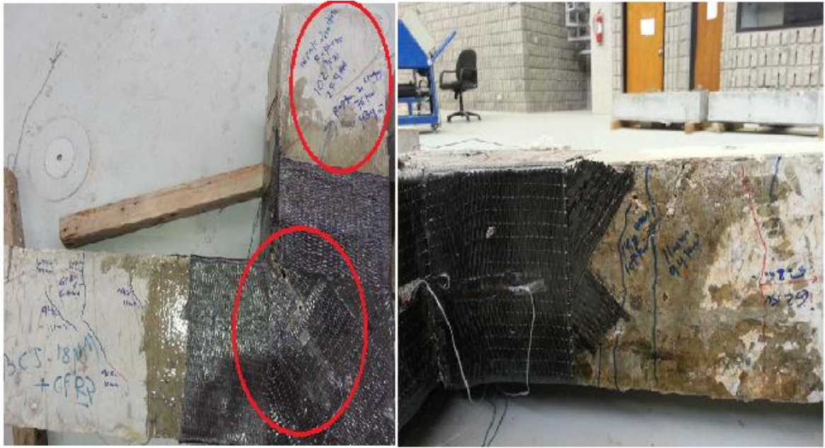
Figure 6.106: Damage propagation and crack pattern at displacement from the experimental test for BCJ-18MM-Bent In with CFRP
