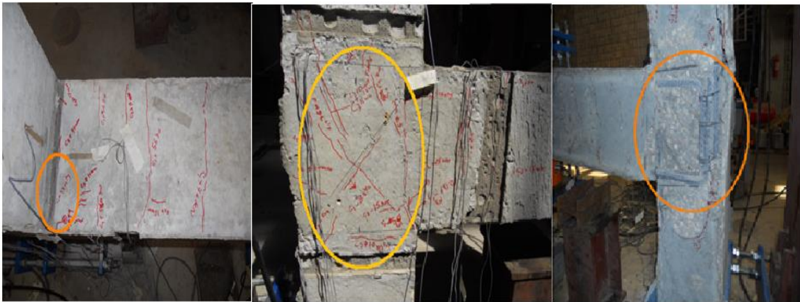
Figure 5.59: Crack pattern specimen BCJ-18MM- without CFRP
