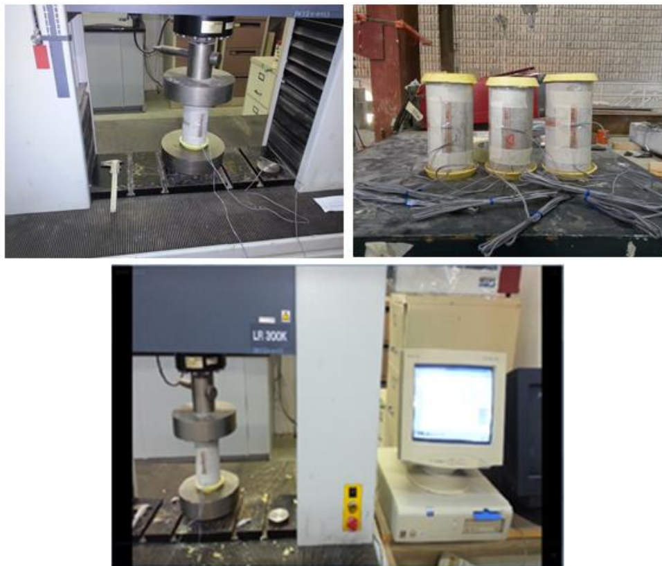
Figure 4.4: Cylinder test for concrete compressive strength
