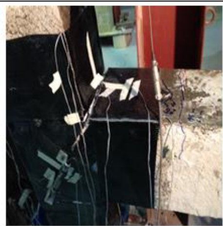
Flexural crack in BCJ interface at 74 KN
