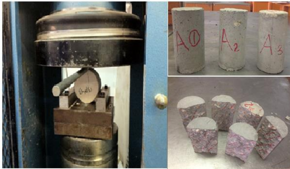
Figure 4.8: Concrete specimen under split test.
