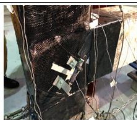
Rupture of CFRP in strong direction at 80KN and 21.7mm
