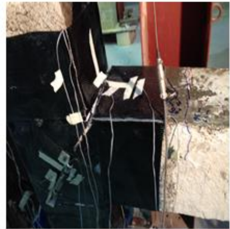
Flexural crack in BCJ interface at 74 kN
