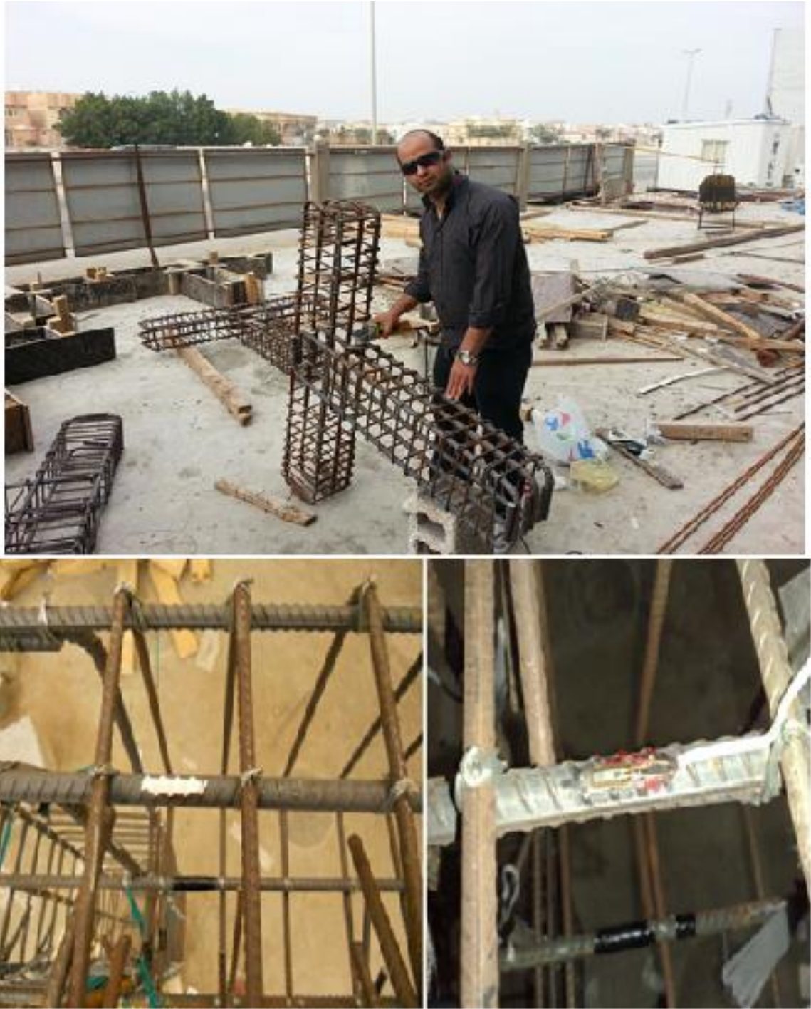
Figure 4.18: Surface preparation for installation of strain gauges
