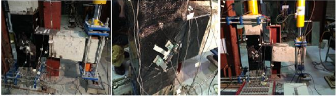
Figure 5.43: Crack pattern for specimen BCJ-12MM- with CFRP
