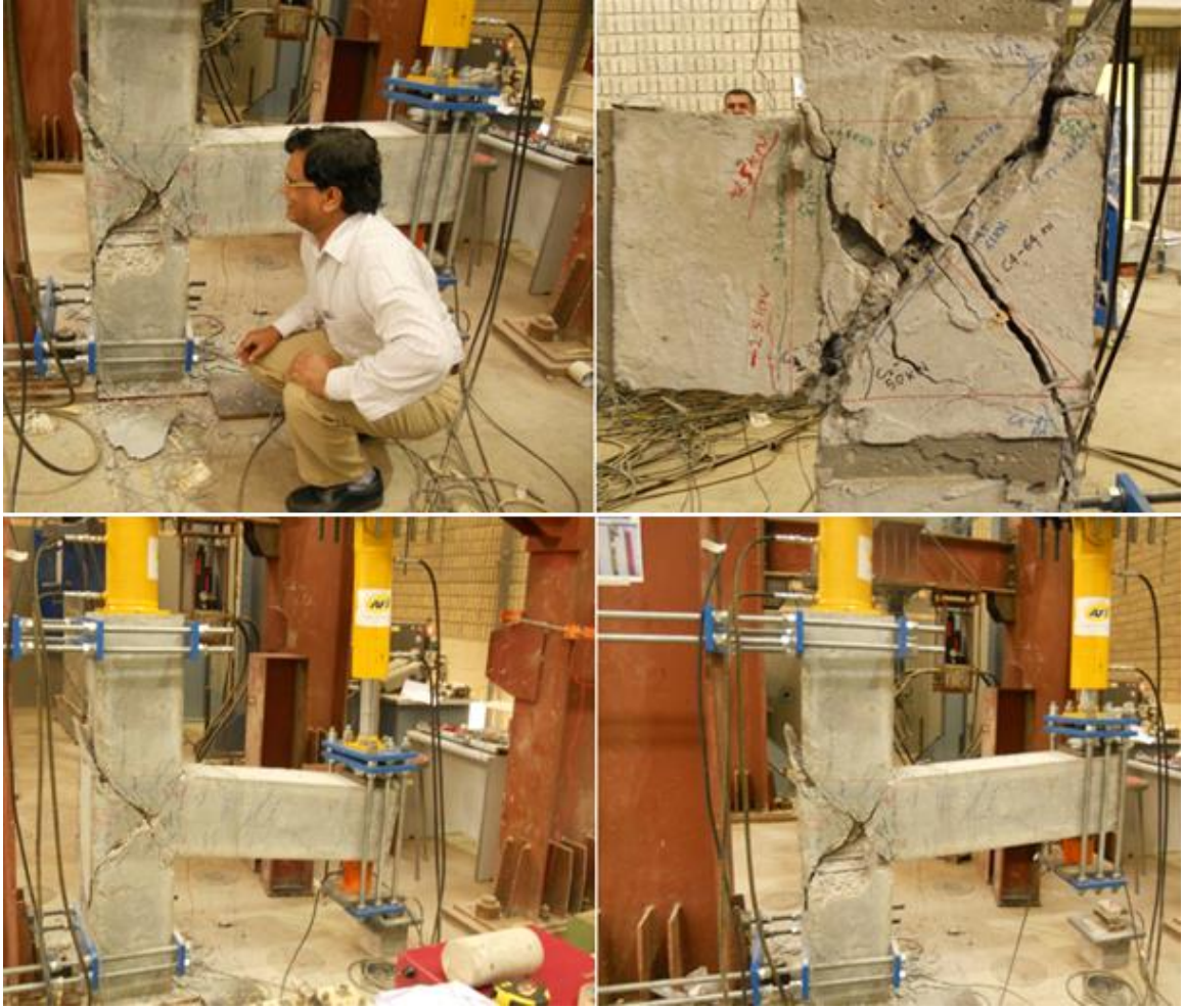
Figure 5.33: Crushing of joint and residual displacement in beam of specimen BCJ-12MM-Bent Up
