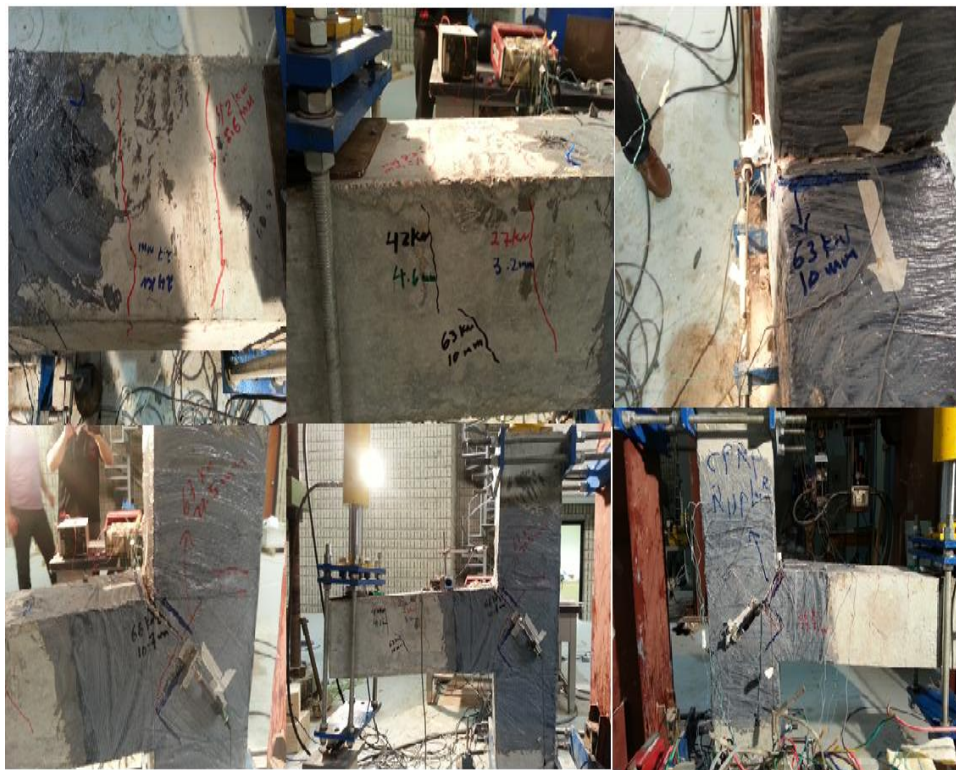
Figure 6.37: Damage propagation and crack pattern from experimental test for BCJ-12MM-Bent in with CFRP
