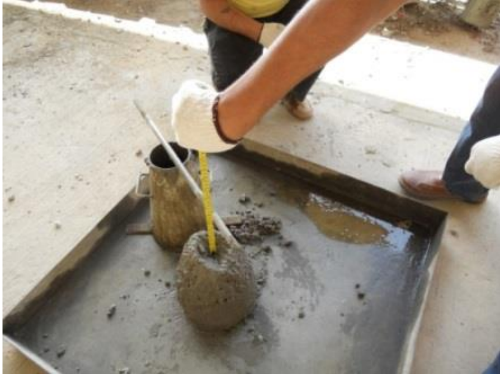
Figure 4.3: Slump test for fresh concrete
