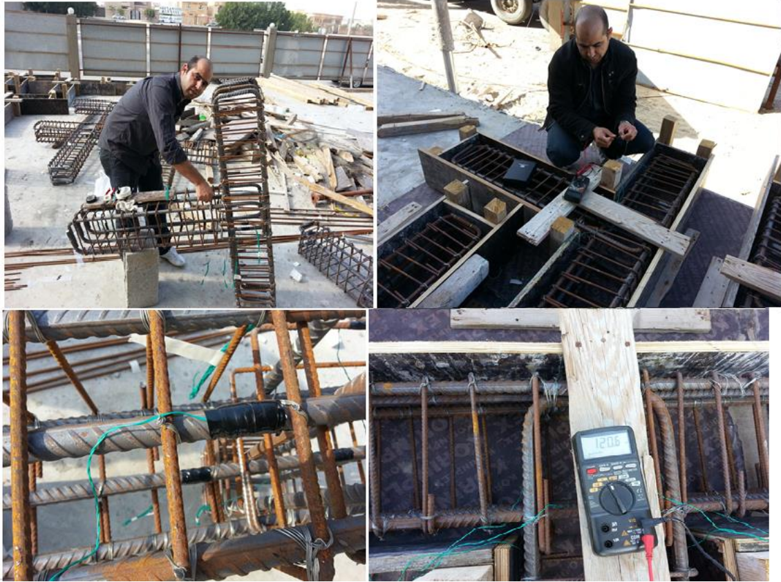
Figure 4.19: Installation of strain gauges and check the voltage reading
