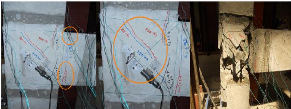
Figure 5.42: Crack pattern for specimen BCJ-12MM- without CFRP
