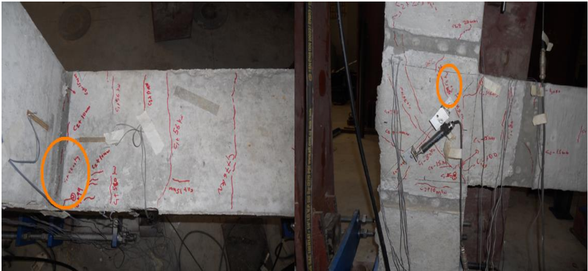
Figure 5.61: First flexural crack for specimen BCJ-18MM
