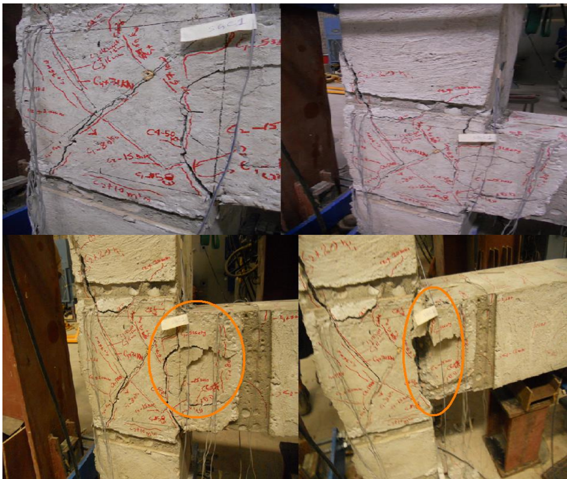
Figure 5.63: Formation of crack in joint during cyclic load test in specimen BCJ-18MM
