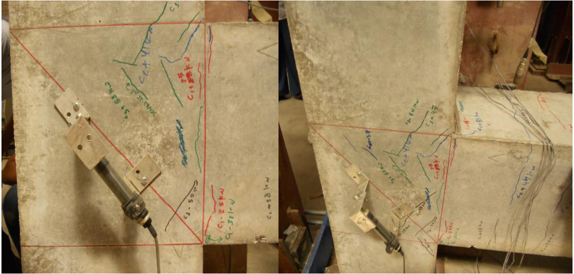
Figure 5.30: Formation of crack in joint during cyclic load test in specimen BCJ-12MM-Bent Up
