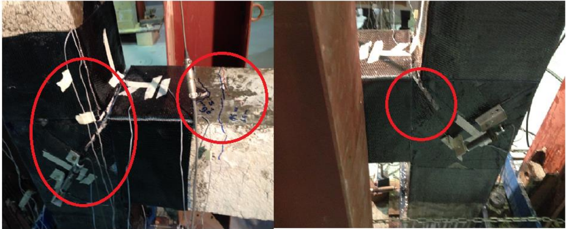
Figure 6.74: Damage propagation and crack pattern from experimental test for BCJ-12MM-Bent up with CFRP
