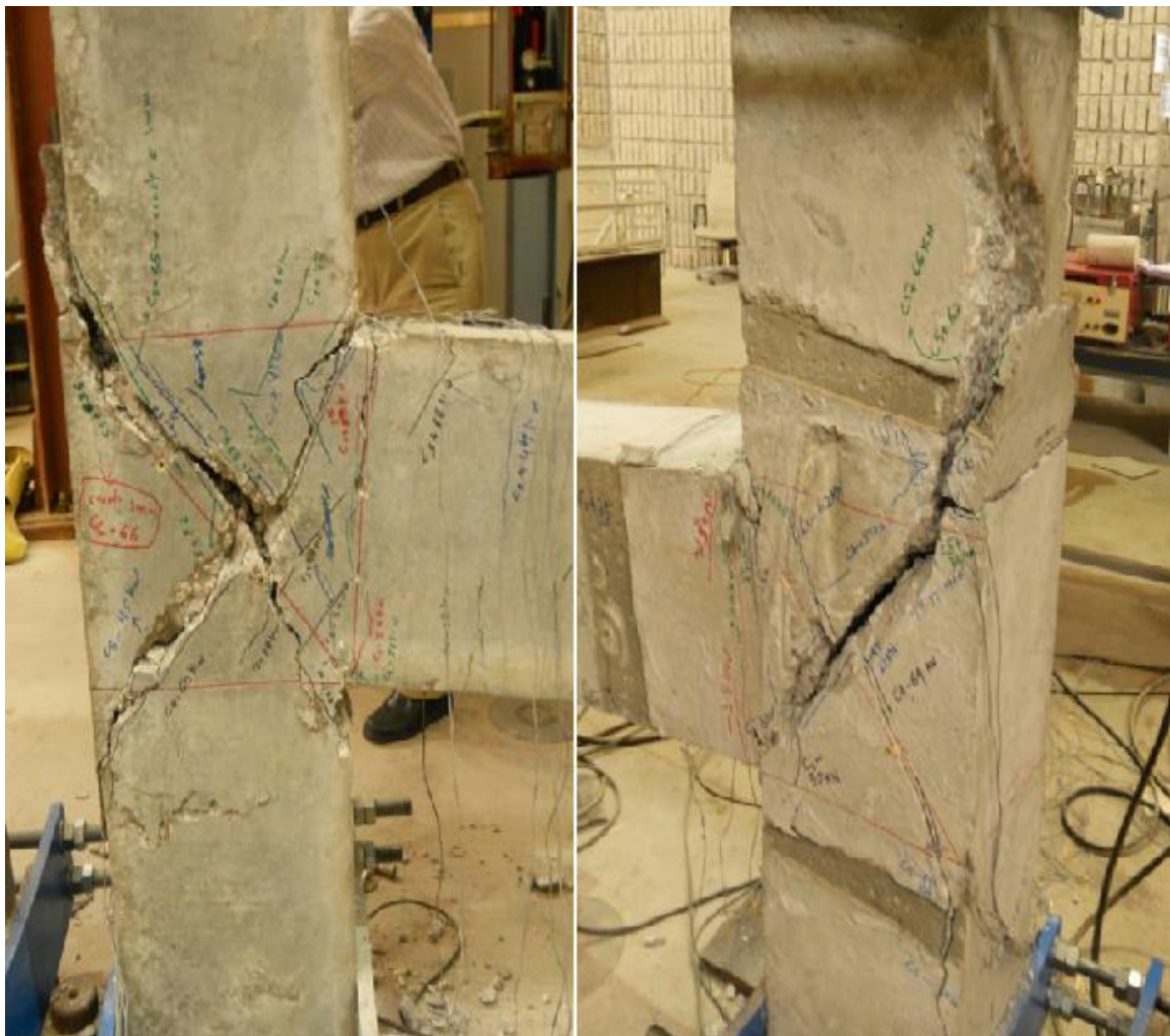
Figure 5.32: Failure of specimen BCJ-12MM-Bent Up
