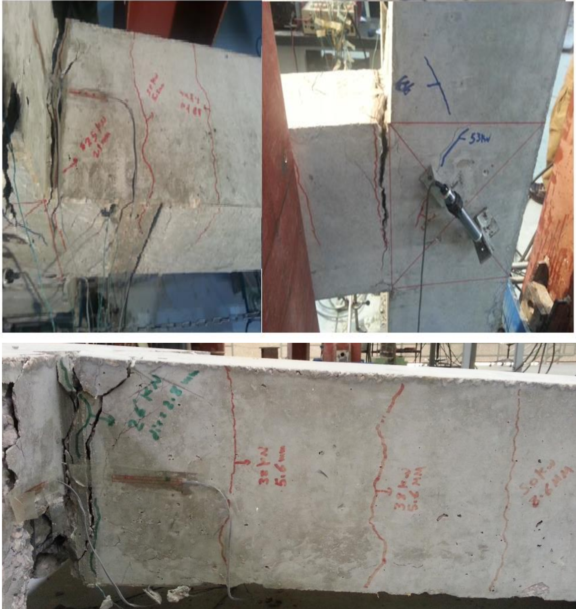
Figure 6.21: Damage propagation and crack pattern from experimental test for BCJ-12MM-Bent in without CFRP
