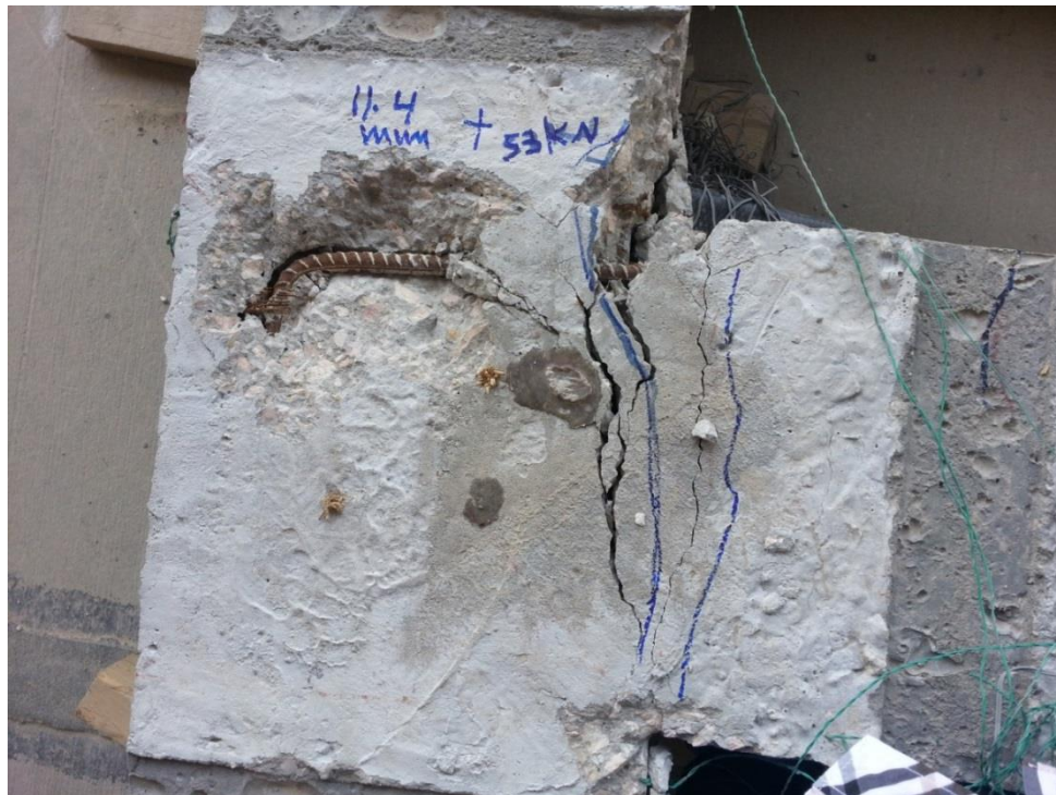
Figure 6.57: Damage propagation and crack pattern from experimental test for BCJ-12MM-Bent Up without CFRP
