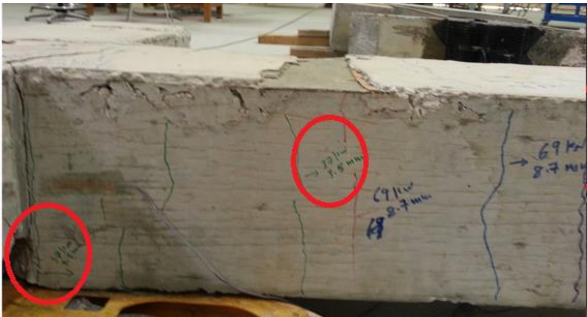
Figure 6.85: Damage propagation and crack pattern from experimental test for BCJ-18MM-Bent In without CFRP
