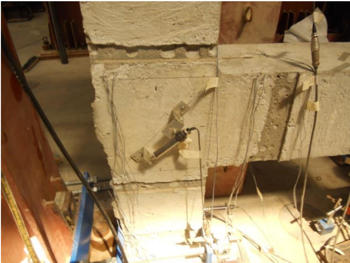
Figure 5.65: Position of LVDT J1 in joint to observe diagonal crack
