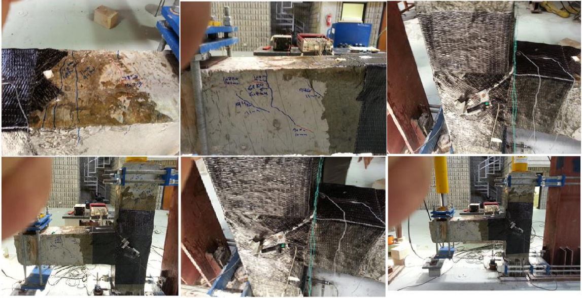
Figure 5.19: Crack pattern Specimen BCJ-18MM- Bent In with CFRP
