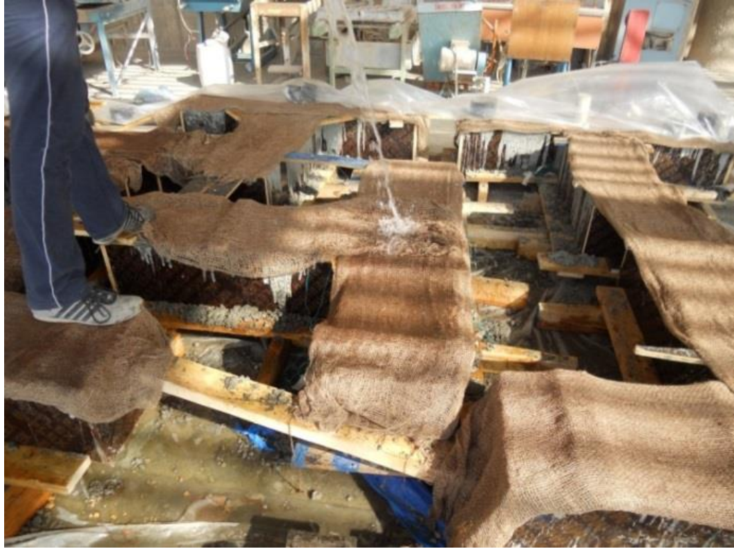
Figure 4.21: Specimens covered with wet burlap for curing
