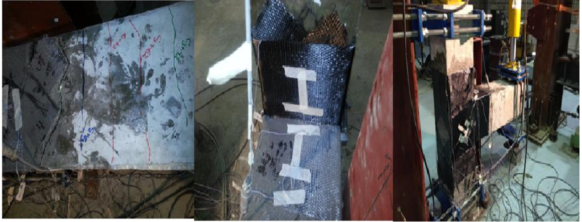
Figure 5.60: Crack pattern specimen BCJ-18MM- with CFRP
