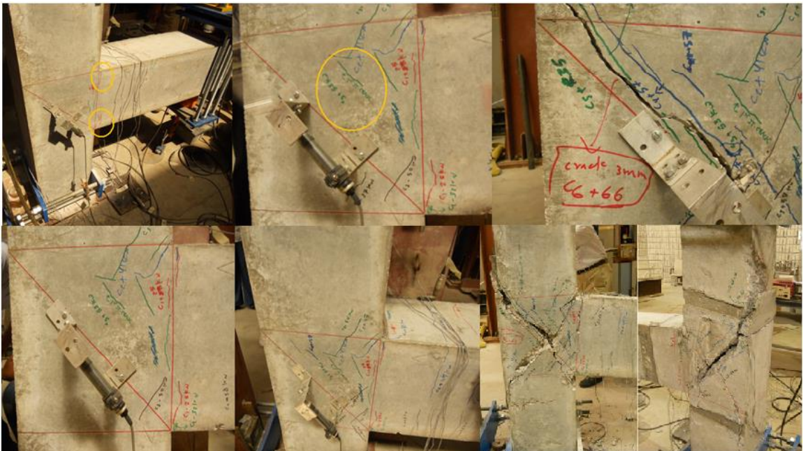
Figure 5.26: Crack pattern for specimen BCJ-12MM-Bent Up without CFRP
