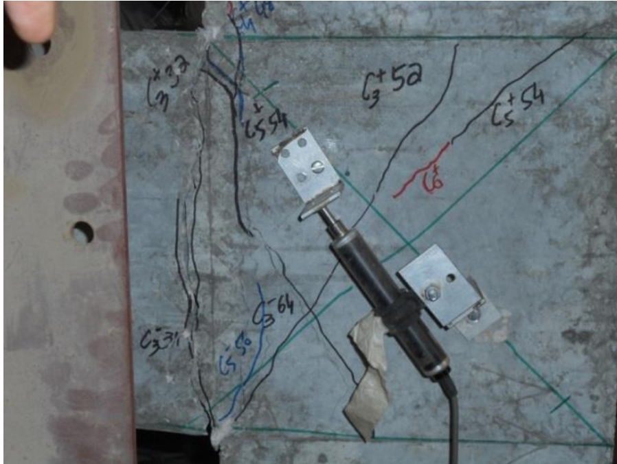
Figure 5.50: Position of LVDT J2 in joint to observe diagonal crack
