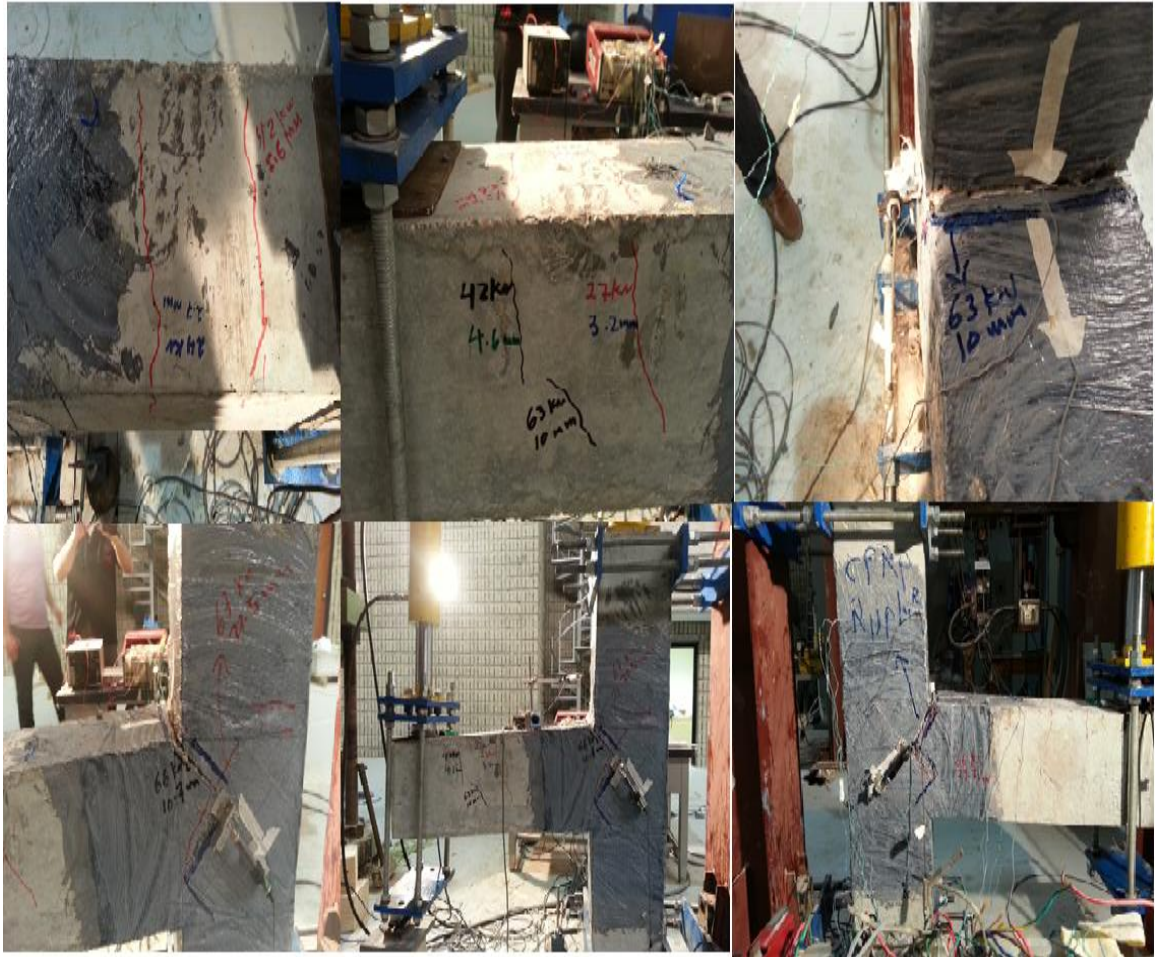
Figure 5.11: Crack pattern specimen BCJ-12MM- with CFRP
