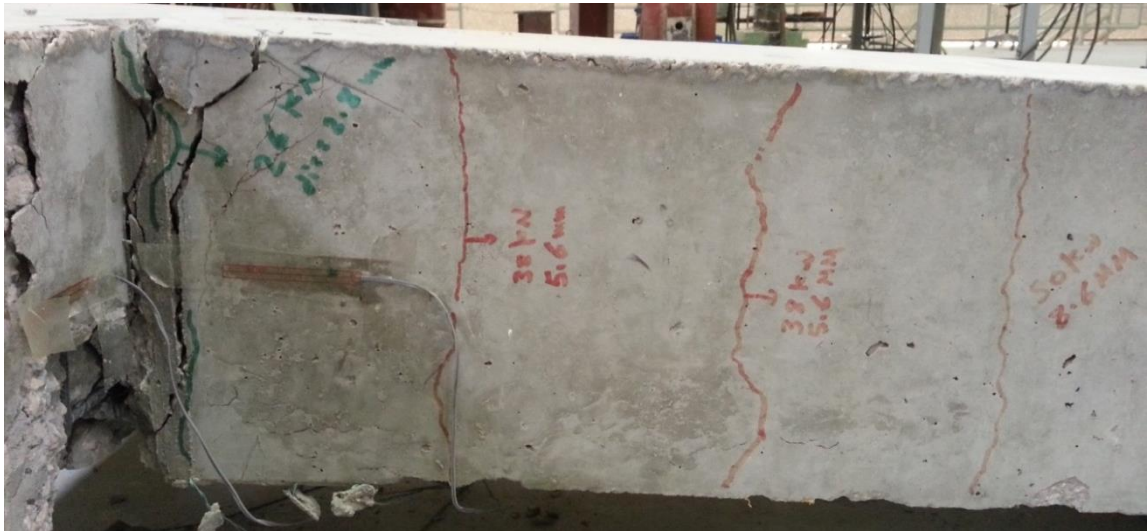
Figure 6.23: Damage propagation and crack pattern from experimental test for BCJ-12MM-Bent in without CFRP
