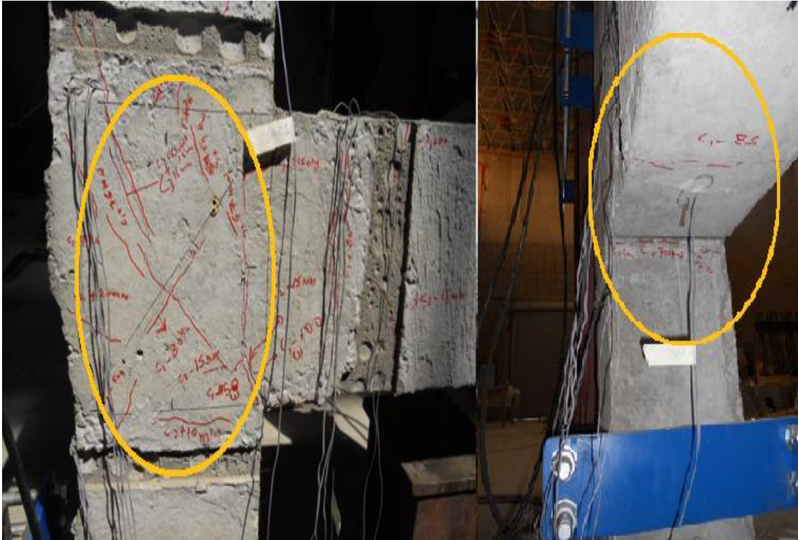
Figure 5.62: First diagonal crack in joint for specimen BCJ-18MM
