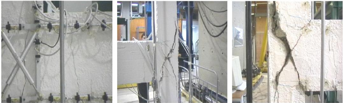
Figure 2.22: T-Joint specimen: beam and joint panel cracks pattern at failure [(Braga, Gigliotti et al. 2009)]
