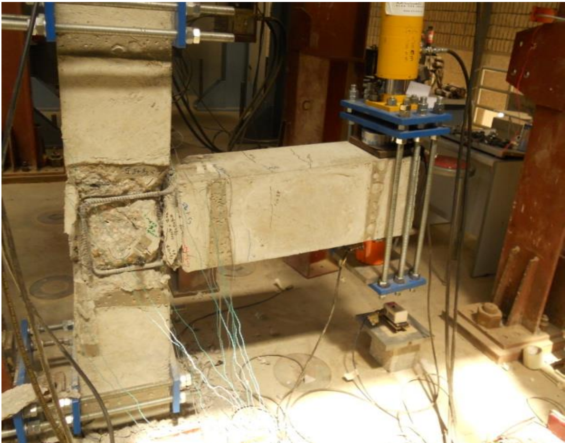
Figure 5.48: Residual displacement in beam for specimen BCJ-12MM-Bent In
