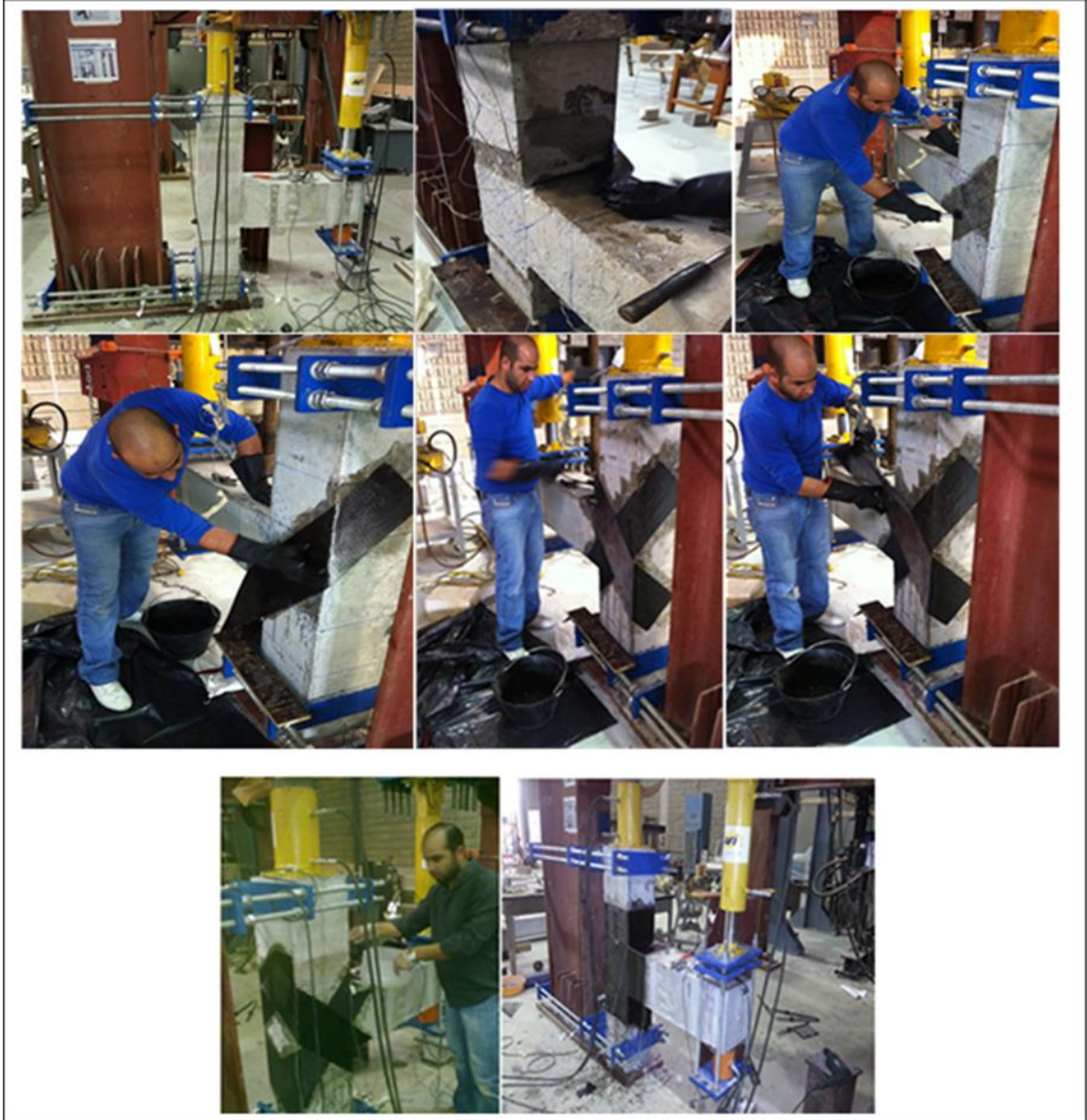
Figure 4.32: Sequence applying the CFRP sheet
