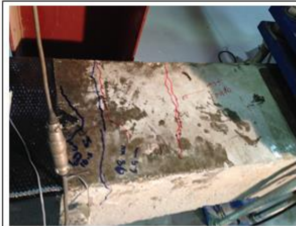
Fisrt flexural crack in beam at 48KN
