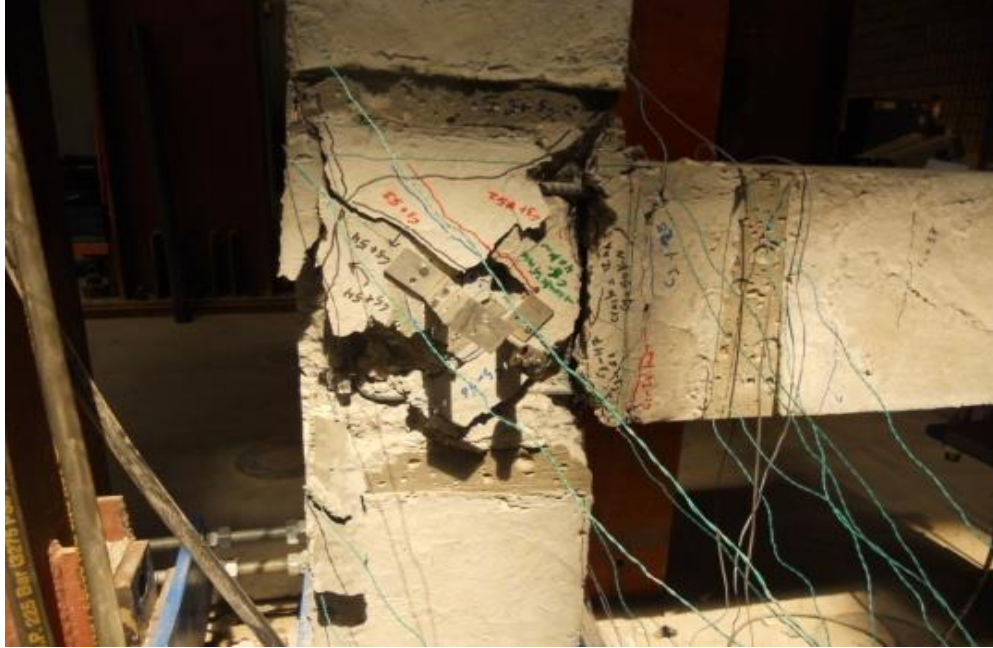
Figure 5.47: Spilling of concrete in joint region for specimen BCJ-12MM-Bent
