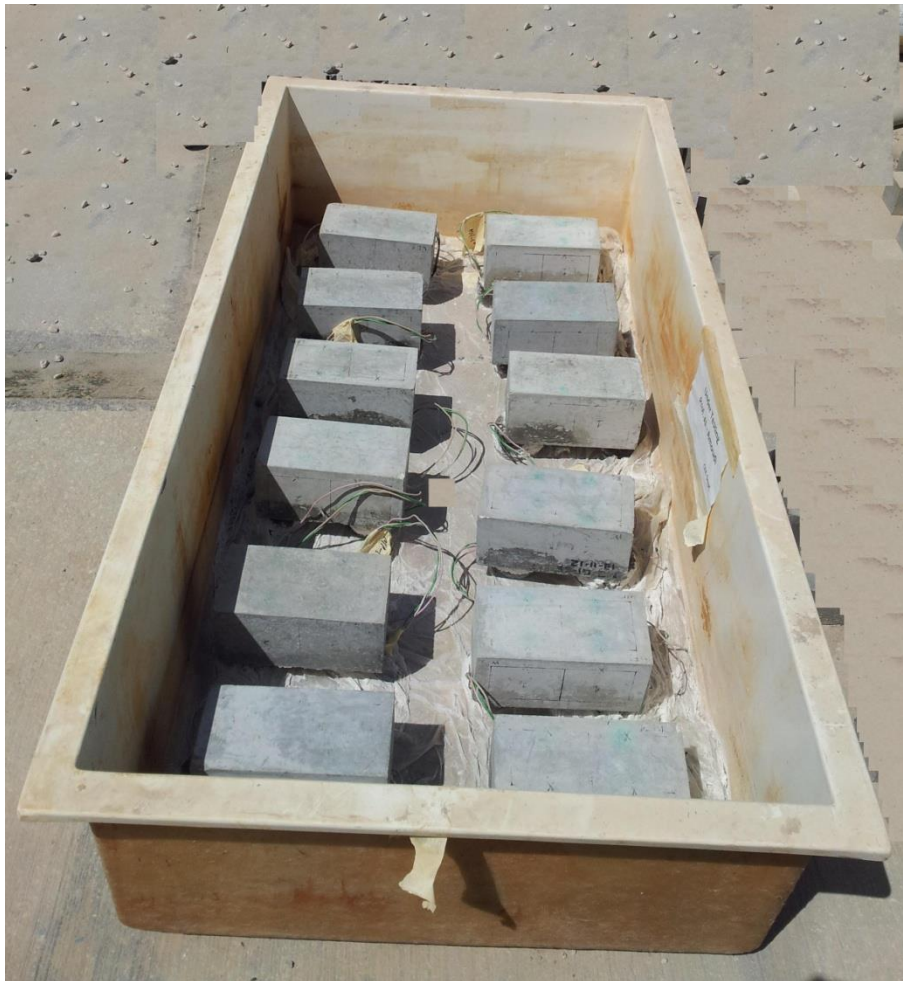
Figure 3.8 Concrete Beam Specimens in the Atmospheric Zone.
