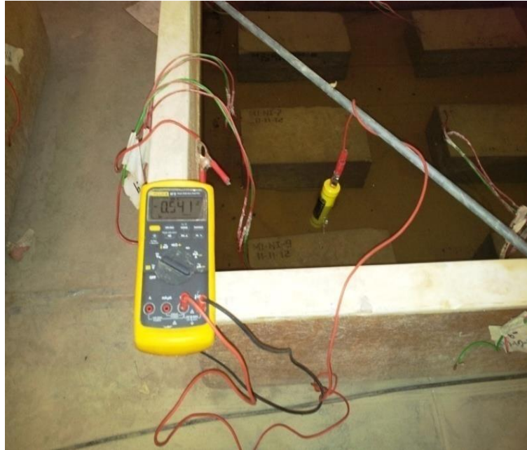
Figure 3.22 Methodology to Measure the Corrosion Potential on Concrete Beam Specimens in Submerged Zone.
