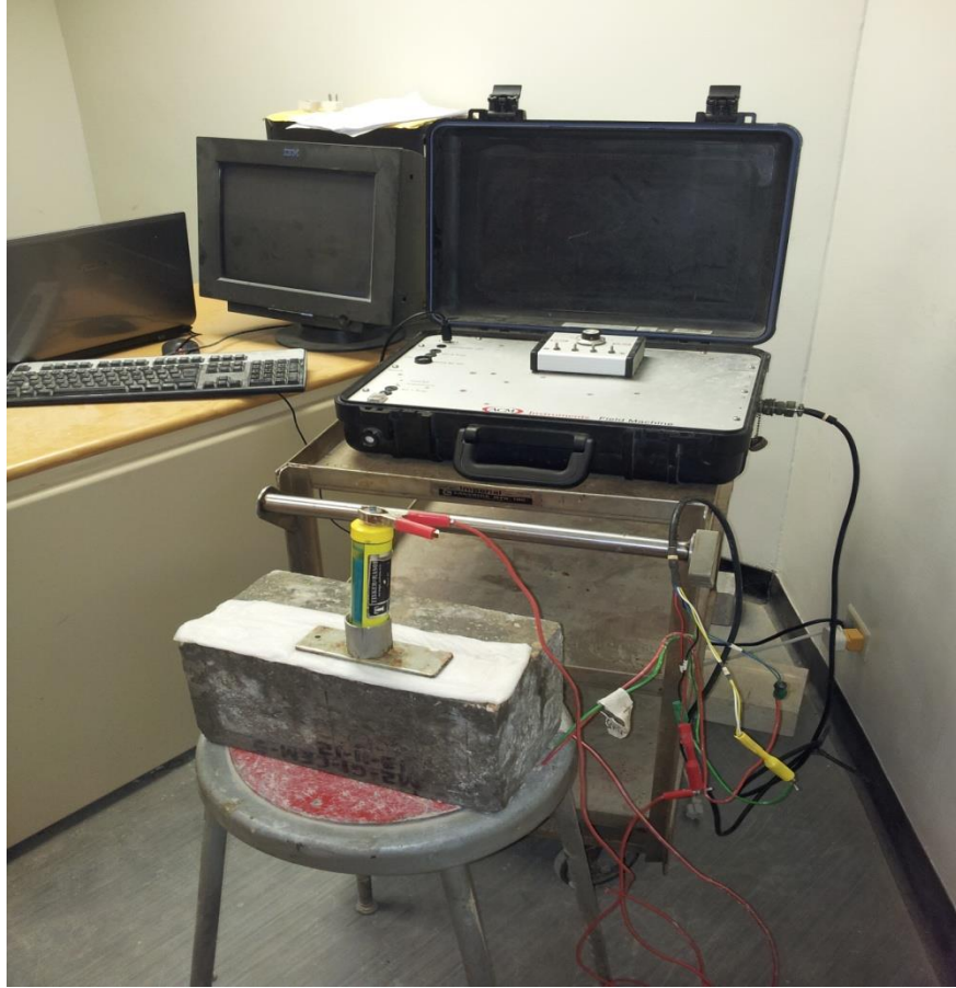
Figure 3.24 Methodology to Measure the Corrosion Current Density on Concrete Beam Specimens in the Atmospheric and Tidal Zones.
