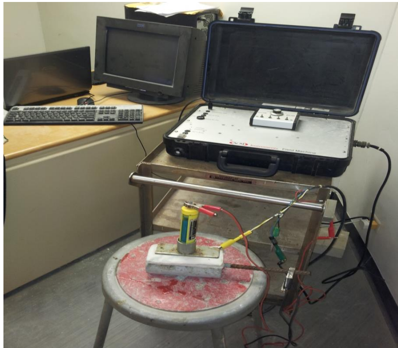
Figure 3.27 Methodology to Measure the Corrosion Current Density on Concrete Cylindrical Specimens.
