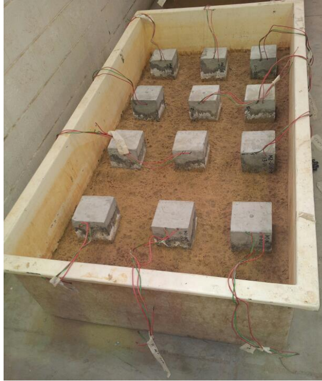
Figure 3.18 Concrete Beam Specimens Placed in the Capillary Zone.
