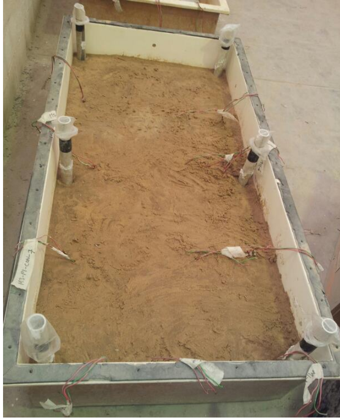
Figure 3.16 Concrete Beam Specimens in the Below Ground Zone.
