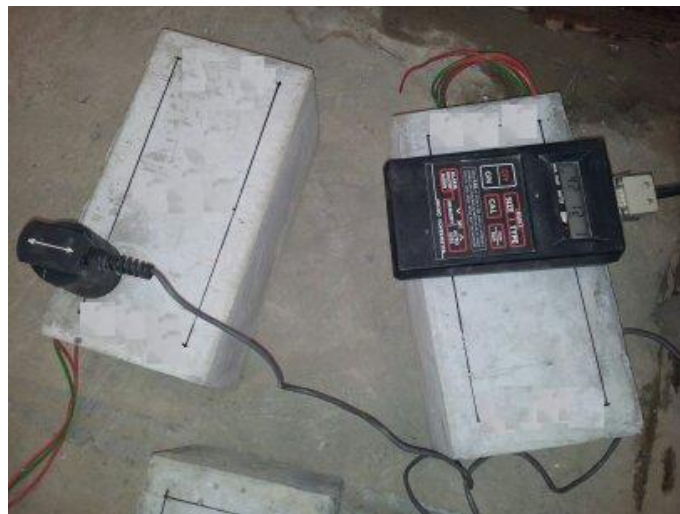
Figure 3.19 Position of Steel Bars Measured with the Help of Cover Meter.
