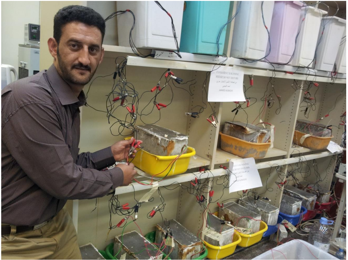
Figures 3.30 Concrete Beam Specimens under Test for the Accelerated Corrosion.
