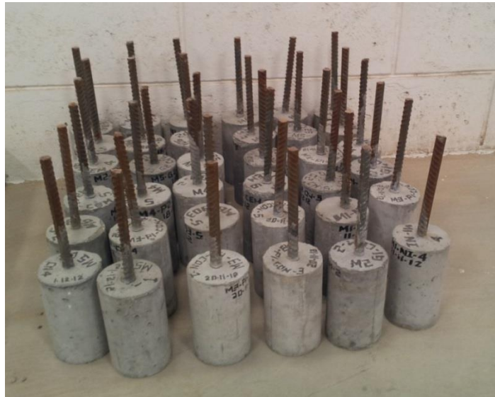
Figure 3.6 Concrete Cylindrical Specimens.
