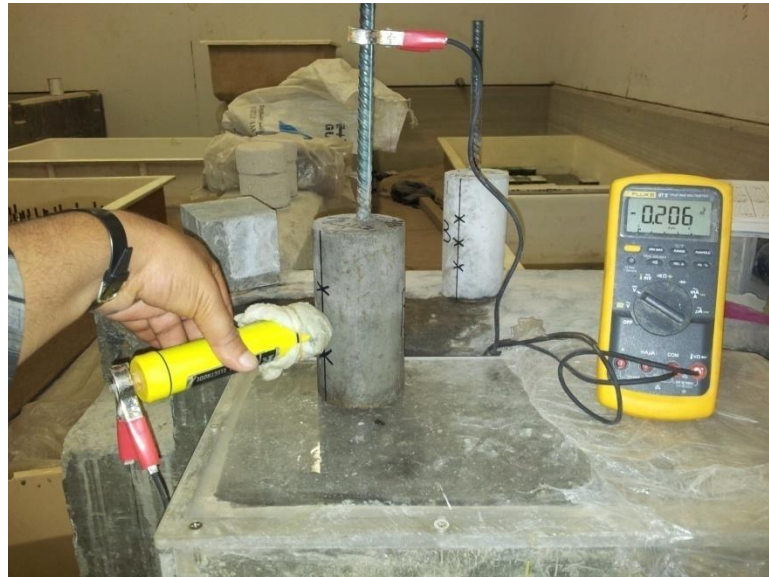
Figure 3.23 Methodology to Measure the Corrosion Potential on Concrete Cylindrical Specimens.
