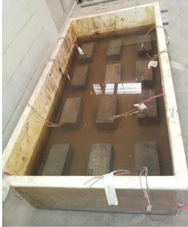
Figure 3.14 Concrete Beam Specimens in the Submerged Zone.
