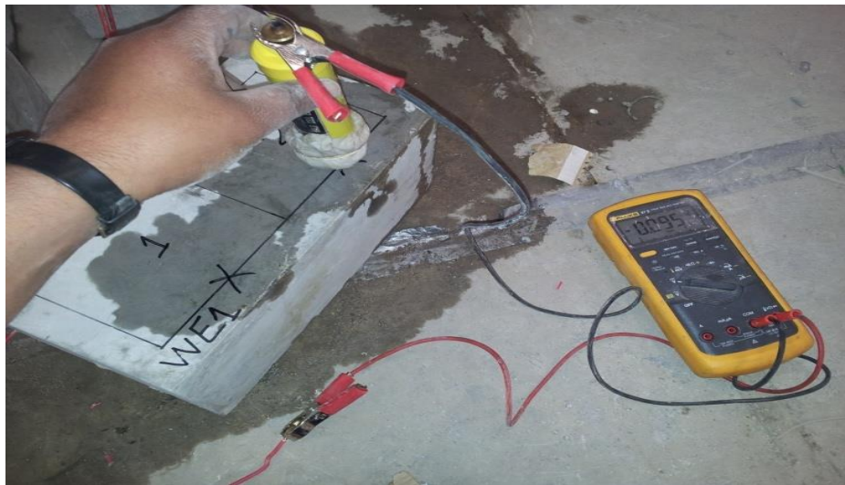
Figure 3.20 Methodology to Measure the Corrosion Potential on Concrete Beam Specimens in the Atmospheric and Tidal Zones.
