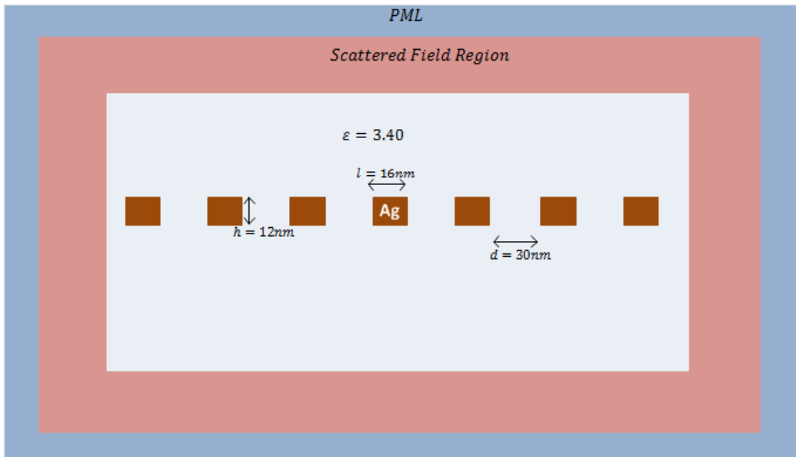
Figure 5.15 Optimized Configuration with silver rectangles embedded in phosphor layer.
