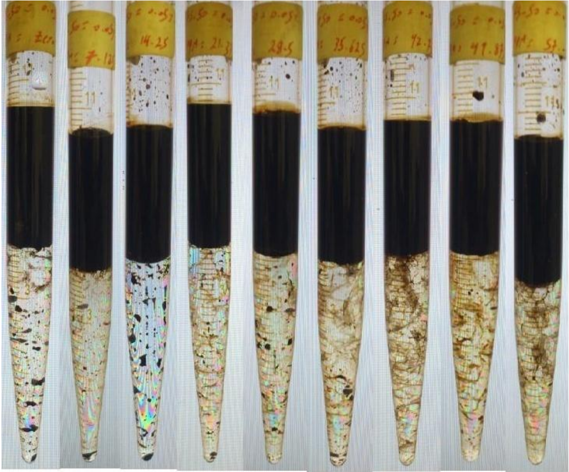
Figure 4. 31: Phase behavior for FS-50 (0.1 wt%) at 90°C after 30 days
