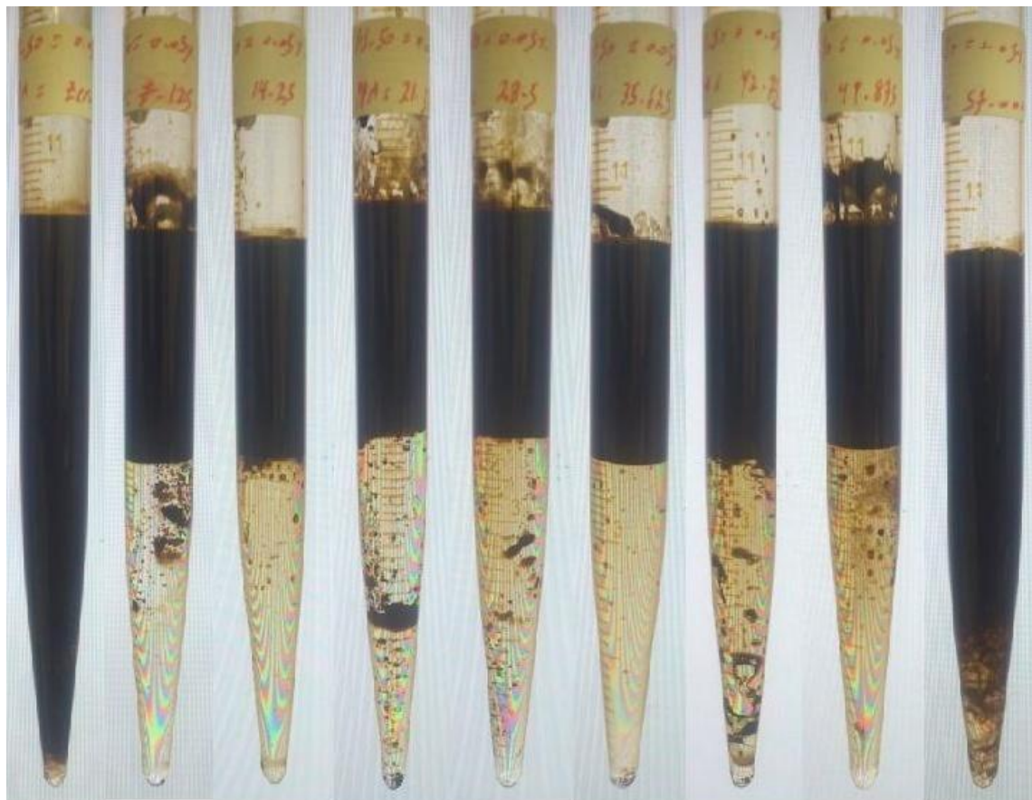
Figure 4. 30: Phase behavior for FS-50 (0.1 wt%) at 25°C after 30 days
