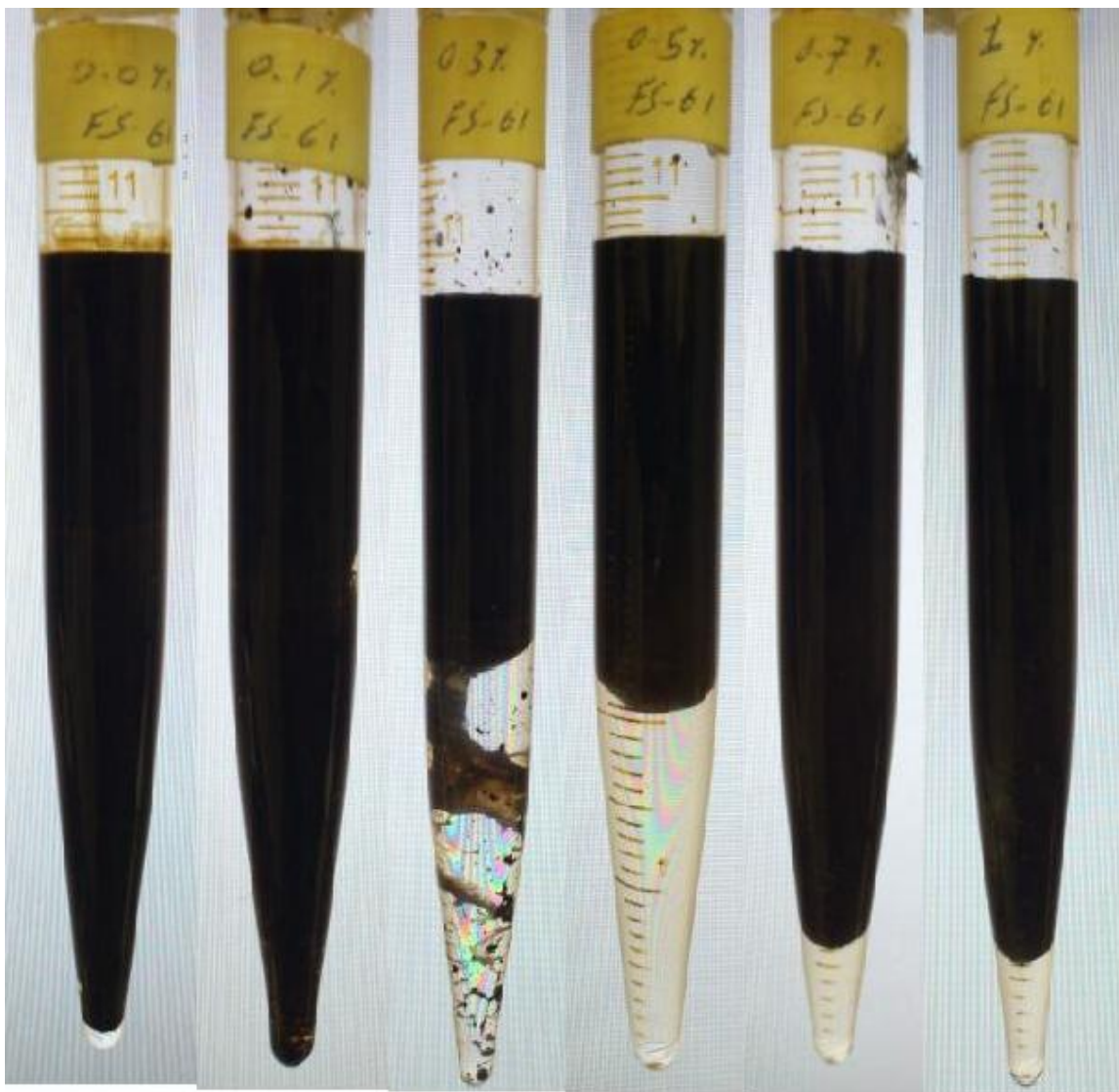
Figure 4. 28: Phase behavior for surfactant FS-61 in deionized water at 90°C after 15 days
