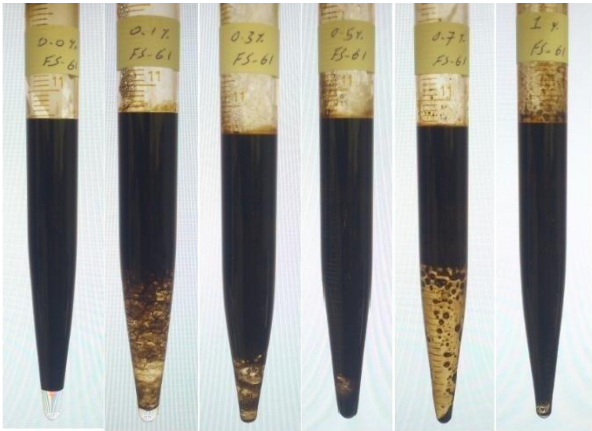
Figure 4. 27: Phase behavior for surfactant FS-61 in deionized water at 25°C after 30 days
