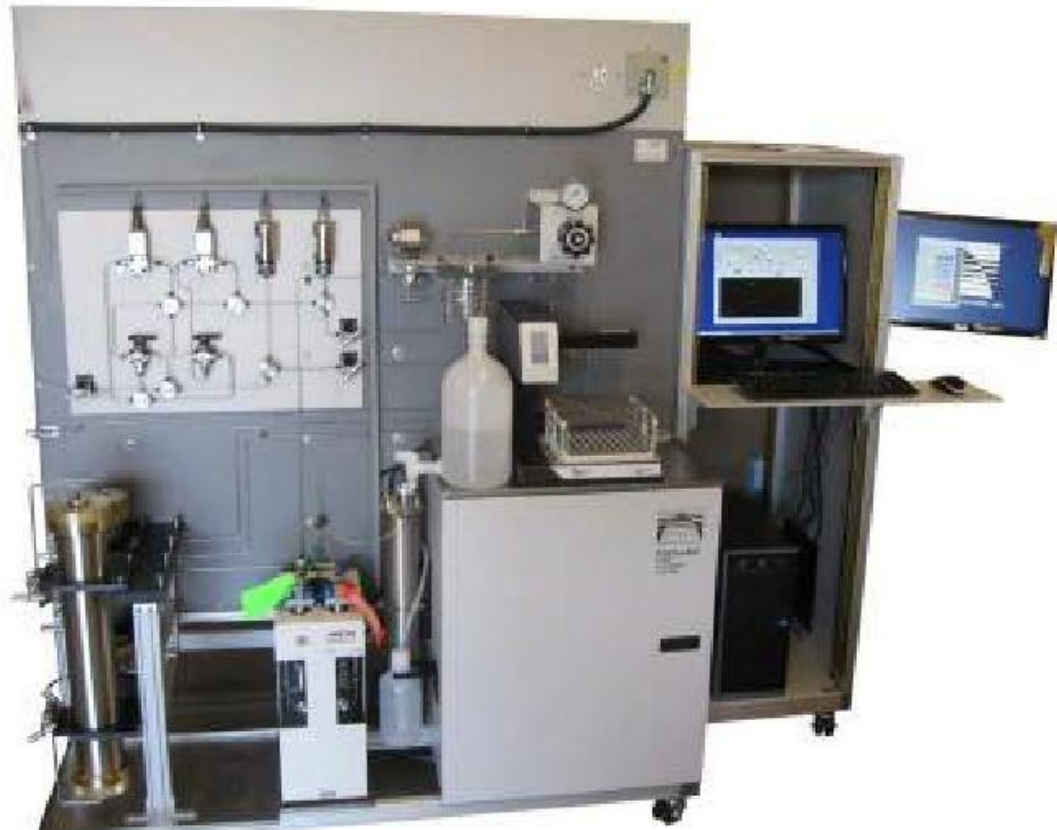
Figure 3.6: Core flooding system (CoreTest FDES-645)
