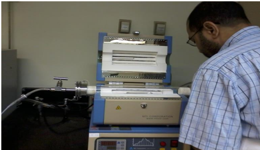
Figure 3: High temperature Vacuum tube furnace used for the heat treatment of the synthesized catalysts.
