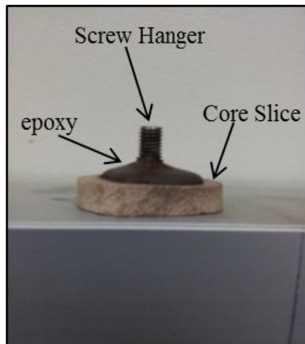
Figure 6.3 Rock slice-hanger assembly
