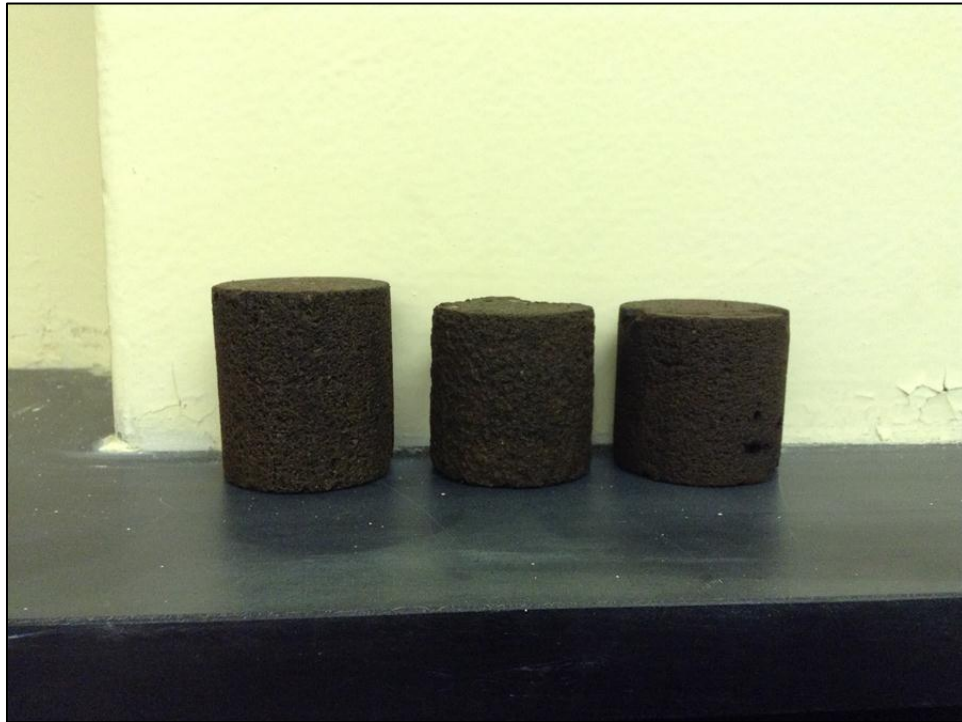
Figure 6.6 The three core plugs used in the core flooding experiment
