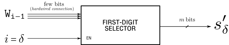
Figure 4.4: The First-Digit Selector. Note that the selector gets its inputs from the W register through hardwired connections.
