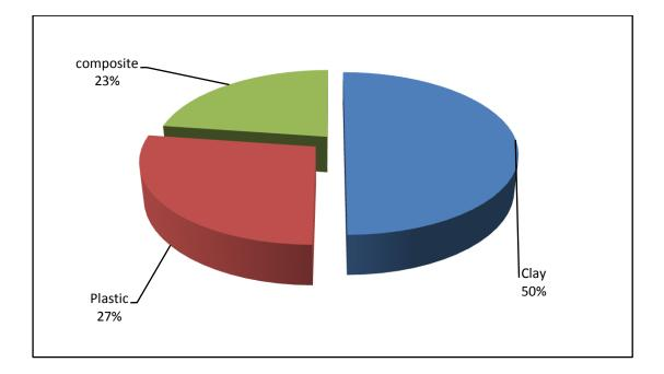
Figure 15.Materials used as landfill or pit bottom liner
