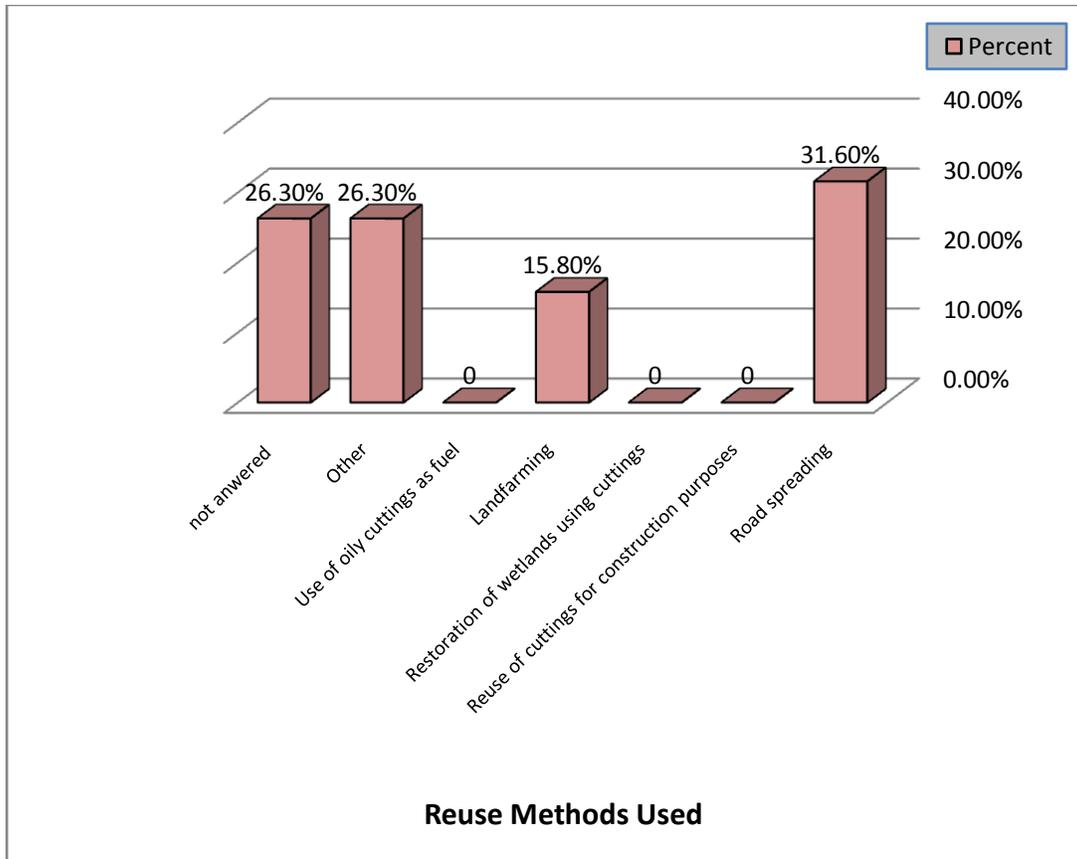
Figure 9. Methods used by drilling companies to reuse waste drilling
