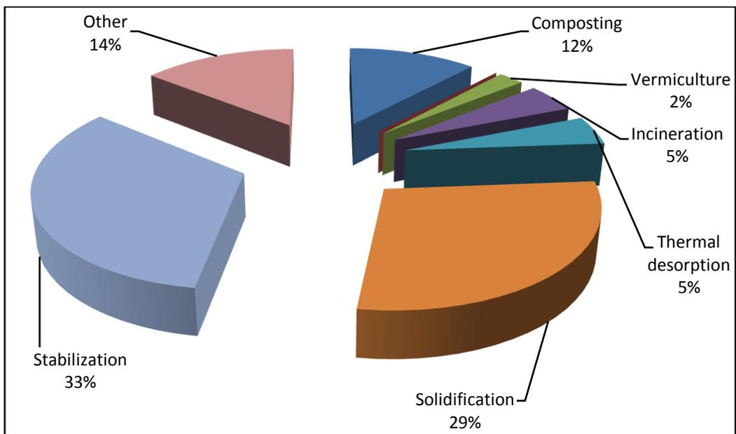
Figure 13. Treatment methodology and technologies used to treat drilling wastes
