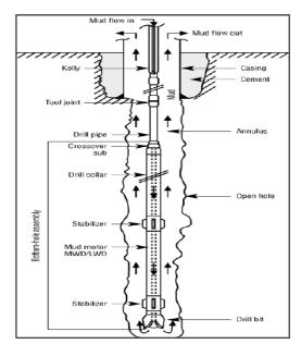
Figure 2. Drilling steps using drilling fluids (Candler, 2008)
