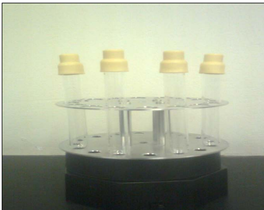
Figure 5: Portable sample carousel holding the quartz tubes.
