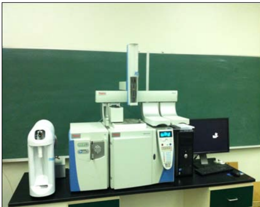
Figure 6: Thermo Scientific Trace GC ultra with ISQ mass spectrometer and TriPlus headspace and autosampler.
