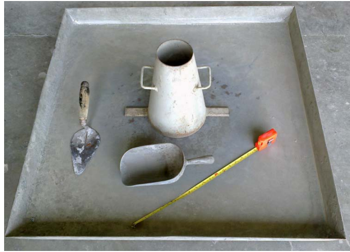
Figure 3.3: Slump flow measurement equipments and accessories.
