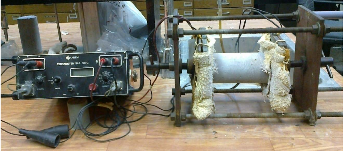
Figure 4.9: Test set-up for electrical resistivity.
