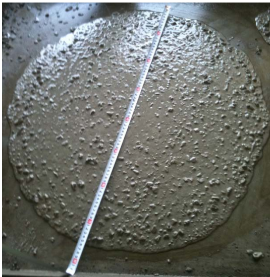
Figure 2.5: SCC filling ability tests (a) Flow table/slump flow test (b) V-funnel test.
