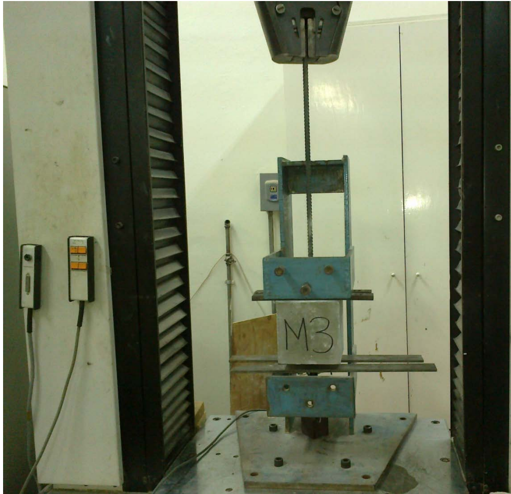
Figure 4.6: Test arrangement for the pull-out test.
