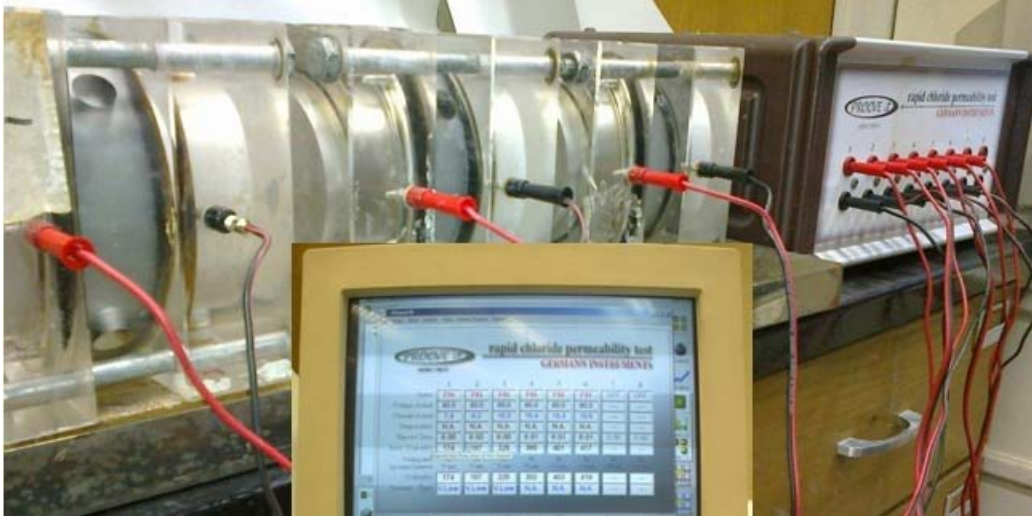
Figure 4.8: Rapid chloride permeability test set-up.
