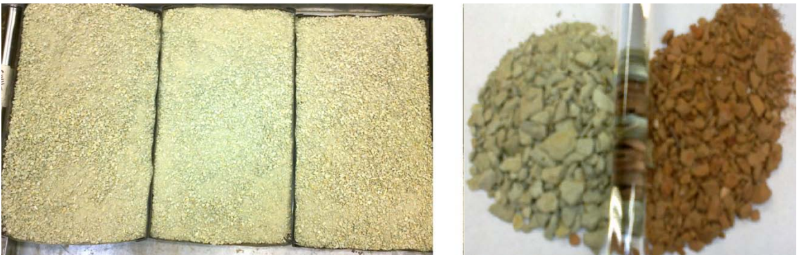
Figure 3.2: (a) Crushed clay laid in furnace trays (b) Raw clay and activated clay shown side-by-side.
