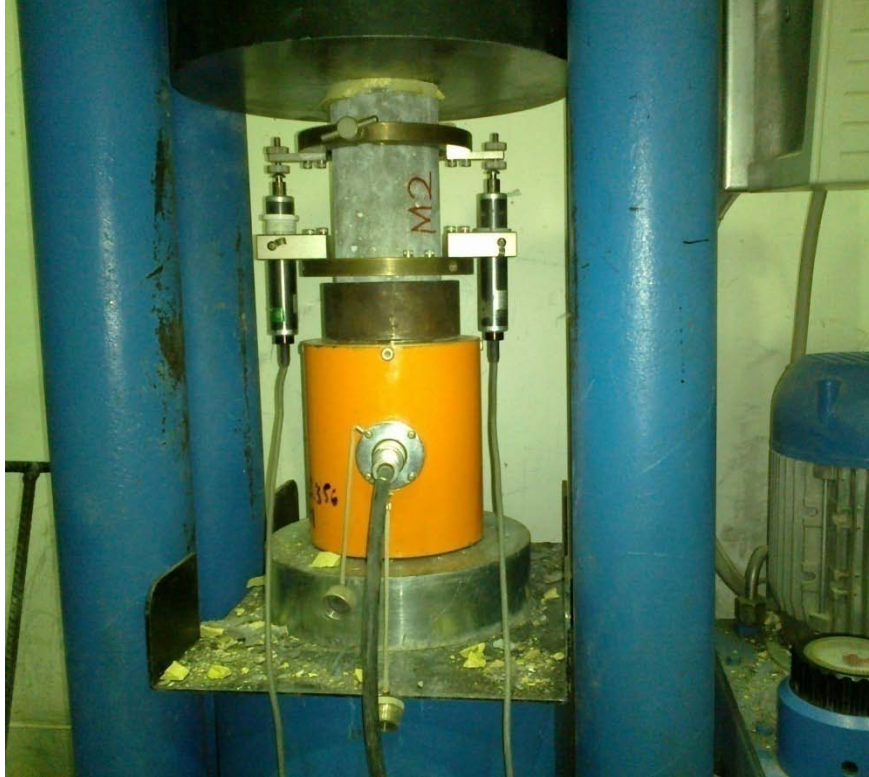
Figure 4.4: Test arrangement for determining Young's modulus
