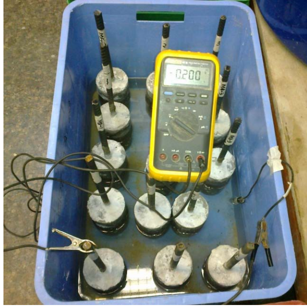
Figure 4.11: Corrosion potential measurement setup.
