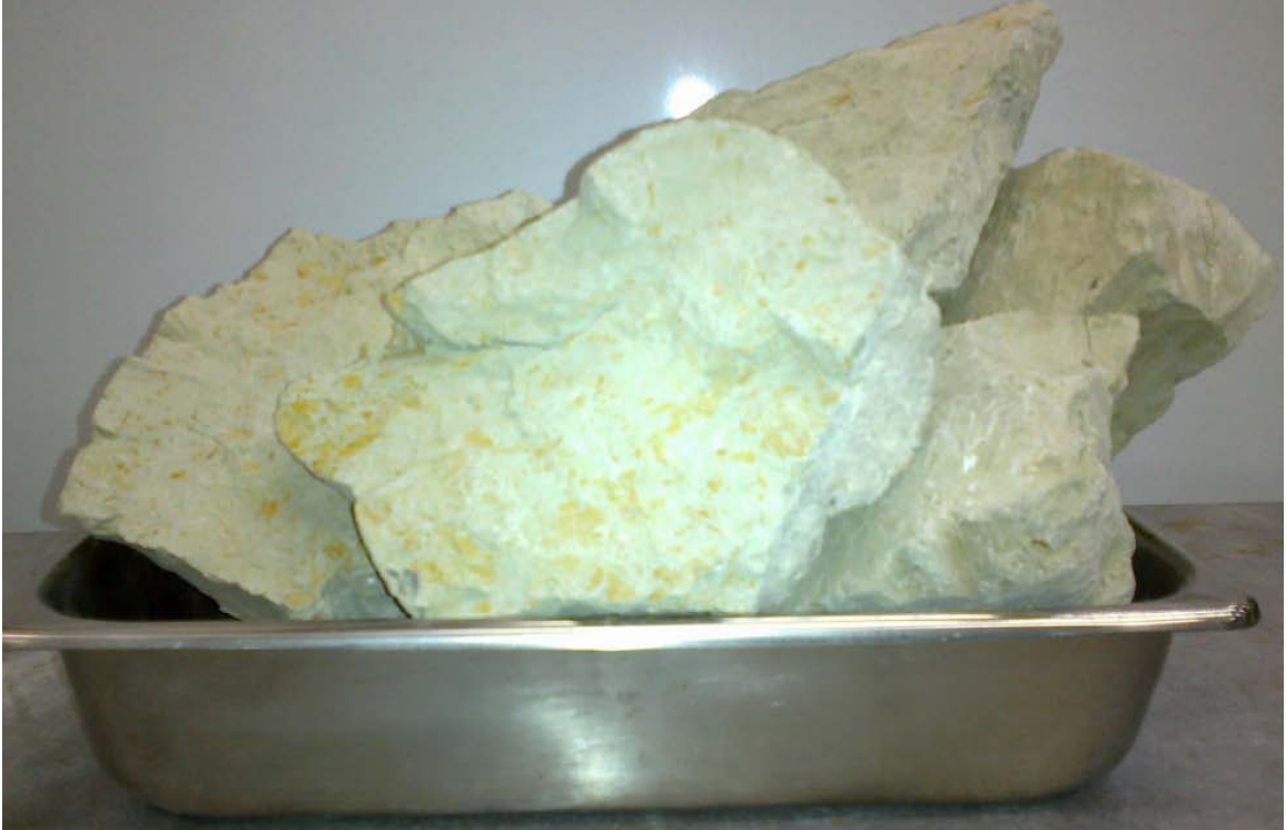
Figure 3.1: Raw clay before processing.
