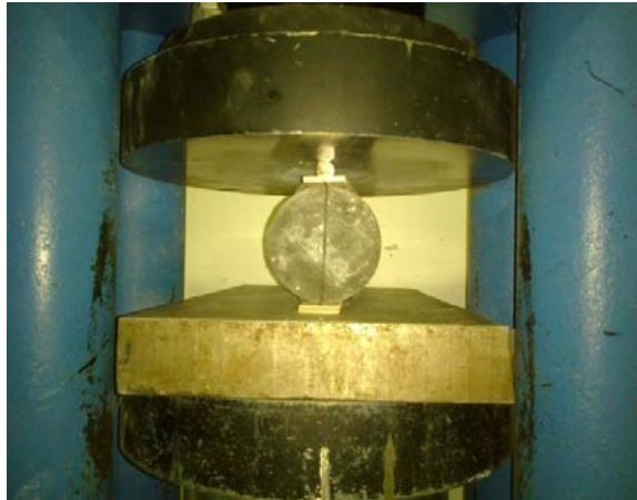
Figure 4.2: Test arrangement for splitting tensile strength.
