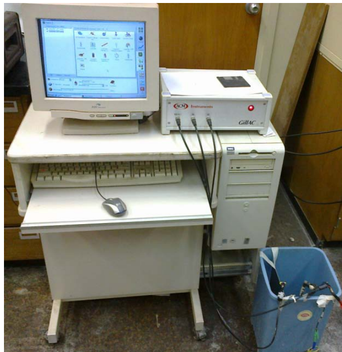
Figure 4.12: Corrosion current density measurement setup.
