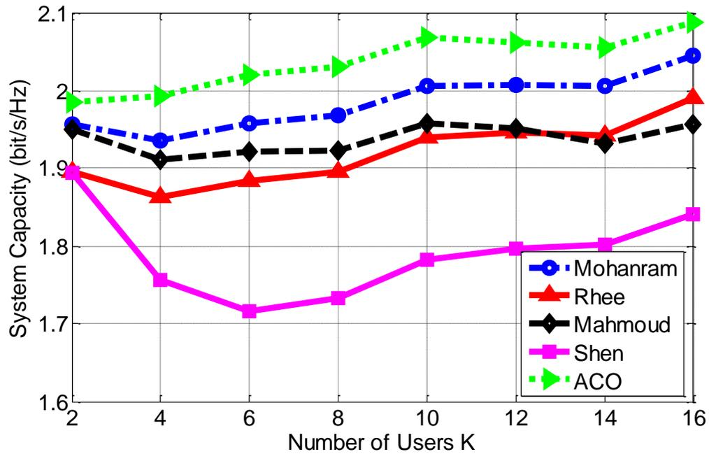
Figure 4.19: Comparison of total system capacity versus number of users for ACO-based algorithm version 3 and other algorithms for  $\gamma_i = 1 \forall (i \% 2) = 1$  and  $\gamma_i = 8 \forall (i \% 2) = 0$  for  $i = 1, 2, \dots, K$
