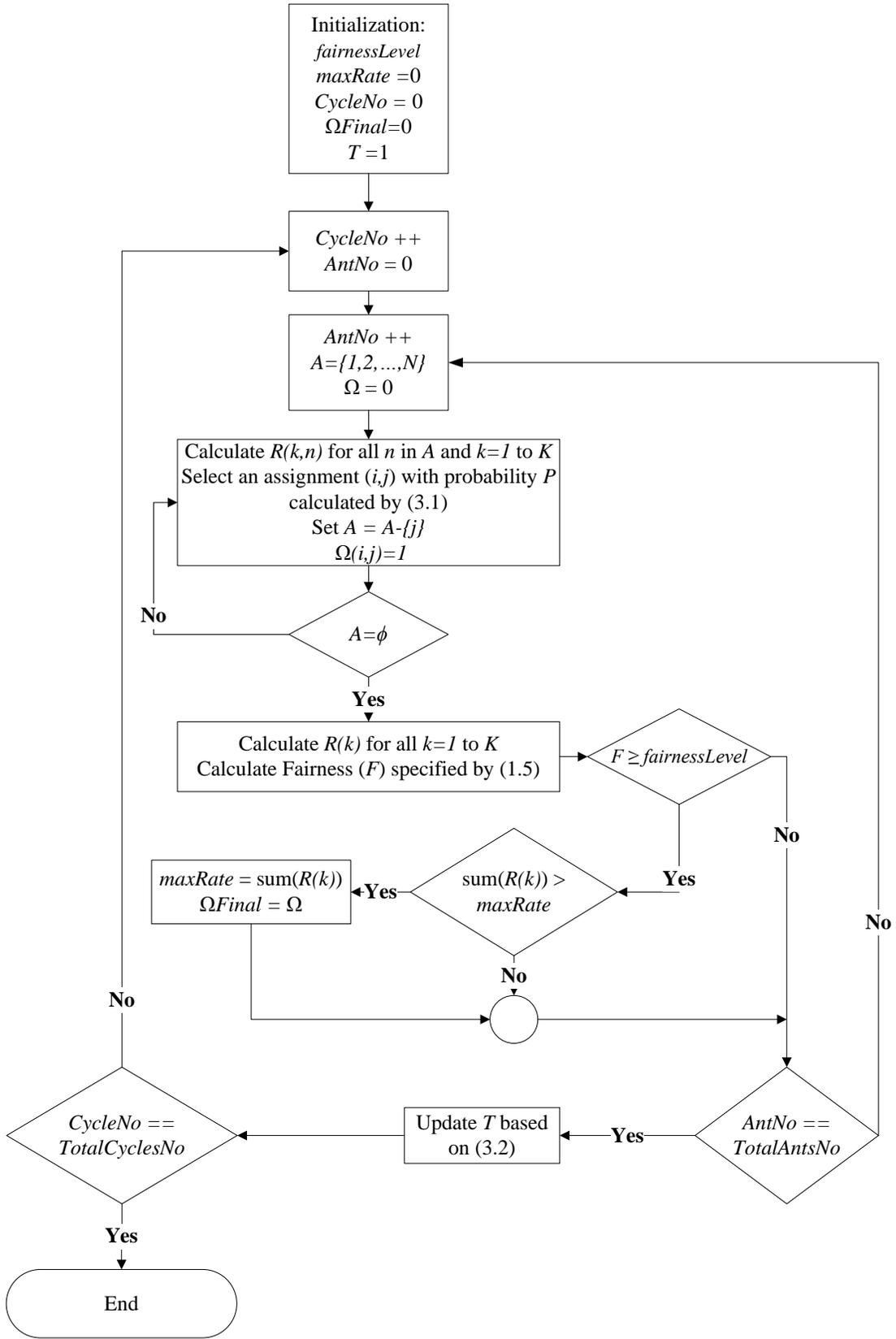
Figure 3.4: Flow Chart of ACO-based Algorithm Implementation
