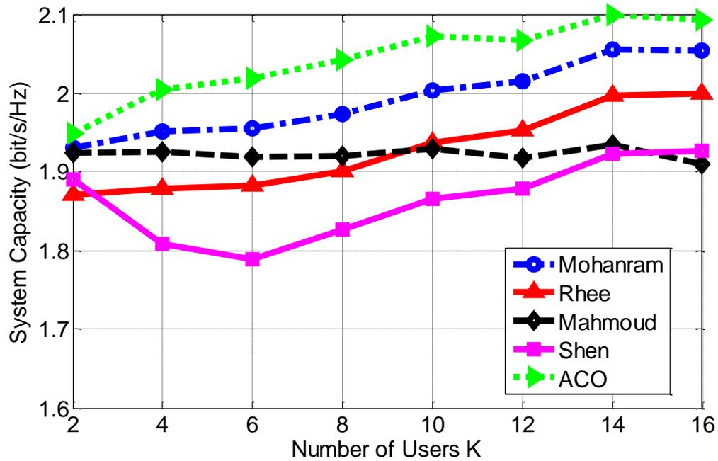
Figure 4.21: Comparison of total system capacity versus number of users for ACO-based algorithm version 3 and other algorithms for  $\gamma_i = 1 \forall (i\%2) = 1$  and  $\gamma_i = 16 \forall (i\%2) = 0$  for  $i = 1, 2, \dots, K$
