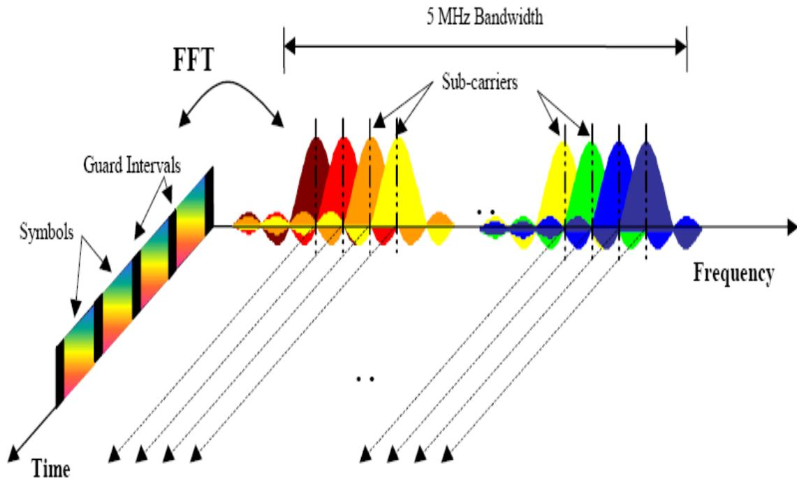
Figure 1.1: OFDM Signal [4]
