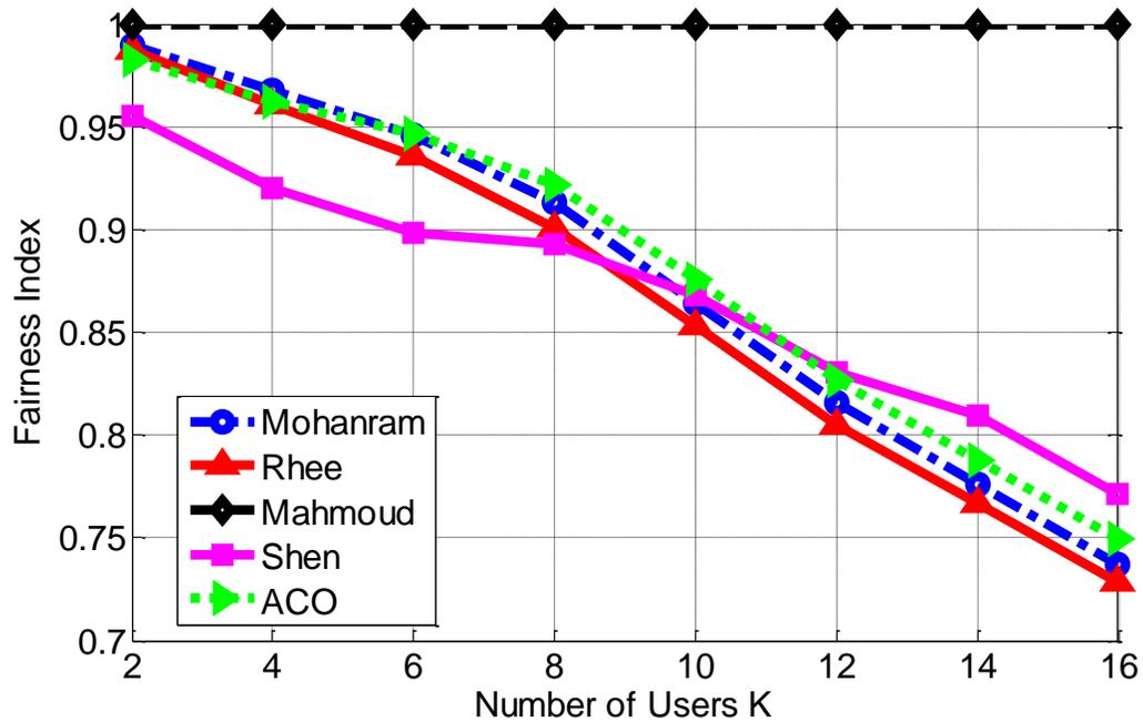
Figure 4.22: Comparison of fairness index versus number of users for ACO-based algorithm version 3 and other algorithms for  $\gamma_i = 1 \forall (i\%2) = 1$  and  $\gamma_i = 16 \forall (i\%2) = 0$  for  $i = 1, 2, \dots, K$
