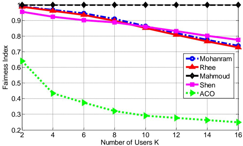
Figure 4.10: Comparison of fairness index versus number of users for ACO-based algorithm version 1 and other algorithms for  $\gamma_i = 1 \forall (i \% 2) = 1$  and  $\gamma_i = 16 \forall (i \% 2) = 0$  for  $i = 1, 2, \dots, K$
