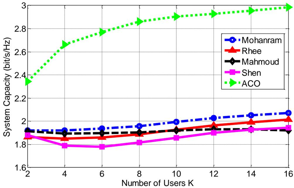
Figure 4.9: Comparison of total system capacity versus number of users for ACO-based algorithm version 1 and other algorithms for  $\gamma_i = 1 \forall (i \% 2) = 1$  and  $\gamma_i = 16 \forall (i \% 2) = 0$  for  $i = 1, 2, \dots, K$
