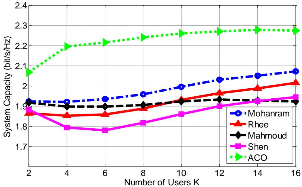
Figure 4.15: Comparison of total system capacity versus number of users for ACO-based algorithm version 2 and other algorithms for  $\gamma_i = 1 \forall (i\%2) = 1$  and  $\gamma_i = 16 \forall (i\%2) = 0$  for  $i = 1, 2, \dots, K$
