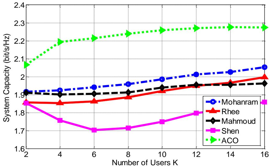
Figure 4.13: Comparison of total system capacity versus number of users for ACO-based algorithm version 2 and other algorithms for  $\gamma_i = 1 \forall (i\%2) = 1$  and  $\gamma_i = 8 \forall (i\%2) = 0$  for  $i = 1, 2, \dots, K$
