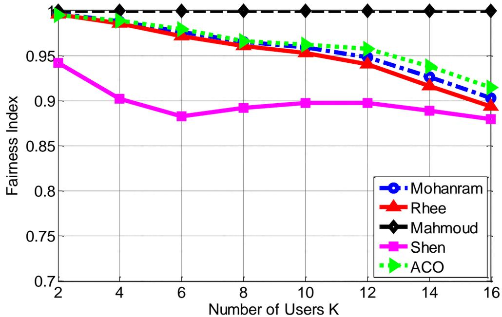
Figure 4.20: Comparison of fairness index versus number of users for ACO-based algorithm version 3 and other algorithms for  $\gamma_i = 1 \forall (i \% 2) = 1$  and  $\gamma_i = 8 \forall (i \% 2) = 0$  for  $i = 1, 2, \dots, K$
