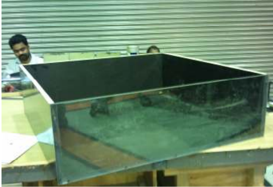
Figure 4.13: Fabricated Formwork for the Study of Flow Profiles During the Casting of the Slab.
