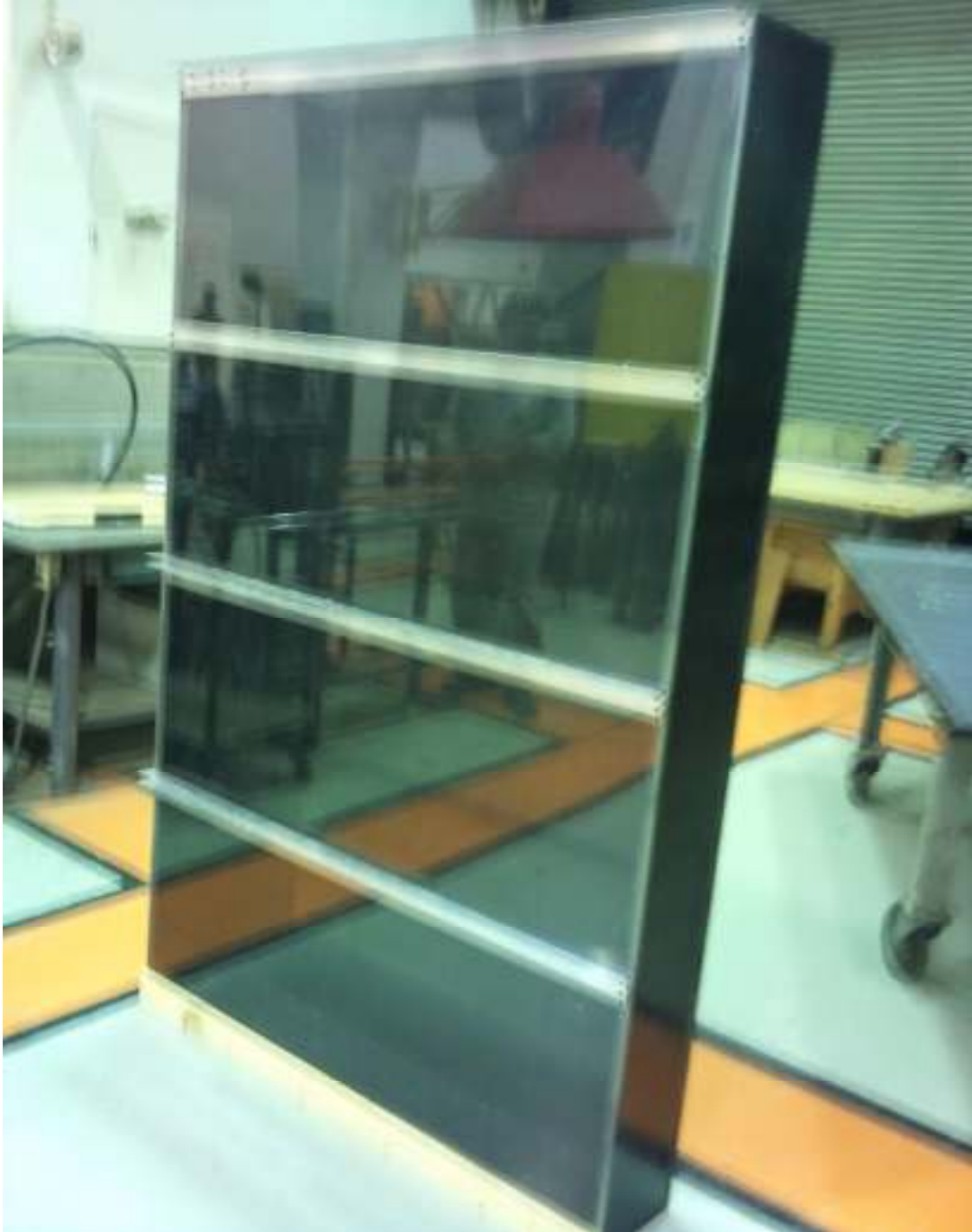
Figure 4.9: A 2mX1.5mX0.2m Fabricated Formwork for the Measurement of Lateral Pressure Exerted by SCC due to Full-Scale Casting of a Wall.
