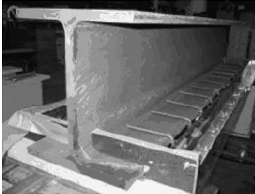
Figure 2.7: 2m Test Semi-Transparent Formwork [Roussel et al., 2007(b)].
