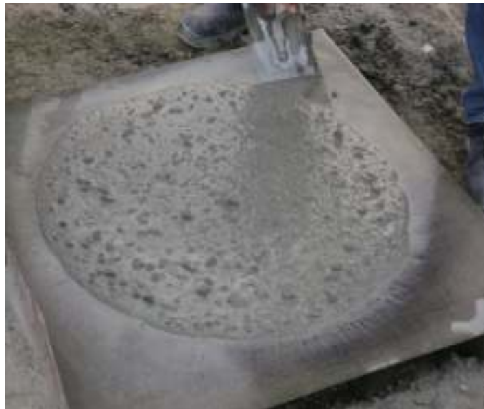
Figure 4.1: Slump Flow and T500 Test.
