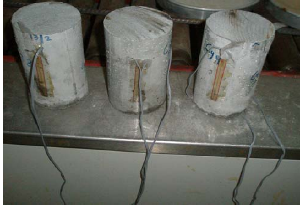
Figure 3.5: Specimens of Ductal with strain gauges for measuring modulus of elasticity.
