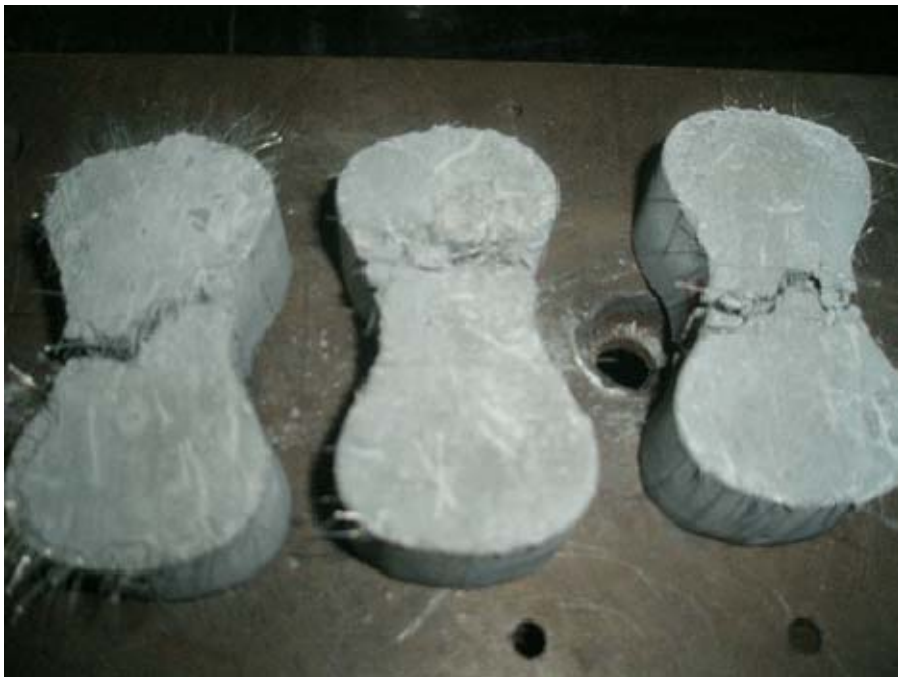
Figure 3.10: Mortar Briquette specimens of Ductal after testing.
