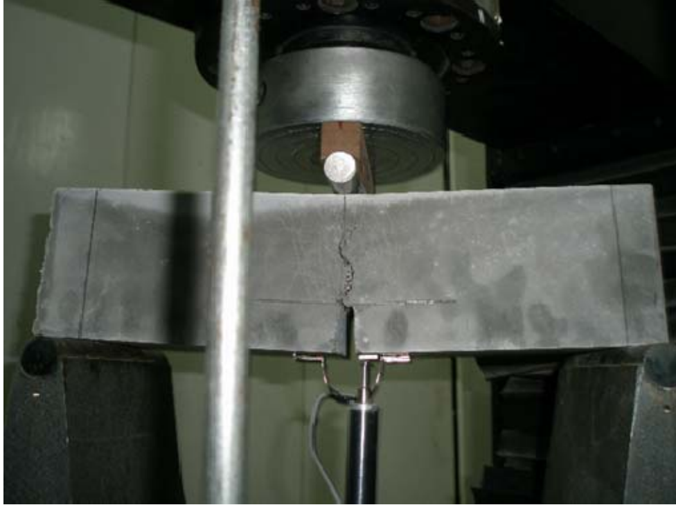
Figure 3.20: Close-up view of fracture toughness test.
