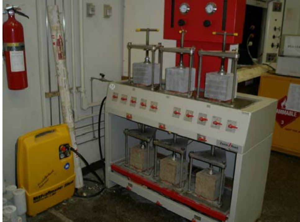
Figure 3.14: Water penetration test setup.
