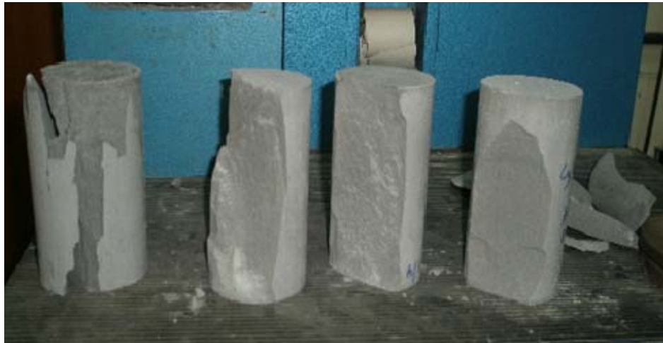
Figure 4.2: Failure mode of Ductal without fiber (0% fibers).
