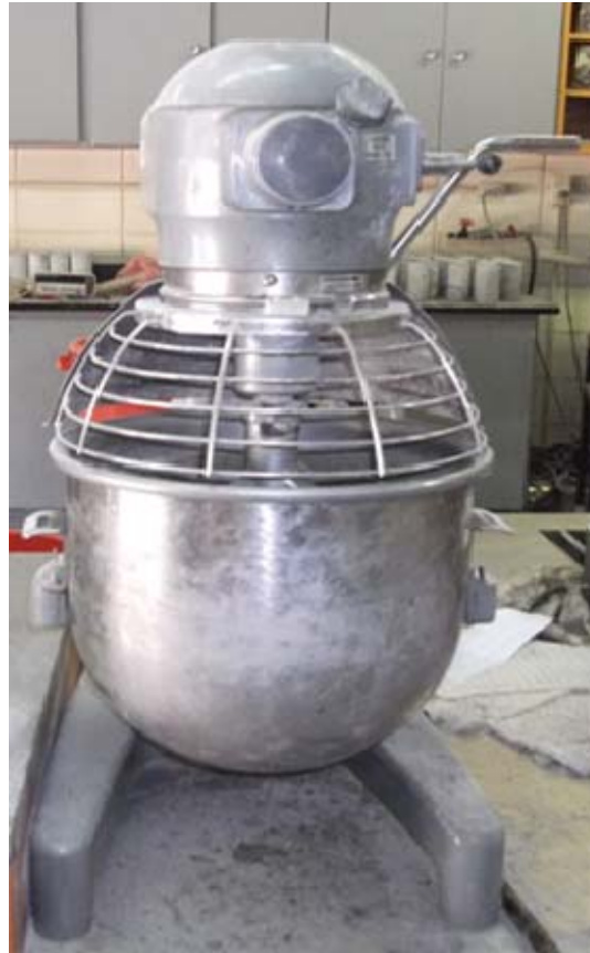
Figure 3.1: HOBART planetary mixer.
