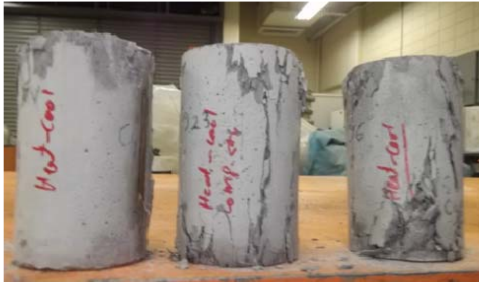
Figure 4.3: Failure mode of Ductal (6.2% fibers).
