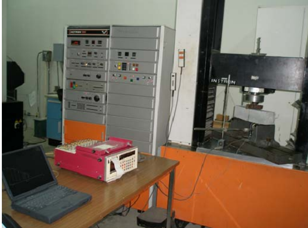
Figure 3.18: Complete test setup for measuring fracture toughness of Ductal prisms.
