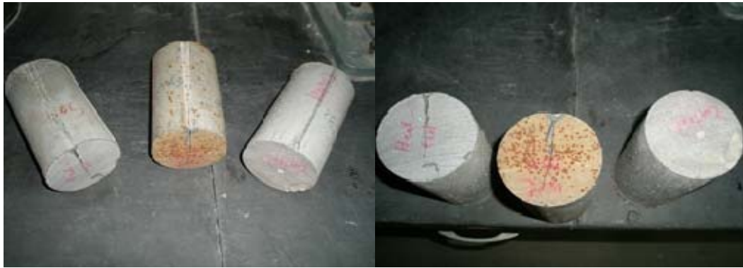
Figure 4.27: Mode of failure after splitting tensile test.
