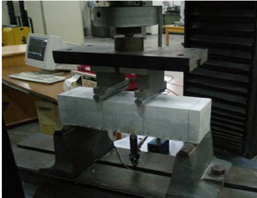
Figure 3.7: Flexural strength test using four-point bending.
