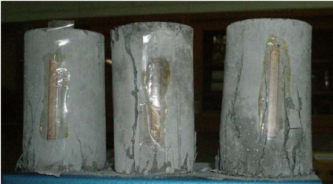
Figure 3.4: Ductal cylinders after failure under compression test.
