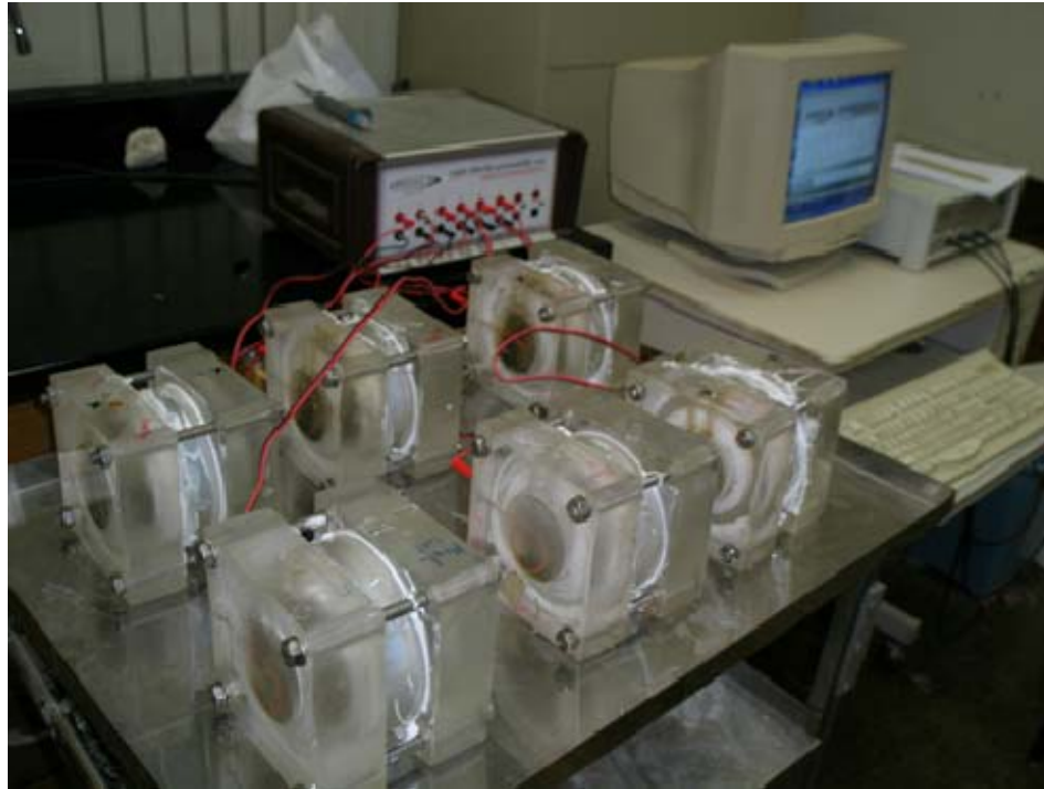
Figure 3.15: Experimental setup to determine the rapid chloride ion penetrability.
