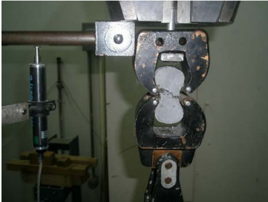
Figure 3.11: Mortar briquette setup including test grips and specimen.
