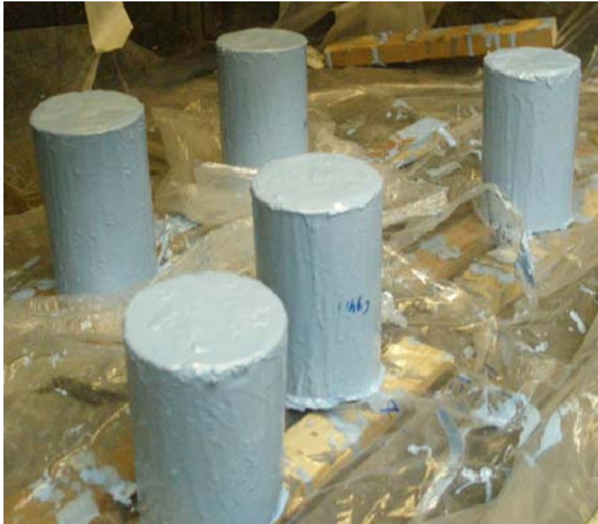
Figure 3.16: Coated specimens utilized for chloride diffusion test.
