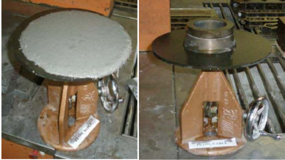
Figure 3.3: Impact table measurement of Ductal flow.
