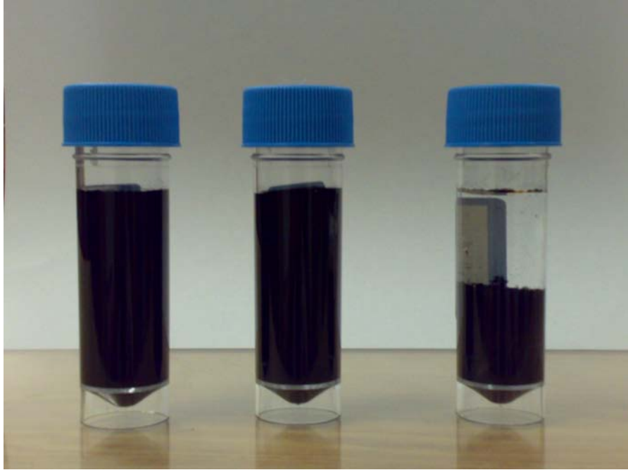
Figure 4.15 Photographs of oxidized MWCNT and MWCNT-PEG nanofluid show no precipitation after two months
