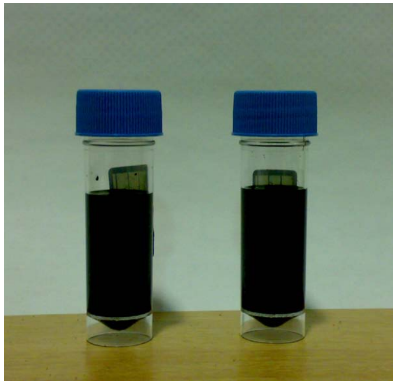
Figure 4.16 Photographs of impregnated MWCNT nanofluid show no precipitation in presence of SDS surfactant after two months
