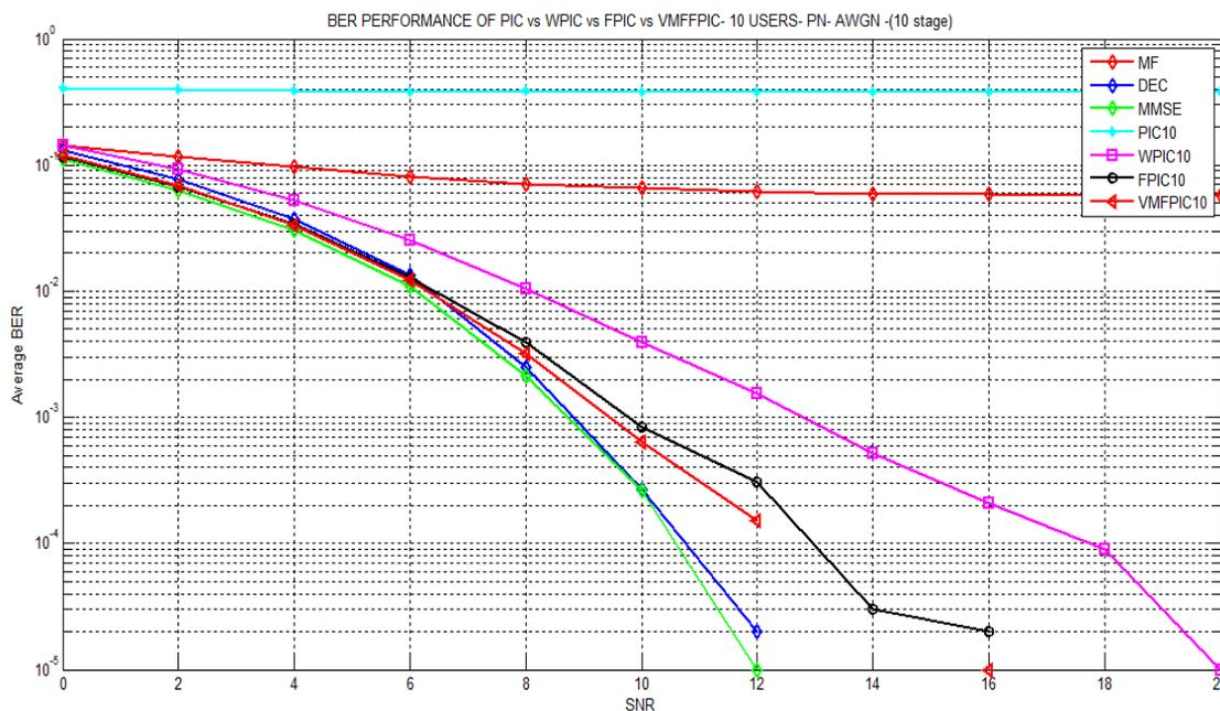
Figure 5-5 BER Performance of Fuzzy PIC using PN Codes- 10 equal power users
