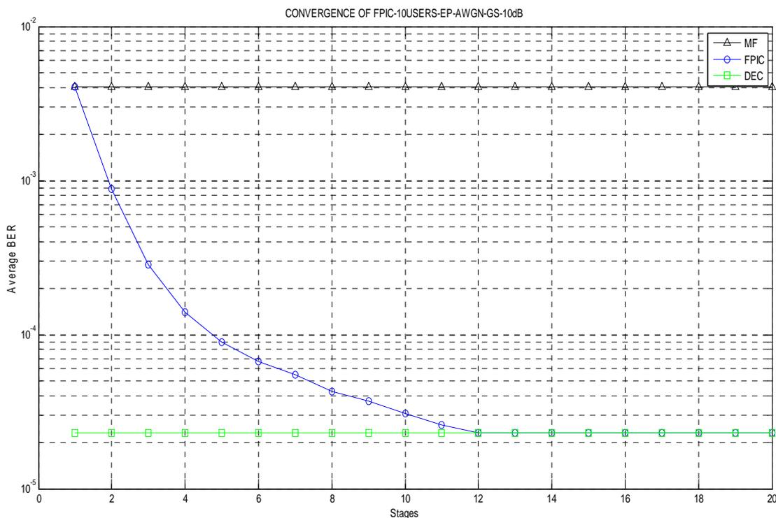
Figure 5-9 Convergence of Fuzzy PIC using Gold Codes- 10 equal power users
