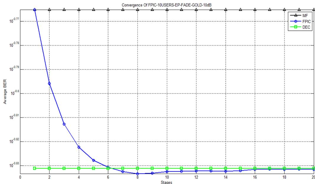
Figure 5-11 Convergence of Fuzzy PIC using Gold Codes- 10 equal power users under Rayleigh flat fading Channel
