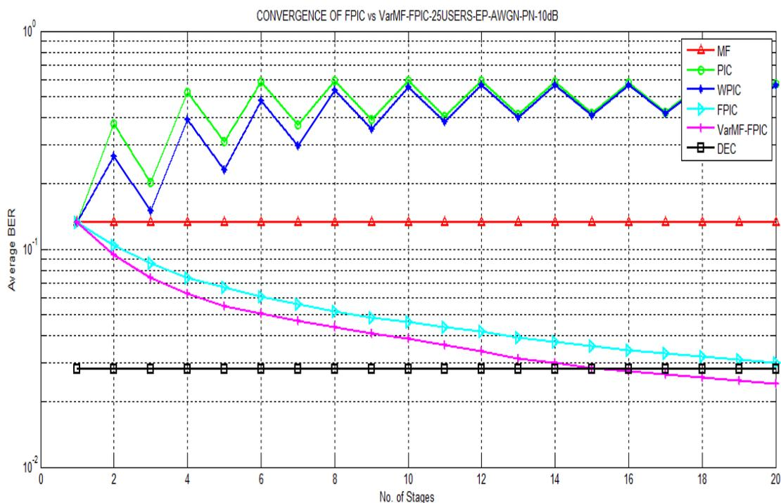
Figure 5-7 Convergence of Fuzzy PIC using PN Codes- 25 equal power users
