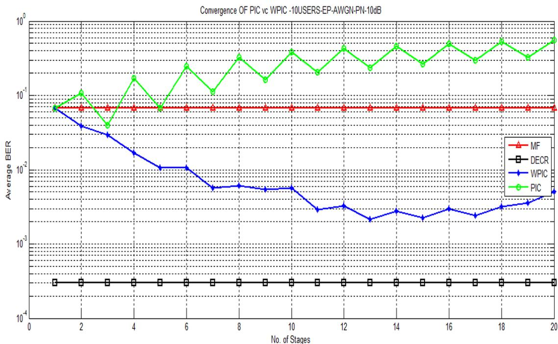
Figure 3-8 Convergence of Weighted PIC using PN Codes – 10 equal power users
