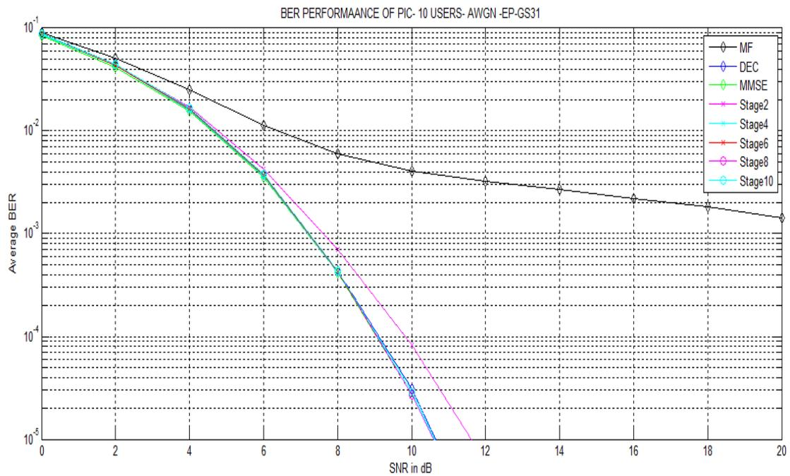
Figure 3-3 BER Performance of PIC using Gold Codes- 10 equal power users
