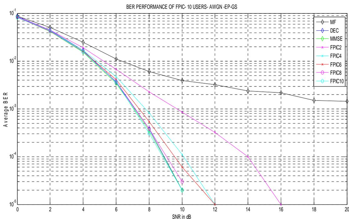
Figure 5-8 BER Performance of Fuzzy PIC using Gold Codes- 10 equal power users
