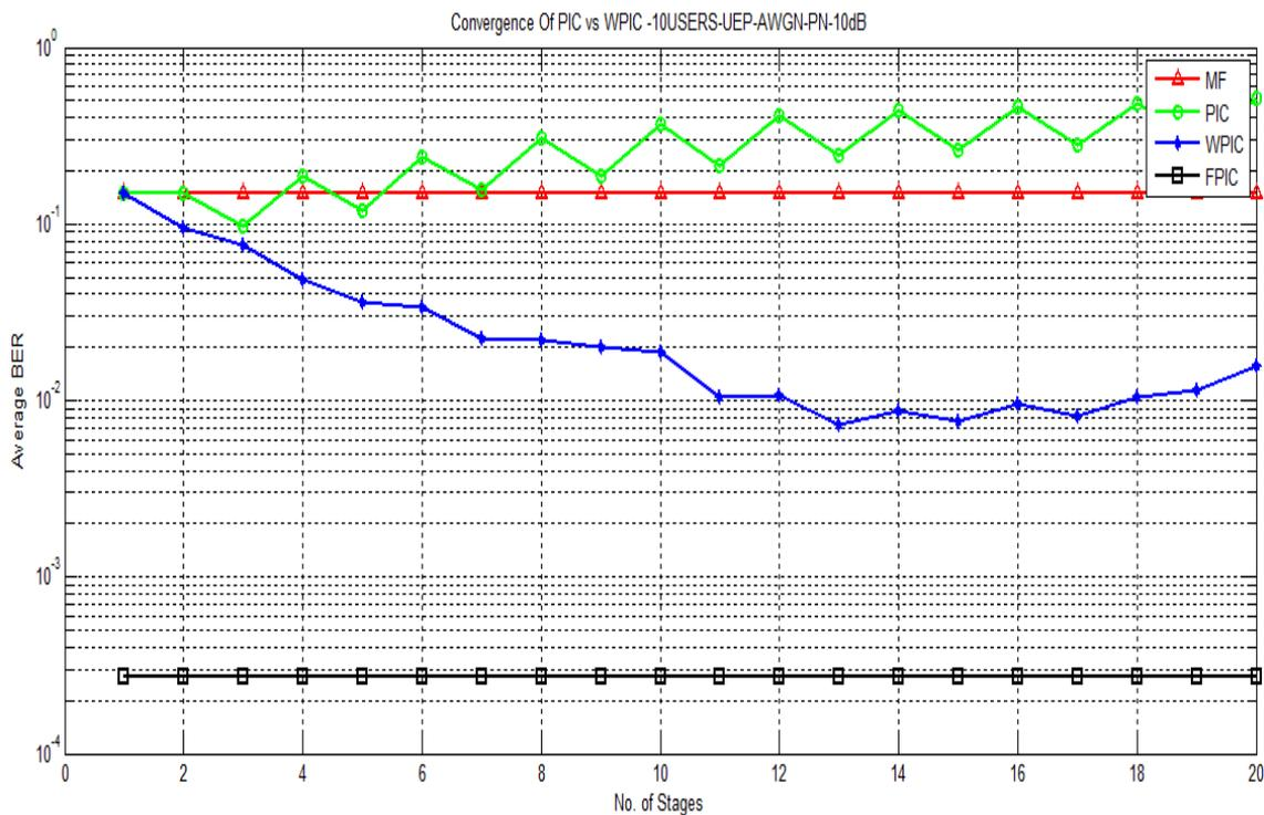
Figure 3-10 Convergence of Weighted PIC using PN Codes – 10 unequal power users
