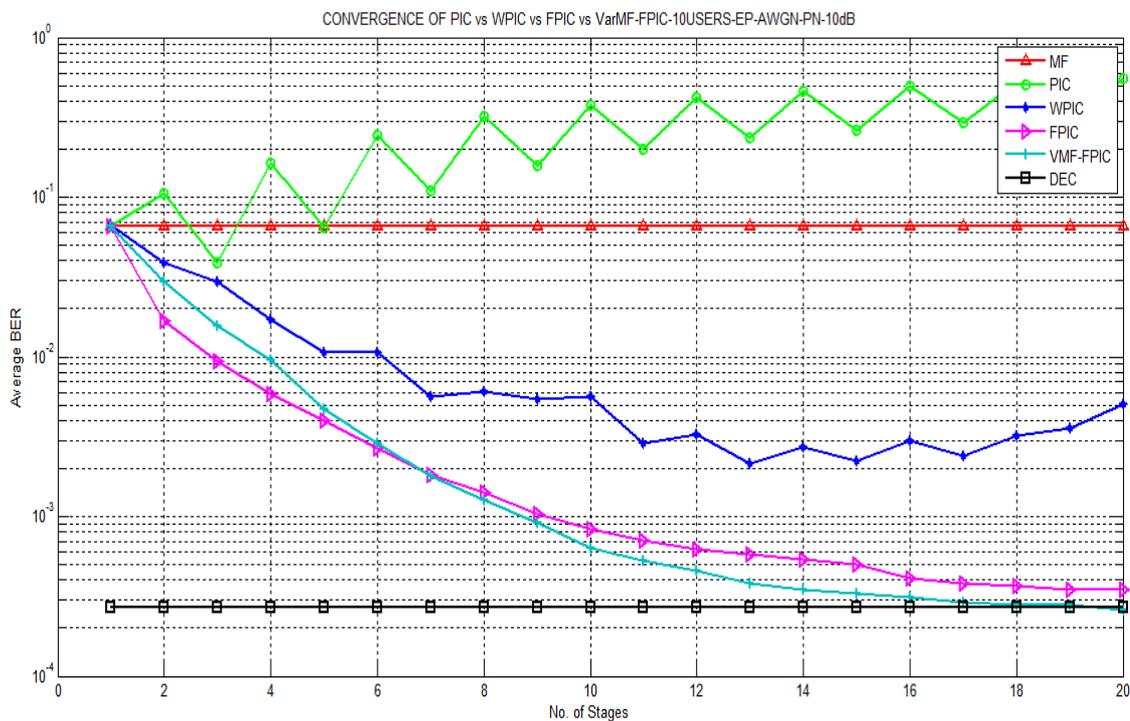
Figure 5-6 Convergence of Fuzzy PIC using PN Codes- 10 equal power users
