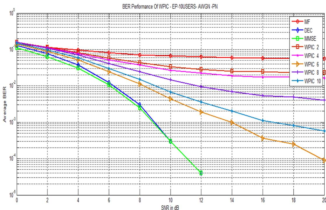
Figure 3-7 BER Performance of Weighted PIC using PN Codes – 10 equal power users
