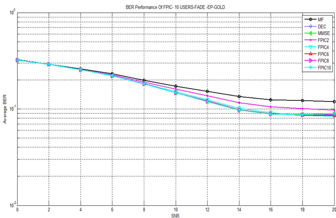
Figure 5-10 BER Performance of Fuzzy PIC using Gold Codes- 10 equal power users under Rayleigh flat fading Channel
