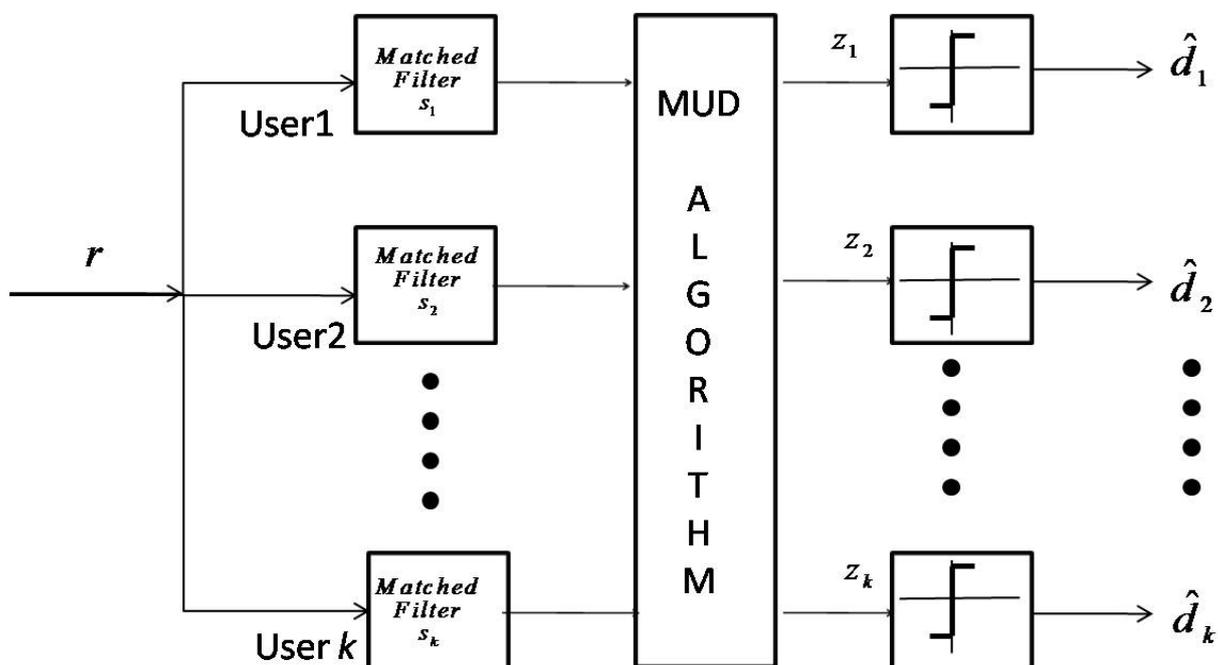
Figure 2-4 General Concept of Multiuser Detection
