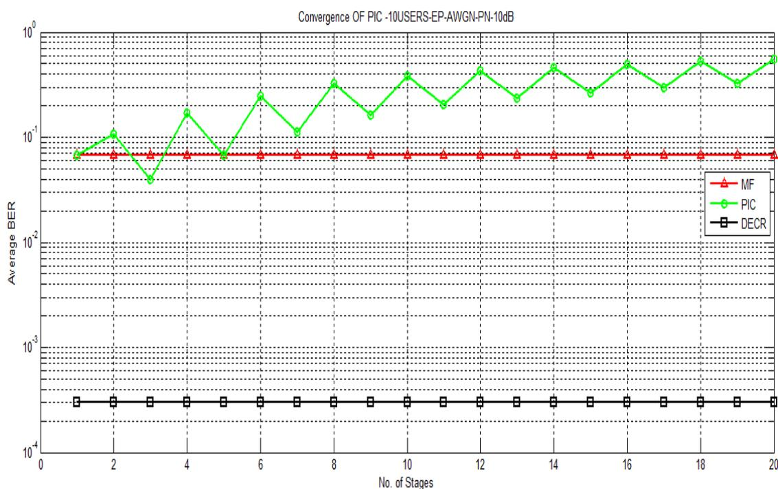
Figure 3-6 Convergence of PIC using PN Codes – 10 equal power users
