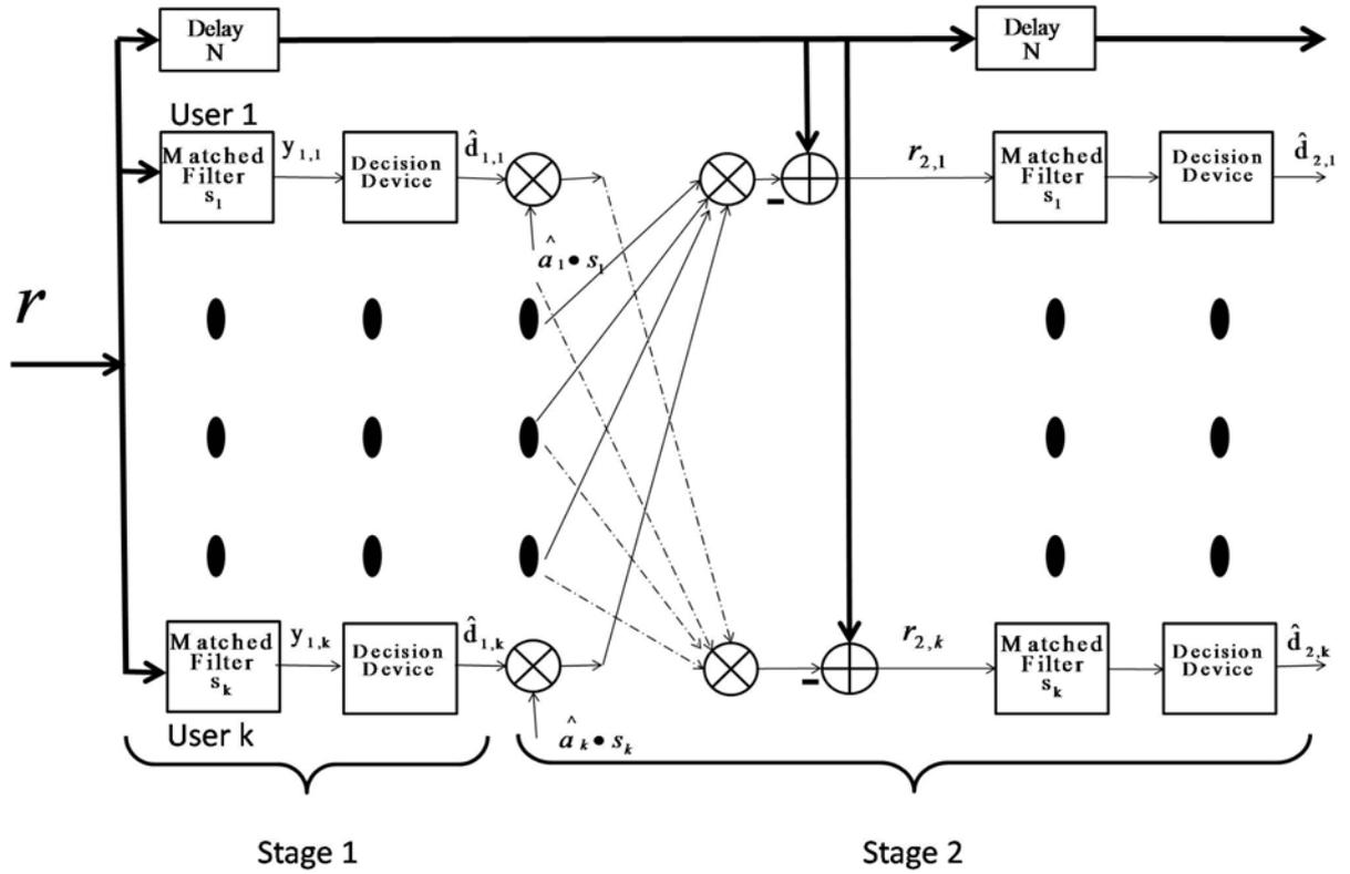
Figure 3-1 Multistage Parallel Interference Cancellation
