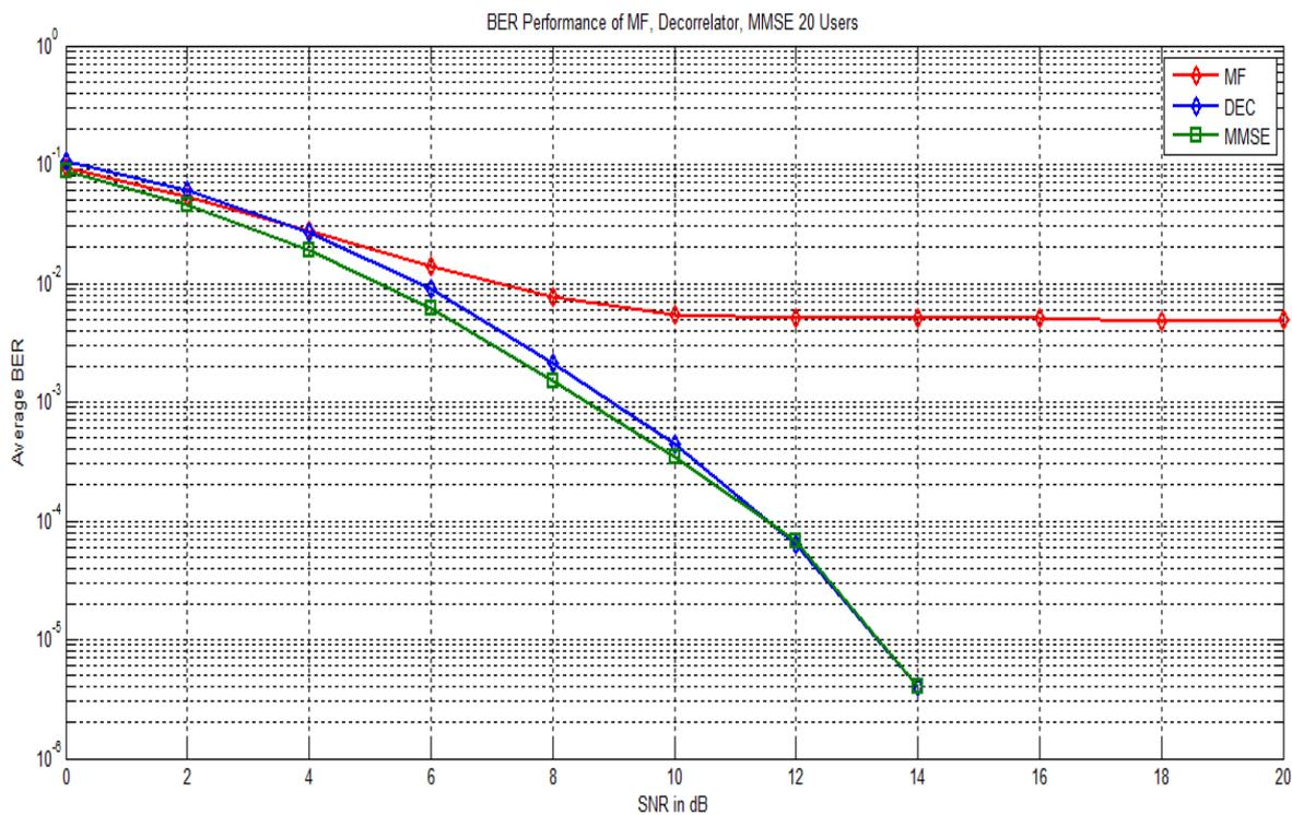
Figure 2-9 BER Performance of MMSE Detector
