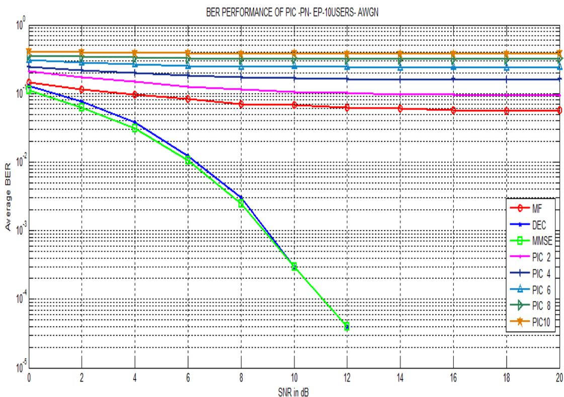
Figure 3-5 BER Performance of PIC using PN Codes – 10 equal power users
