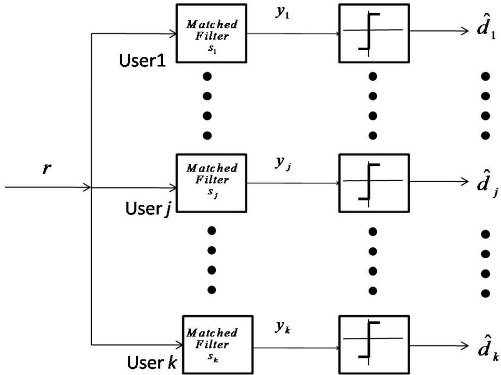
Figure 2-2 Conventional Matched Filter Receiver
