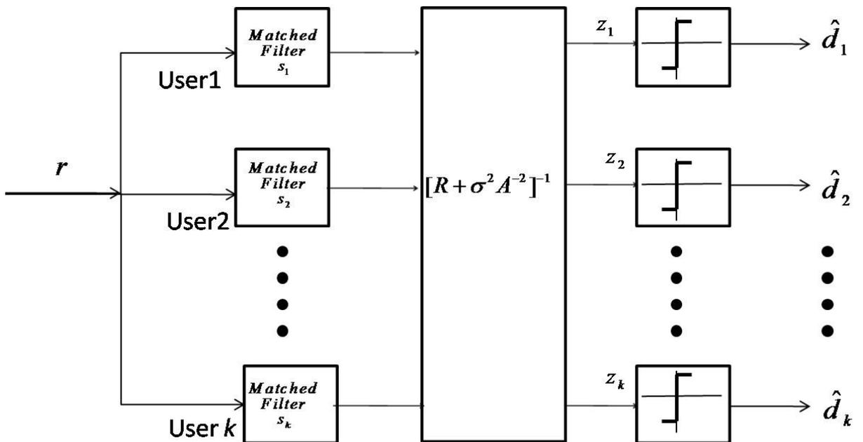
Figure 2-8 MMSE Detector
