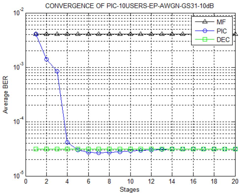
Figure 3-4 Convergence of PIC using Gold Codes – 10 equal power users
