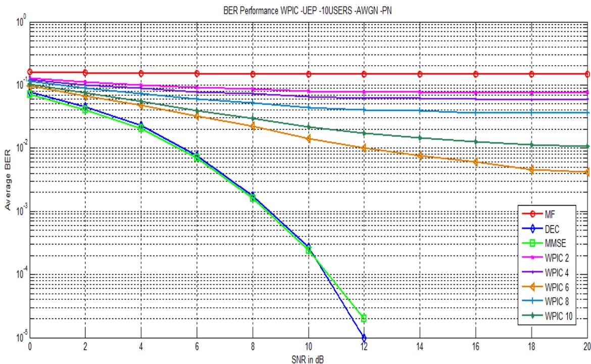
Figure 3-9 BER Performance of Weighted PIC using PN Codes – 10 unequal power users
