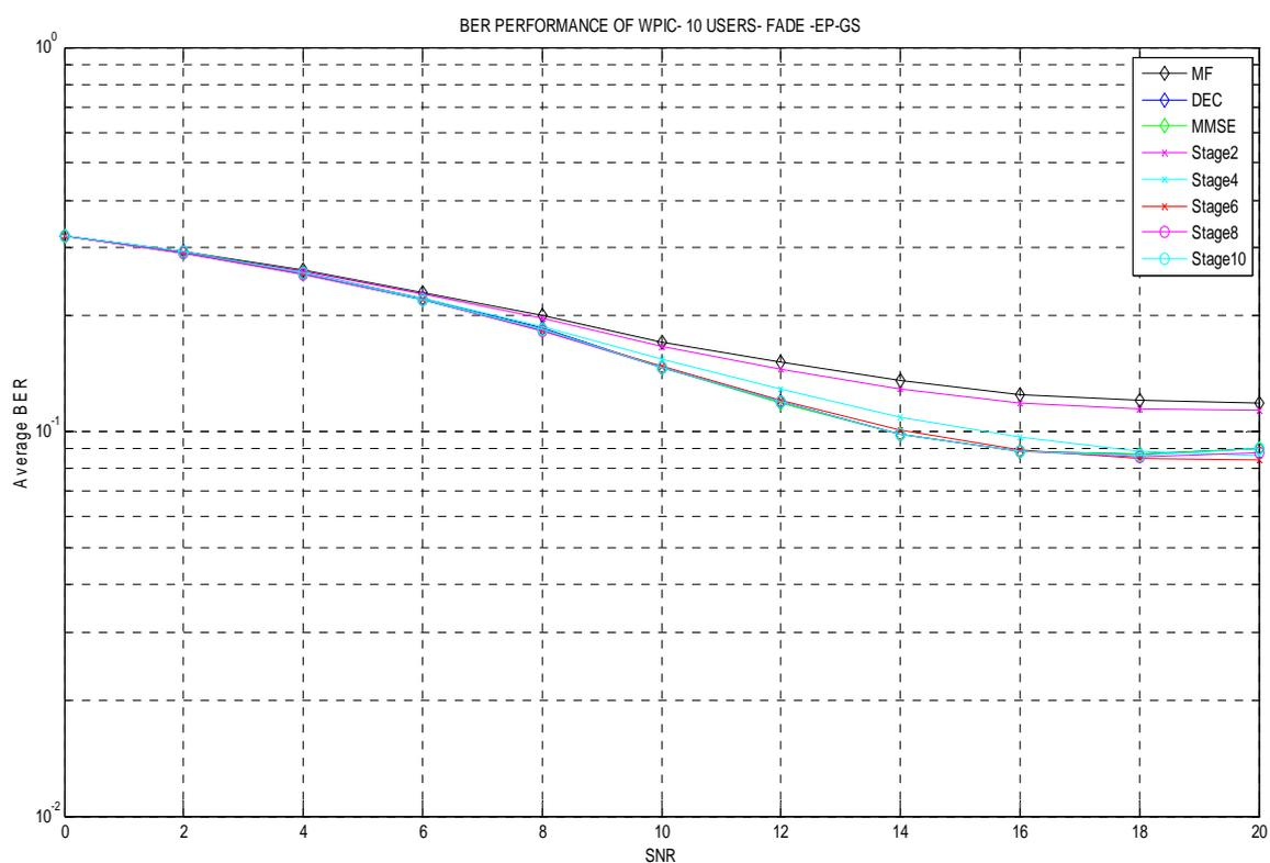
Figure 3-11 BER Performance of Weighted PIC using Gold Codes – 10 equal power users under fading channel
