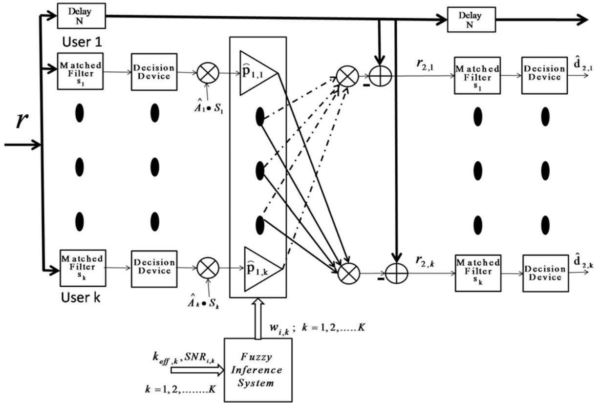
Figure 5-1 Proposed Fuzzy based Weighted PIC detector
