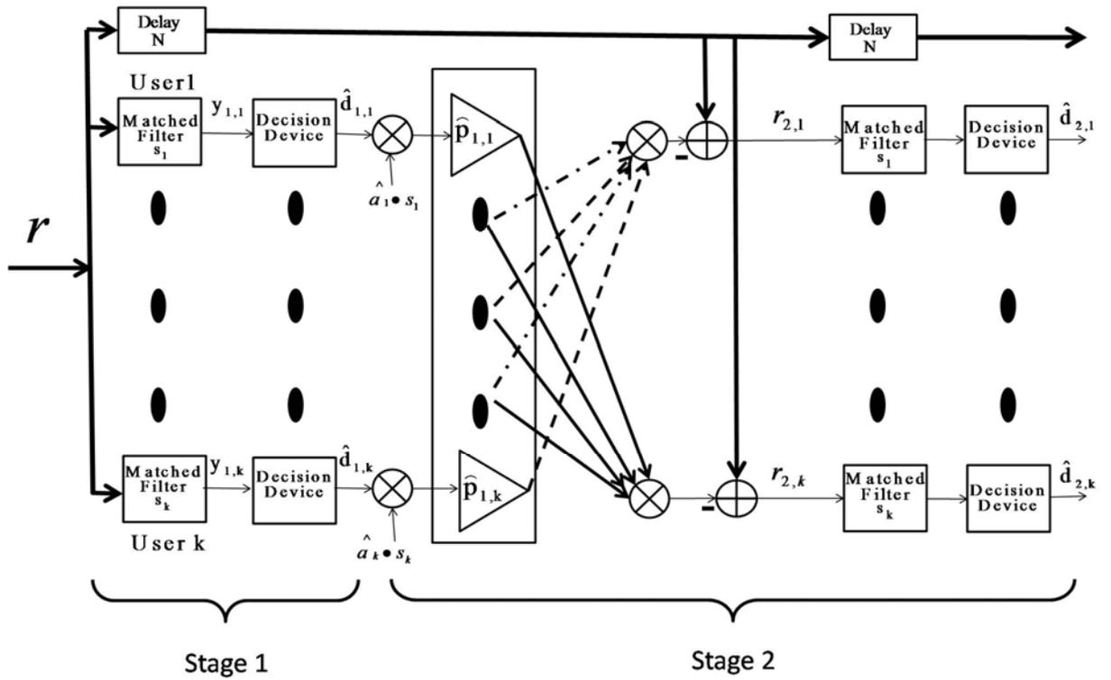
Figure 3-2 Weighted Parallel Interference Cancellation
