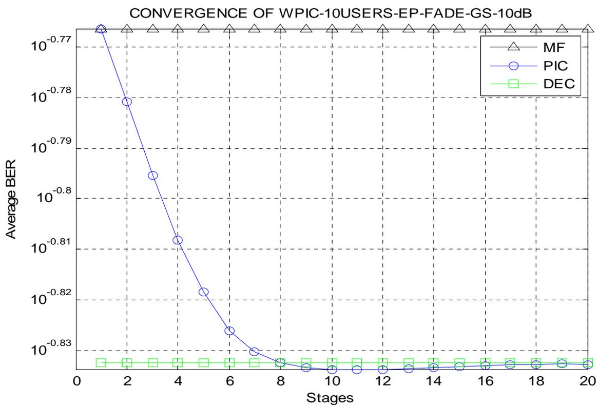
Figure 3-12 Convergence of Weighted PIC using Gold Codes – 10 equal power users under fading channel
