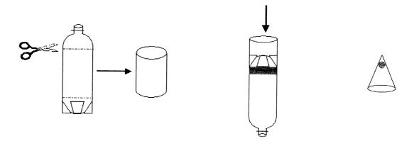
Then make a nose cone that slides easily on and off of the sleeve. Put some modeling clay in the top of the nose cone so that it will cause the rocket to flip over when the rocket starts to descend, and the weight also helps the nose cone falls off. Remember to use some string to attach the nose cone to the rocket body.
