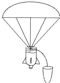
Use a soda bottle with the top and bottom cut off to make a sleeve to hold the parachute.
