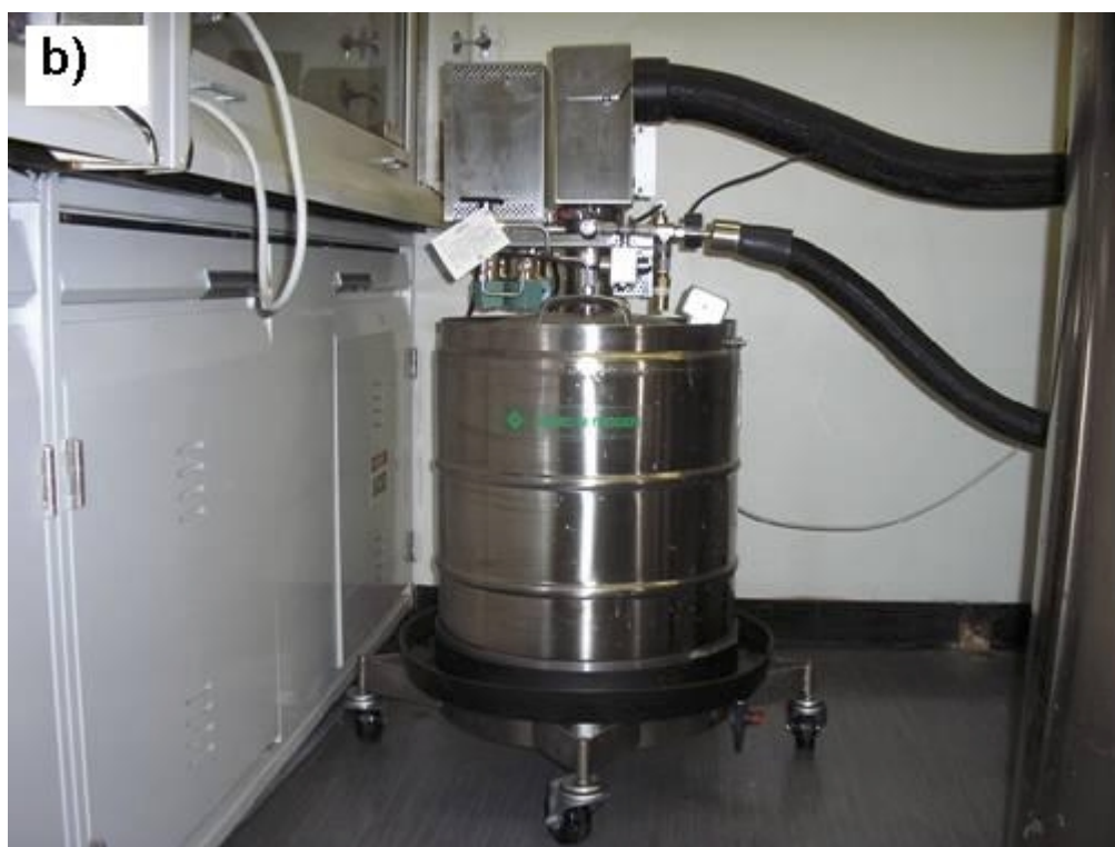
Figure 3.3: a) Modulated DSC Q1000, TA Instrument Inc. equipped with Auto sampler b) Liquid Nitrogen Cooling System (LNCS).
