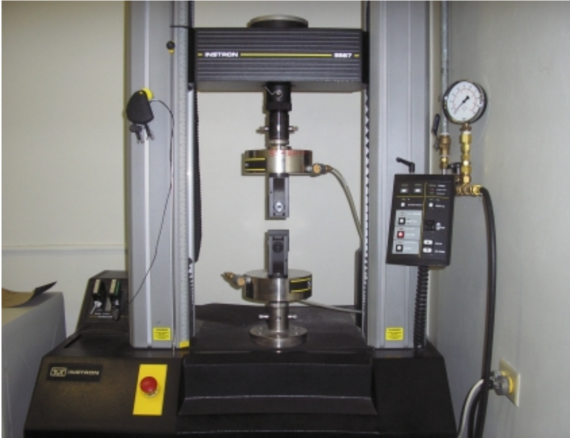
Figure 3.2: Instron 5567 equipped with Pneumatic side action grips.
