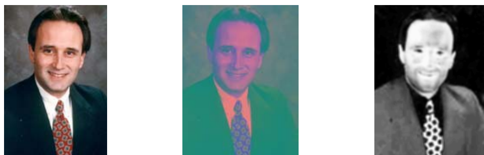
Figure 2.3: The original RGB image, the image transformed to chromatic color space and the skin likelihood image
