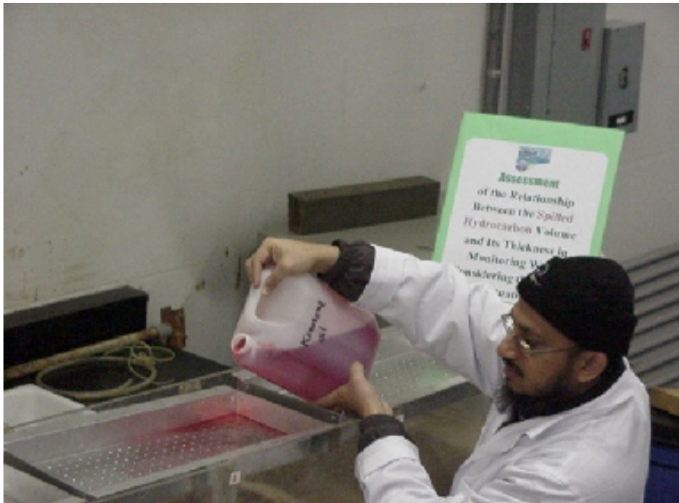
Plate 5.1 Initial hydrocarbon spill in the porous media.
