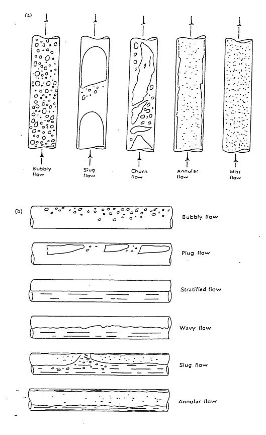
Figure 2.1 Typical two-phase flow patterns: (a) flow patterns in vertical flow (b) flow patterns in horizontal flow (after Tong & Tang<sup>18</sup>)
