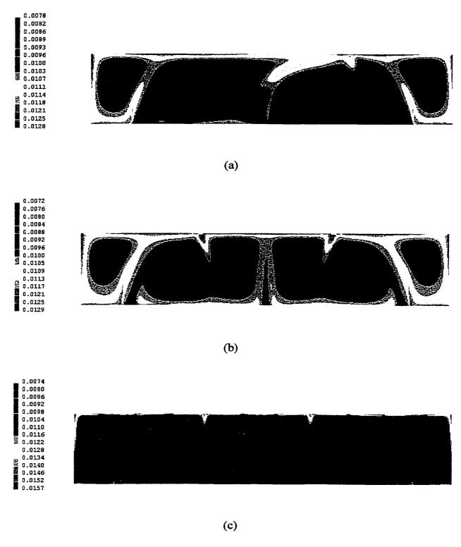
Figure 5.8. Contours of the liquid volume fraction (R2) at 57 m/s for (a) one outlet, (b) two-outlets, and (c) multiple outlets
