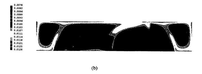
Figure 5.4. (a) Gas volume fraction (R1) and (b) Liquid volume fraction (R2) for an injection velocity of 57 m/s.
