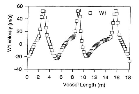
Figure 4.4. A plot of the (a) V1 velocity across the vessel at slab 25, and (b) W1 velocity across the vessel length at slab 25
