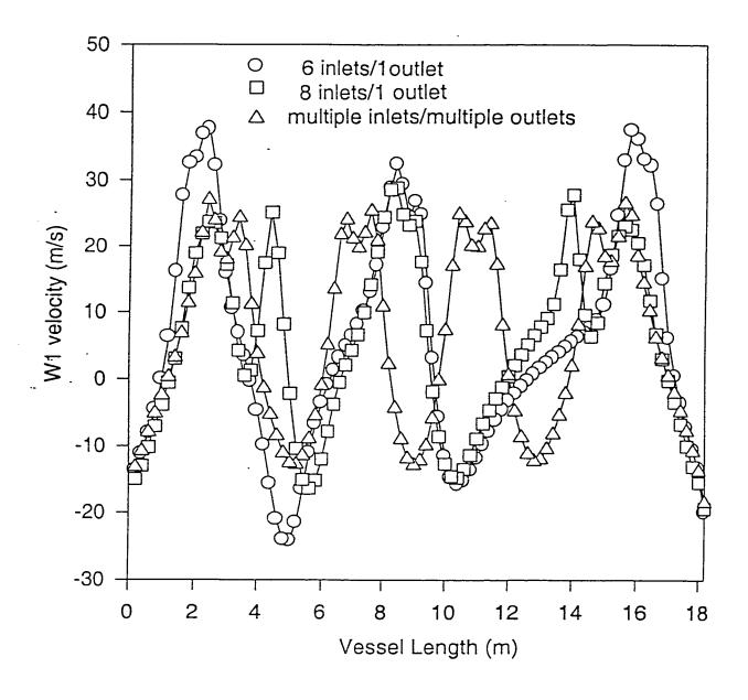
Figure 4.11 (b) A plot of W1 versus the vessel length for slab 25 for three different inlet/outlet arrangements.
