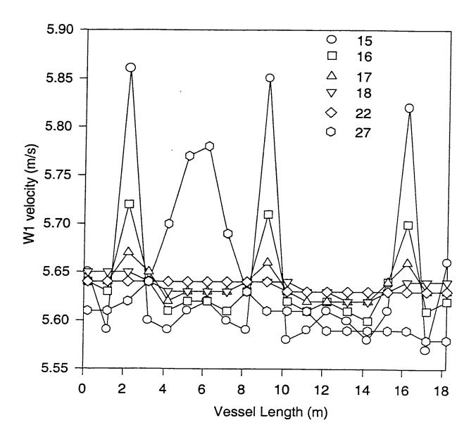
Figure 6.7. A plot of velocity in the z-direction for the packed bed with  $F_z = 5000$  and  $F_y = 5000$  at various positions in the bed
