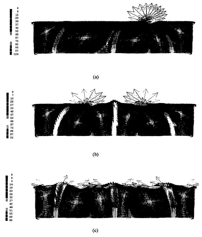
Figure 4.7. Velocity Field for an injection velocity of 57 m/s, three inlets and (a) one outlet, (b) two outlets and (c) multiple outlets
