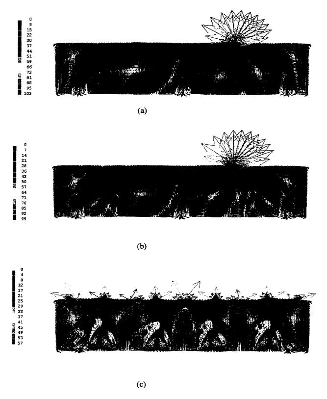
Figure 4.10. (a) Velocity Field for 6 cell inlet, (b) Velocity Field for 8 cell inlet, and (c) Velocity Field for a multiple inlet/ multiple outlet
