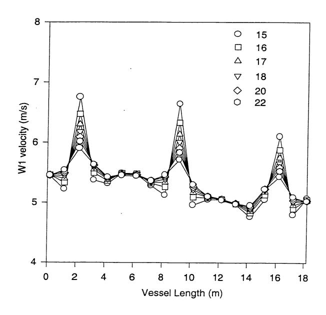
Figure 6.3 (b). A plot of W1 versus the vessel length at various positions in the packed bed
