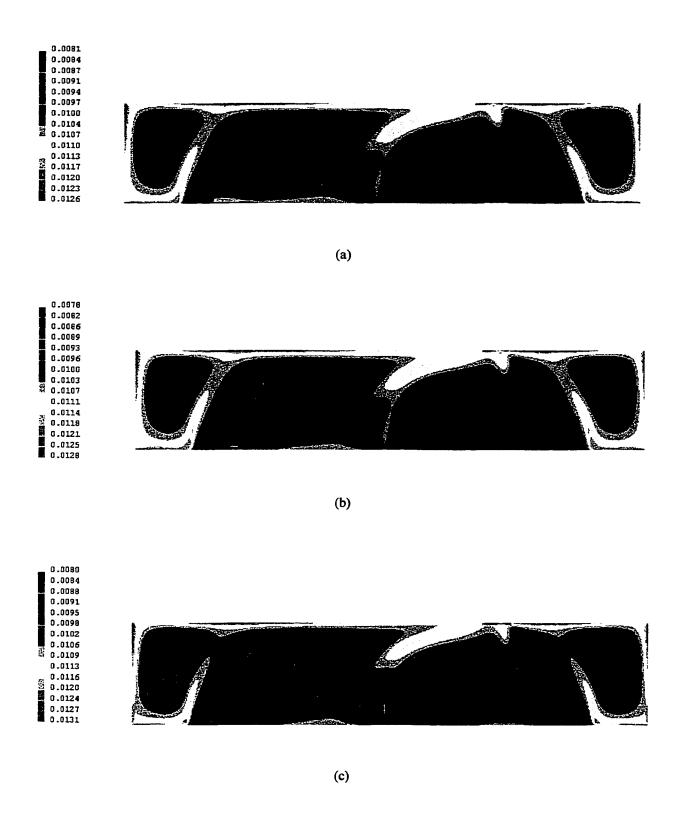
Figure 5.6. (a) Contours of the Liquid volume fraction (R2) at an injection velocity of (a) 45 m/s, (b) 57 m/s and (c) 70 m/s.
