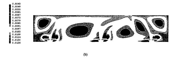
Figure 5.12. Annular disc 1.6 m OD and 0.4 m ID. (a) Velocity Field and (b) Contour of the Liquid volume fraction (R2)
