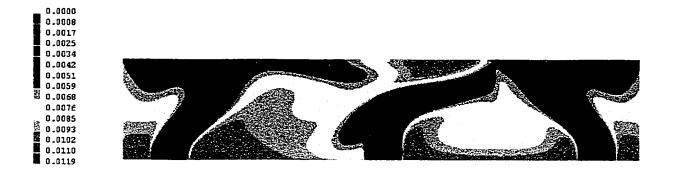
Figure 5.9 Six inlets (a) Velocity Field, and (b) Contour of R2
