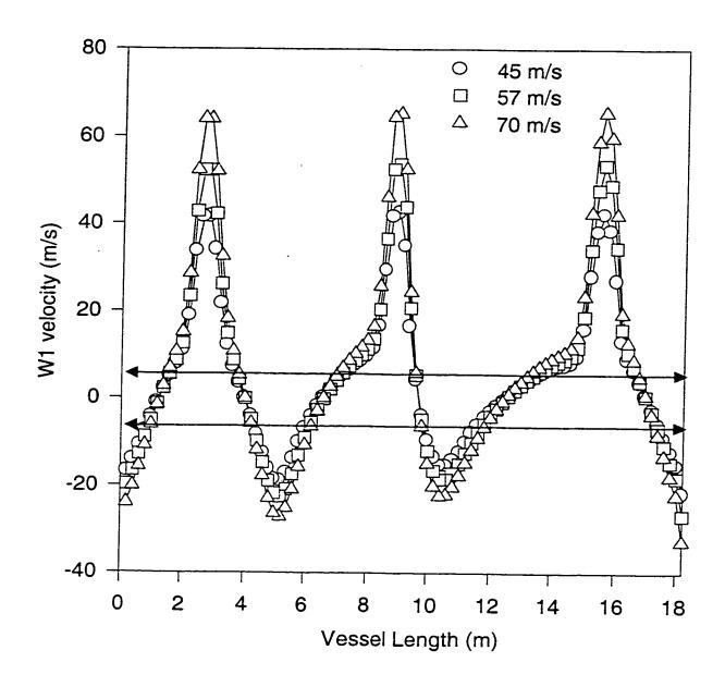
Figure 4.6. (b) A plot of W1 versus the vessel length for slab 25 at three different injection velocities
