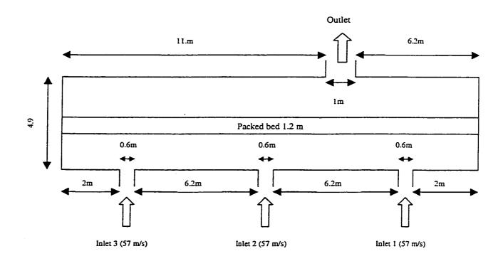
Figure 6.1. Schematic of the Packed Bed
