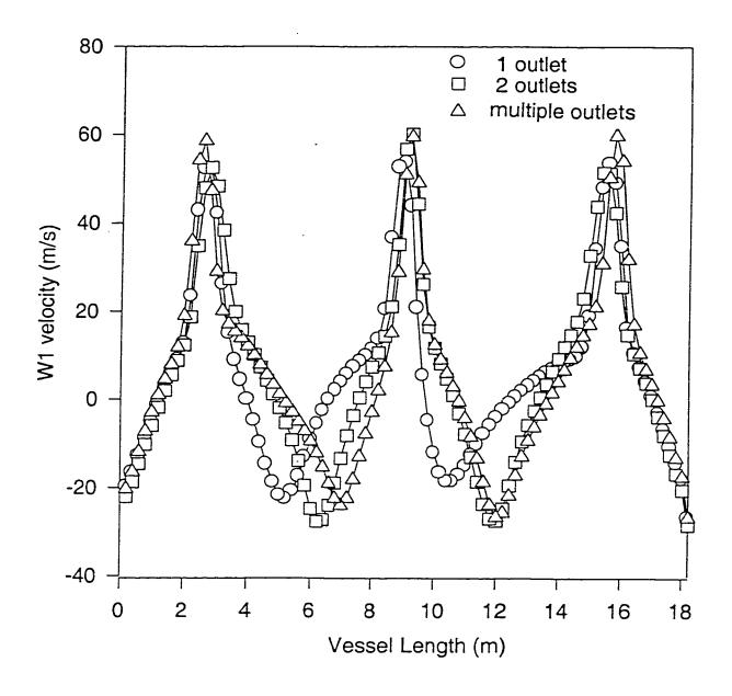
Figure 4.9 (b). A plot of W1 versus the vessel length for slab 25 at three different outlet arrangements.
