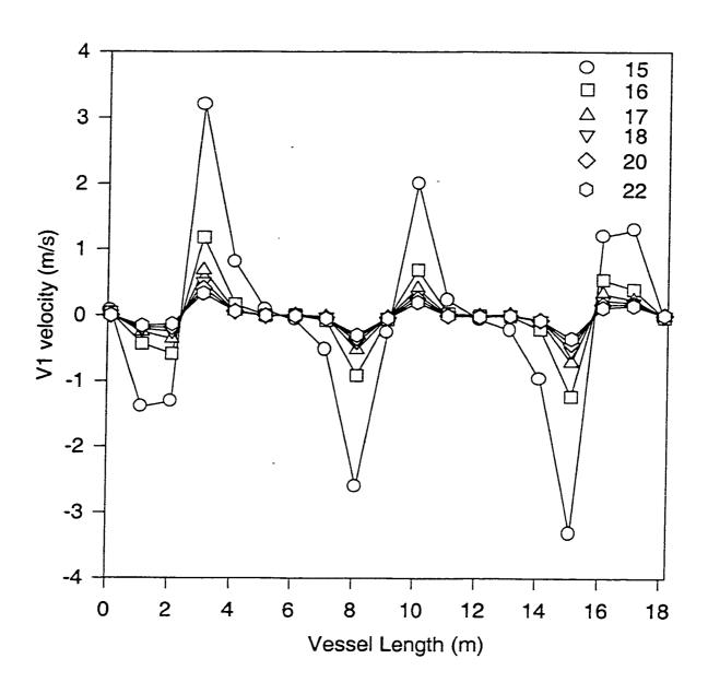
Figure 6.3 (a). A plot of V1 versus the vessel length at various positions in the packed bed
