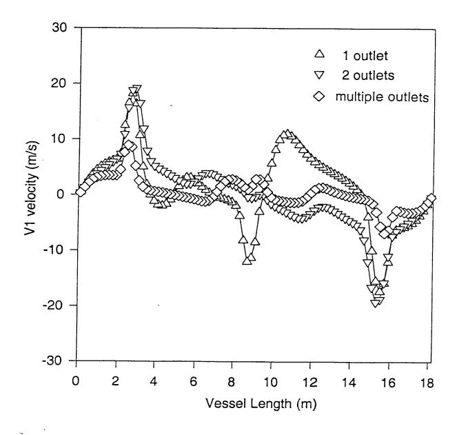
Figure 4.9 (a) A plot of V1 versus the vessel length for slab 25 for three different outlet arrangements.
