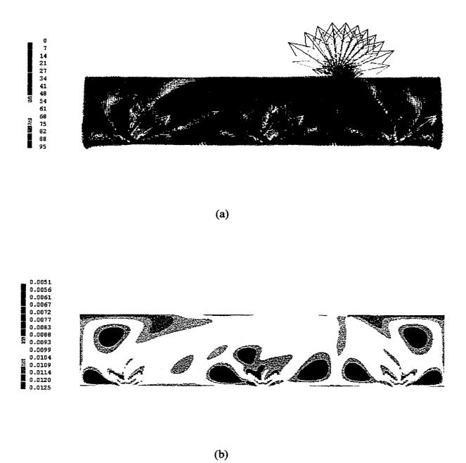
Figure 5.14. Conical Insert. (a) Velocity Field and (b) Liquid volume fraction (R2)
