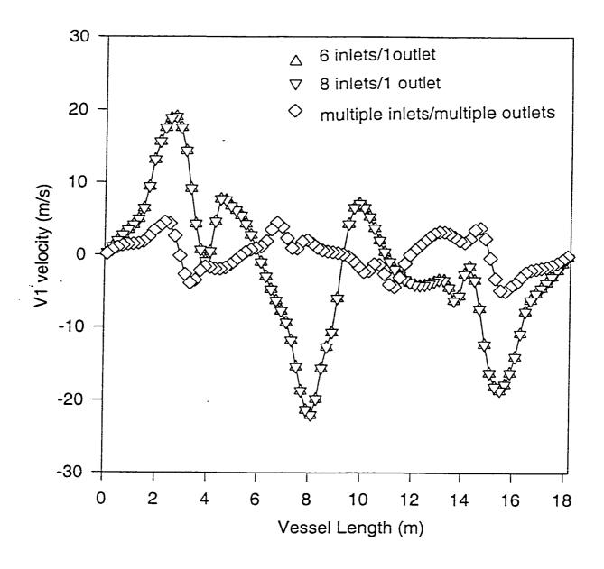
Figure 4.11 (a) A plot of V1 versus the vessel length for slab 25 for three different inlet/outlet arrangements.
