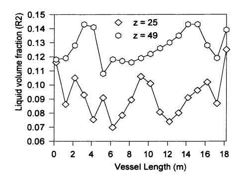
Figure 5.17. Comparison of R2 for the case with gas density =  $20 \text{ kg/m}^3$  and liquid density =  $600 \text{ kg/m}^3$ , with Gas to Liquid split (99:01)
