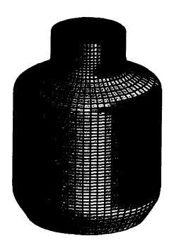
Figure 4.39: A NURBS Surface with 19 X 19 mesh of Control Points.
