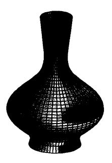
Figure 4.36: Decomposed NURBS Surface with 17 X 17 mesh of Control Points.
