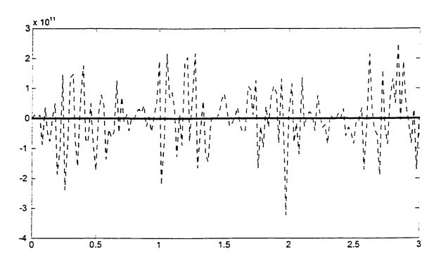
Figure 2.21: Response of the classical heat model in the case of noisy data with SNR=20 dB,  $N=4,\,m=4,\,T=2.$
