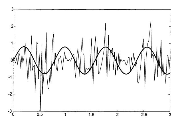
Figure 2.16: Response of the damped model in the case of noisy data with SNR=20 dB.  $N=8, T=1, m=8, \delta=0.065.$
