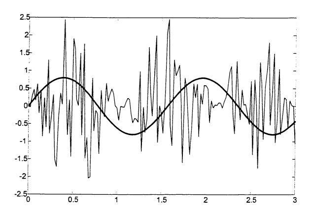
Figure 2.14: Response of the damped model in the case of noisy data with SNR=20 dB,  $N=4, T=1, m=4, \delta=0.067$ .
