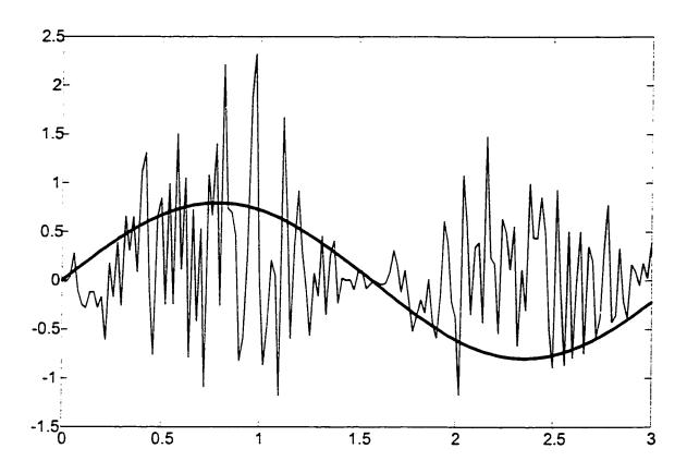
Figure 2.18: Response of the damped model in the case of noisy data with SNR=20 dB,  $N=3, m=2, T=2, \delta=0.14$ .
