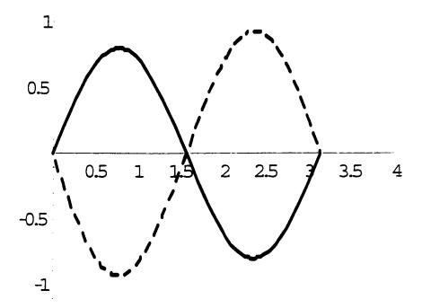
Figure 2.3: Response of the undamped model to the damped data in the case. m=2 and  $\delta=5$  with  $4m^2<\delta^2$ . The thick solid line represents the exact initial profile while the dashed line represents the recovered profile.
