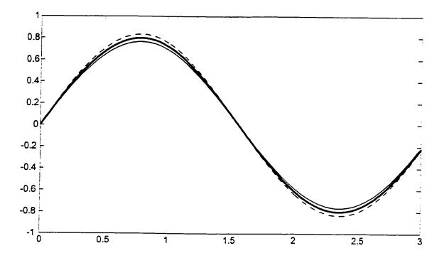
Figure 2.9: The case m=2.T=1.  $\ell=0.01$ . The thick solid line represents the exact initial profile, the thin solid line represents the response of the damped model to the classical heat data and the dashed line represents the response of the classical heat model to the damped data.
