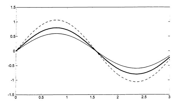
Figure 2.8: The case  $m=2, T=1, \ \delta=0.05$ . The thick solid line represents the exact initial profile, the thin solid line represents the response of the damped model to the classical heat data and the dashed line represents the response of the classical heat model to the damped data.
