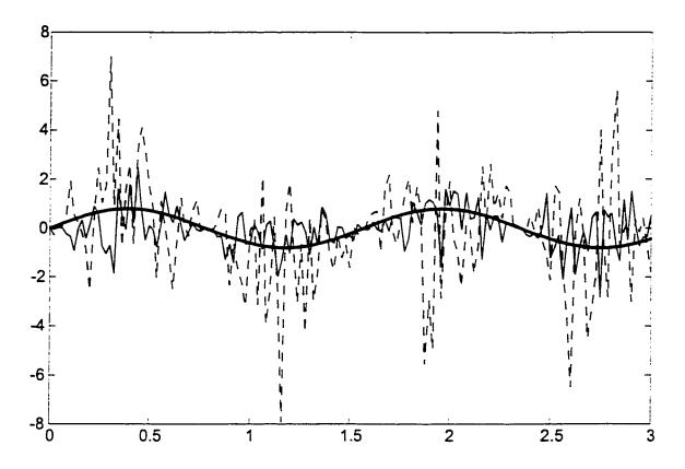
Figure 2.13: The case of noisy data with SNR=100 dB. N=4.T=1.~m=4.  $\delta=0.022$ . The noisy data used in the heat conduction solution is represented by the dotted line and in the damped wave solution by the thin solid line and the exact initial profile by the thick solid line.
