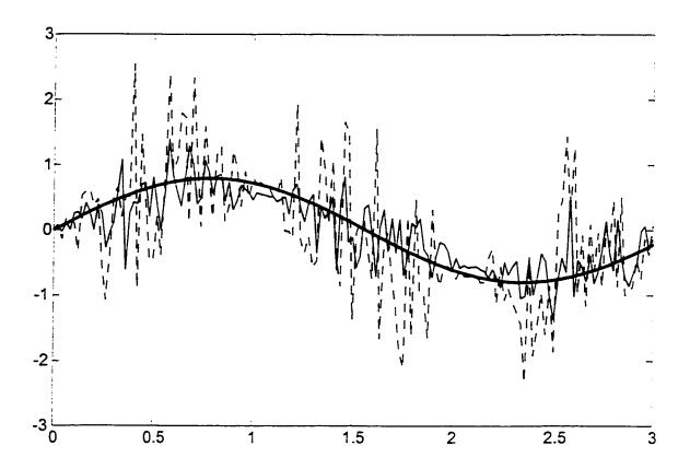
Figure 2.10: The case of noisy data with SNR=50 dB, N=3, m=2, T=1,  $\delta=0.04$ . The noisy data used in the heat conduction solution is represented by the dotted line and in the damped wave solution by the thin solid line and the exact initial profile by the thick solid line.
