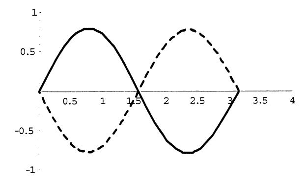
Figure 2.2: Response of the undamped model to the damped data in the case, m=2 and  $\delta=4$  with  $4m^2=\delta^2$ . The thick solid line represents the exact initial profile while the dashed line represents the recovered profile.
