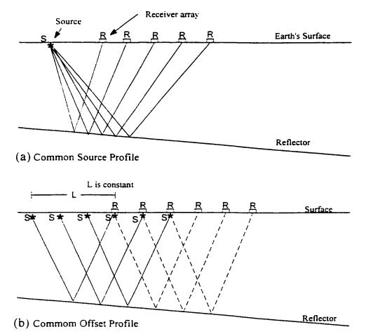
Figure C.1: Geometry of the source receiver array.
