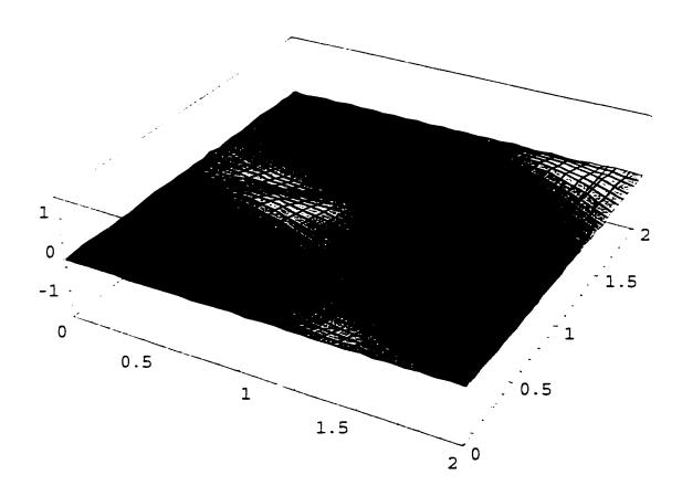
Figure 2.5: Response of the undamped model to the damped data in the case,  $4\lambda_{n,m}^2 > \delta^2$ , with  $\delta = 3$ .
