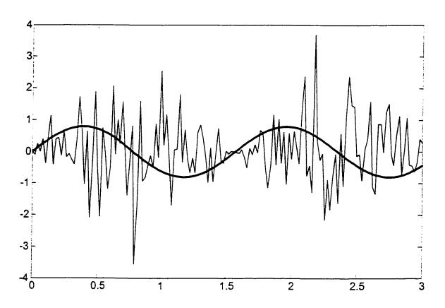
Figure 2.20: Response of the damped model in the case of noisy data with SNR=20 dB. N=4. m=4. T=2,  $\delta=0.11$ .
