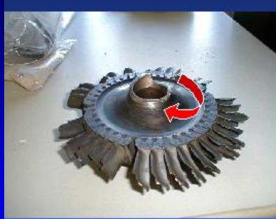
UH-1N Turbine: Helical shaft failure
