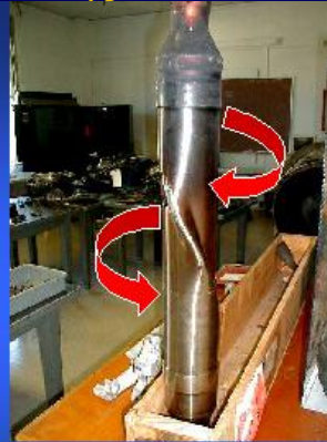
F-18 Engine Shaft Torsional Buckling
