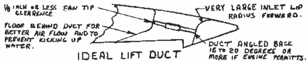
FIGURE 4 Entry and Exit losses (Courtesy of Universal Hovercraft)
