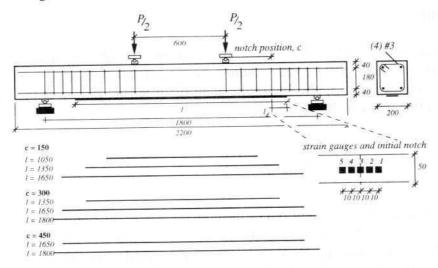
Figure 9. Delamination specimen with initial shear notches
