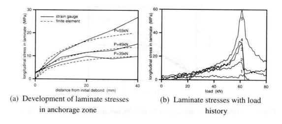
Figure 6. Results from the strain gauges on the beam with 1.4m bonded length
