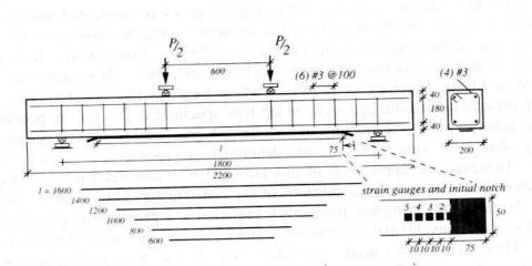
Figure 4. Specialized delamination test specimen
