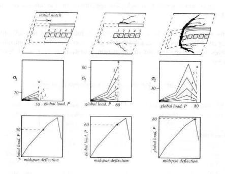
Figure 7. Delamination process zone development with idealizations of Figures 6(b) and 5 for the 1.4 m laminate length beam
