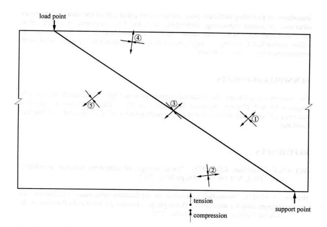
Figure 1 Direction of principle strain on the bonded external steel plate of a strengthened reinforced concrete beam.
