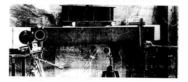
Figure 2 Loading arrangement and failure mechanism for plated rectangular beam.
