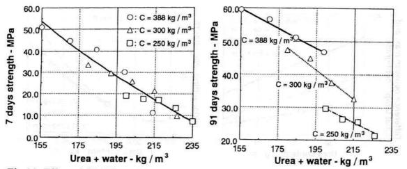
Fig.11. Effect of (U+W) on 7days strength Fig.12. Effect of (U+W) on 91days strength
