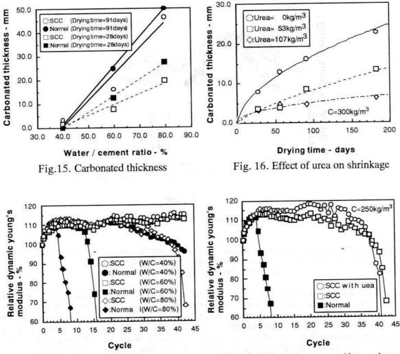
Fig.17. Resistance to sulfate attack
