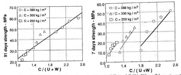
Fig.9. Effect of C/(U+W) on 91days strength Fig.10. Effect of C/(U+W) on 7days strength
