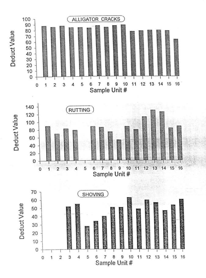
Fig. 5 : Distribution of deduct values of alligator cracks, rutting and showing over the sample units of a test site.
