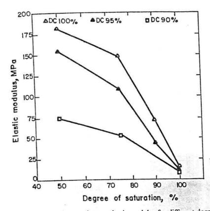
Fig. 7. Effect of degree of saturation on elastic modulus for different degrees of compaction and confining pressures.
