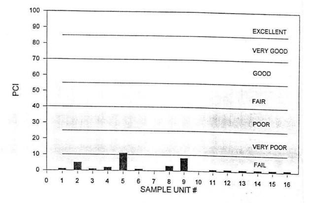
Fig. 6 : Distribution of the pavement condition Index PCI over the sample units of a test site.
