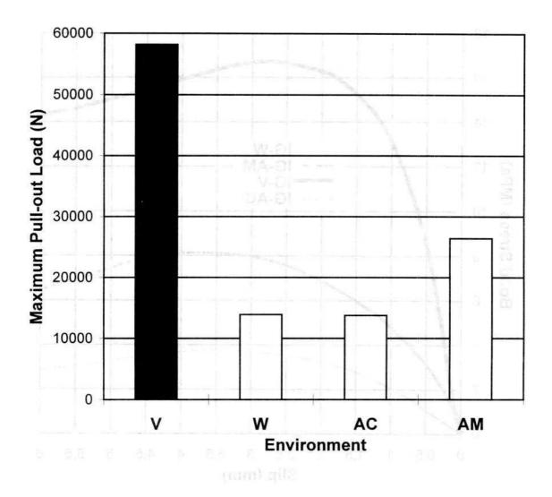
Fig.5. Maximum pull-out load for IG rods after exposure to different environments
