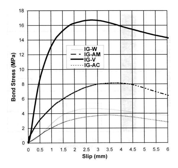
Fig.4. Bond stress vs. free-end slip for IG-V, IG-AM, IG-AC, and IG-W specimens
