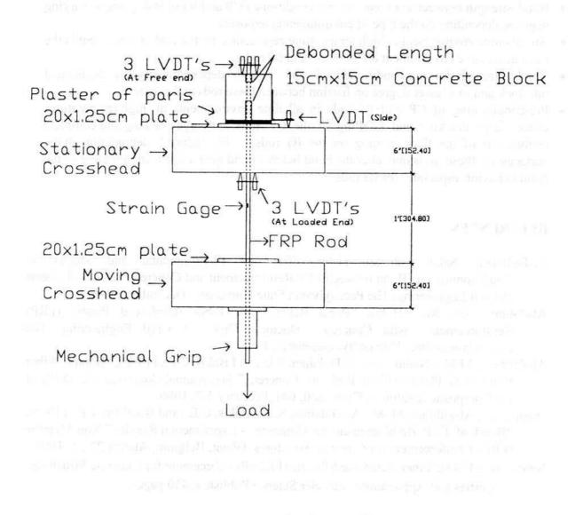
Fig. 1. Schematic diagram for direct pull out test setup
