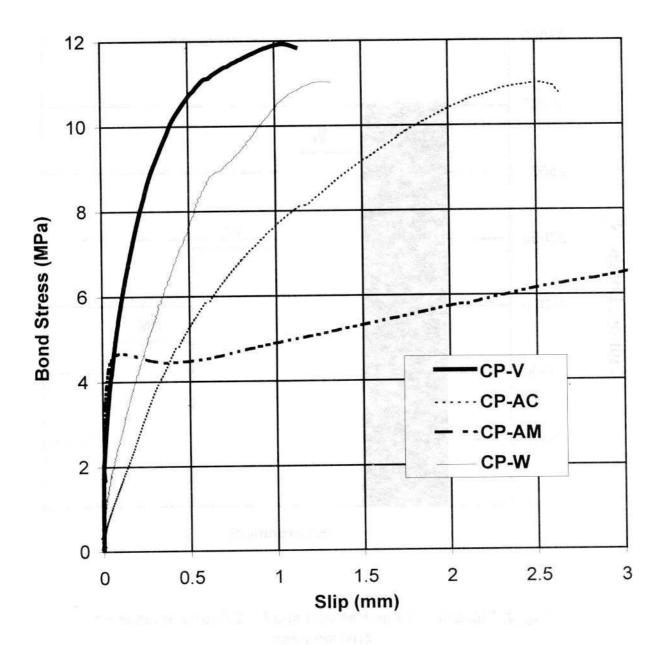
Fig. 2. Bond stress vs. free-end slip for CP-V, CP-AM, CP-AC, and CP-W specimens
